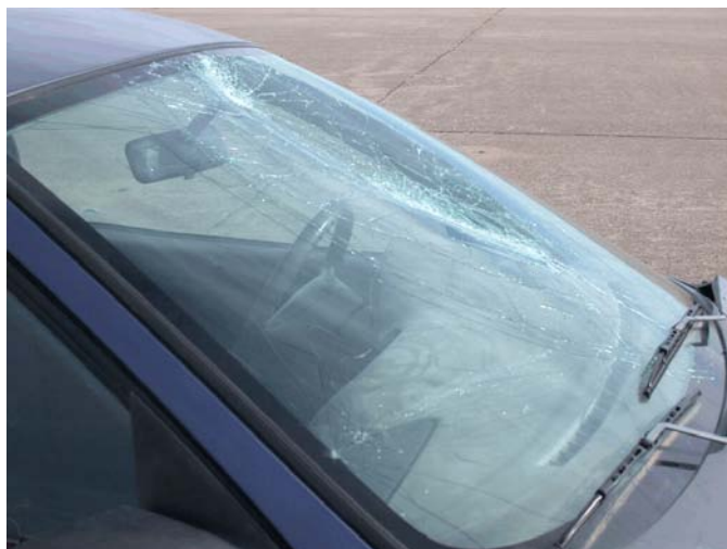
Figure 13. Windshield Damage, Test M-3
