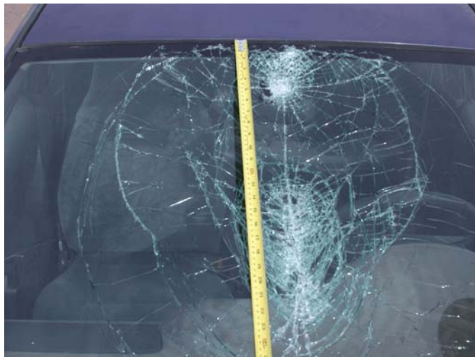
Figure 14. Windshield Damage, Test M-3
