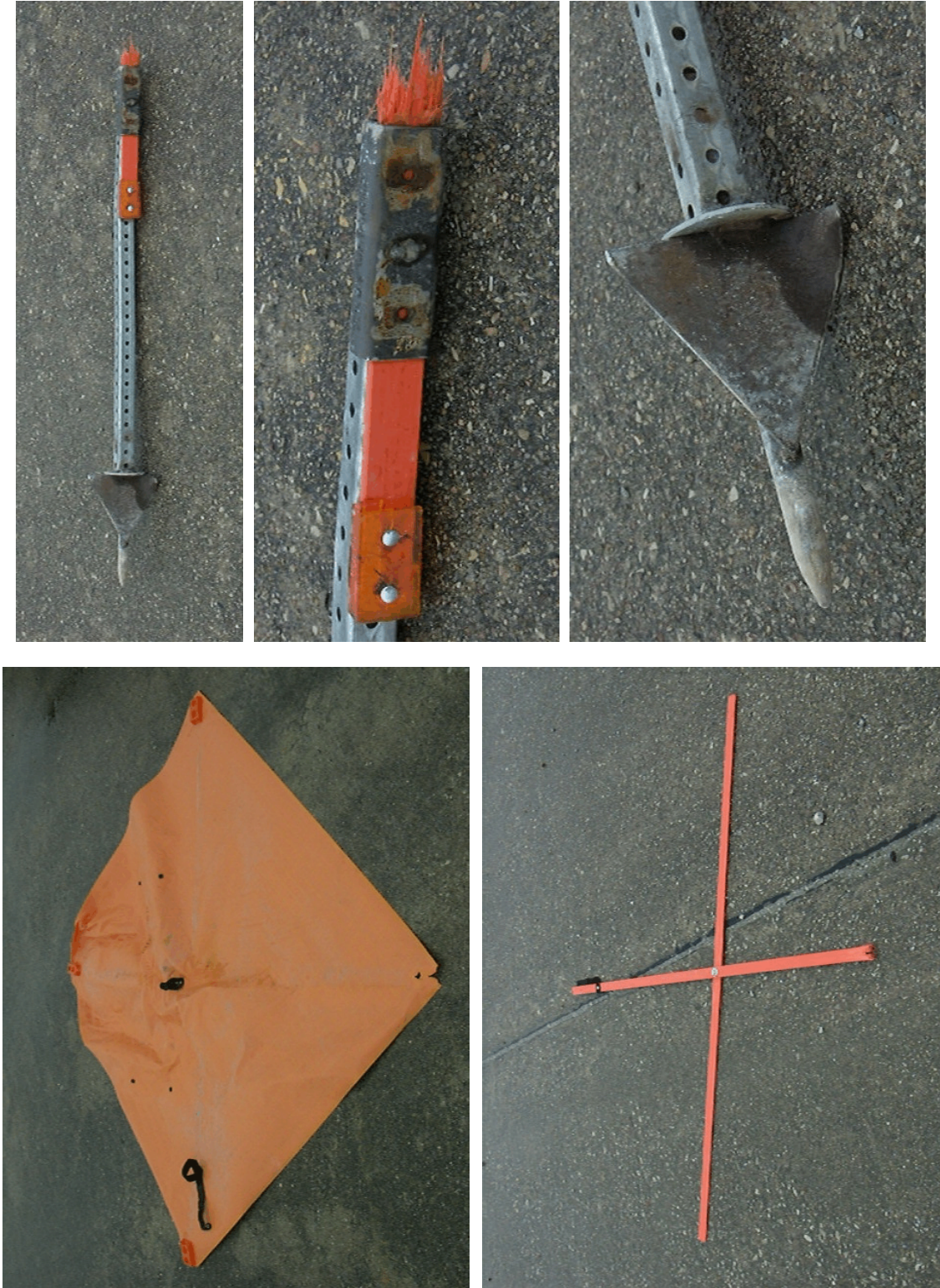
Figure 33. System Damage, Bogie Test MOSBOG-12 (0 degrees)
