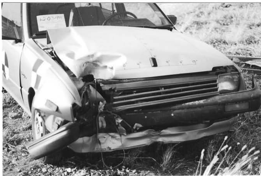
Figure 29. Vehicle Damage, SDG-2
