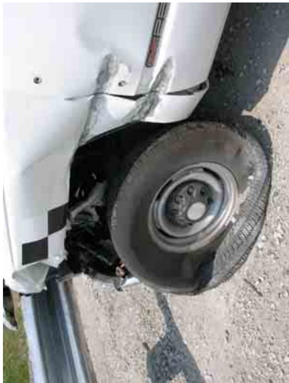
Figure 114. Vehicle Damage, Test MGSDF-1
