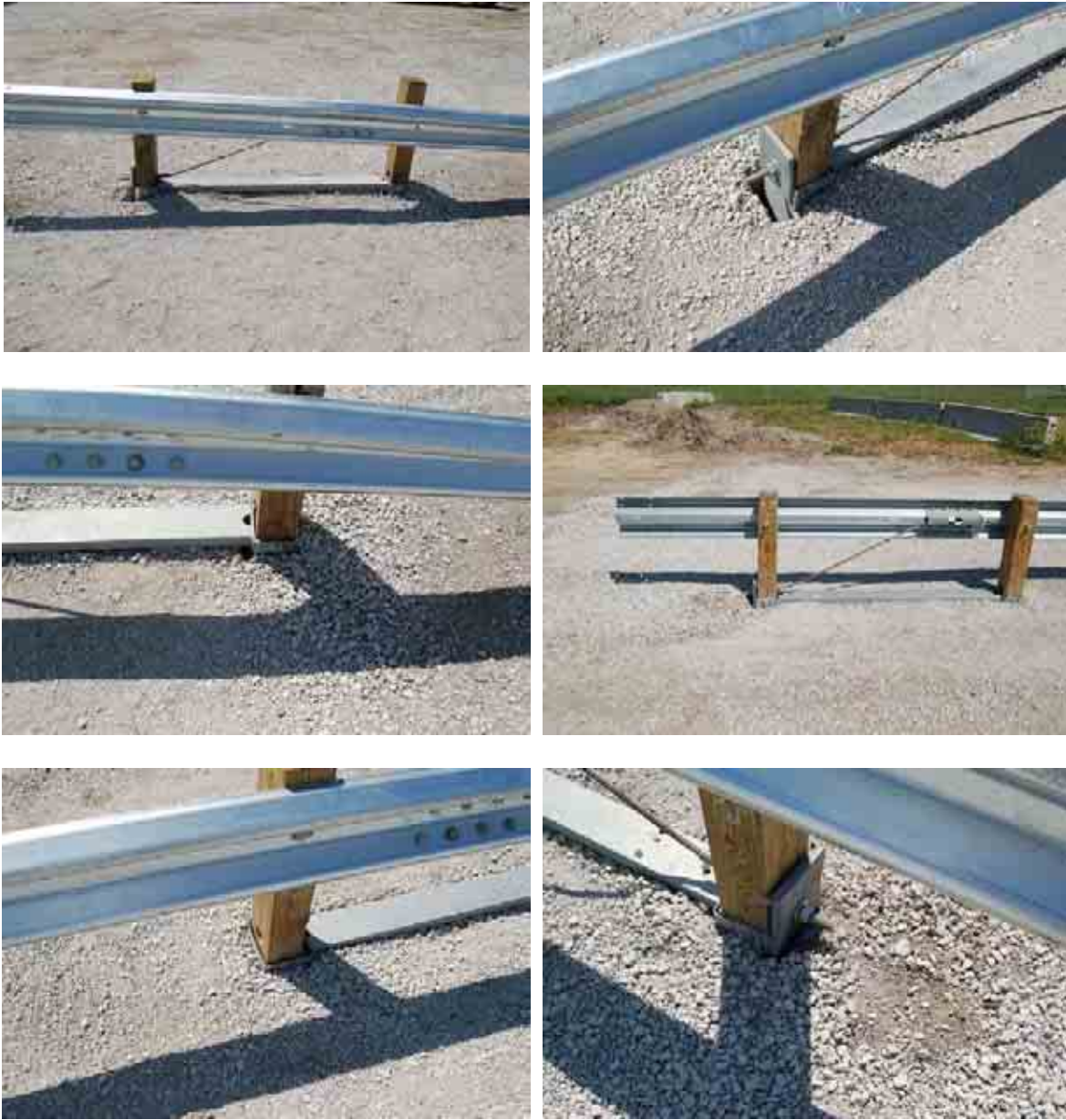
Figure 128. System Damage, Test MGSPP-1
