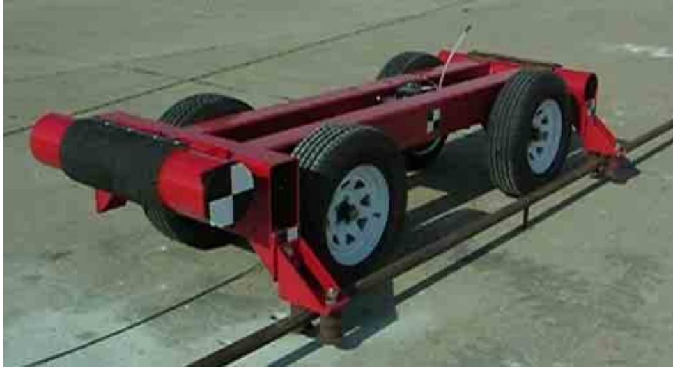
Figure 6. Rigid Frame Bogie on Guidance Track
