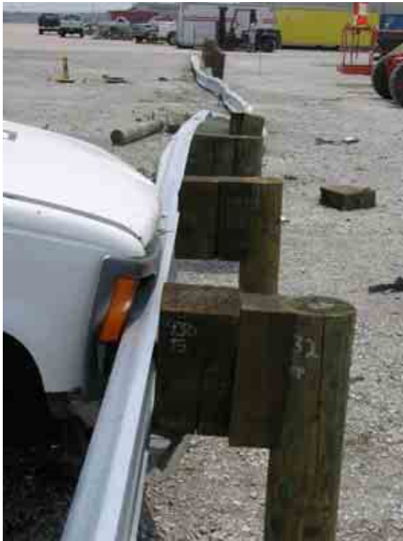
Figure 107. Vehicle Final Position and Trajectory, Test MGSDF-1
