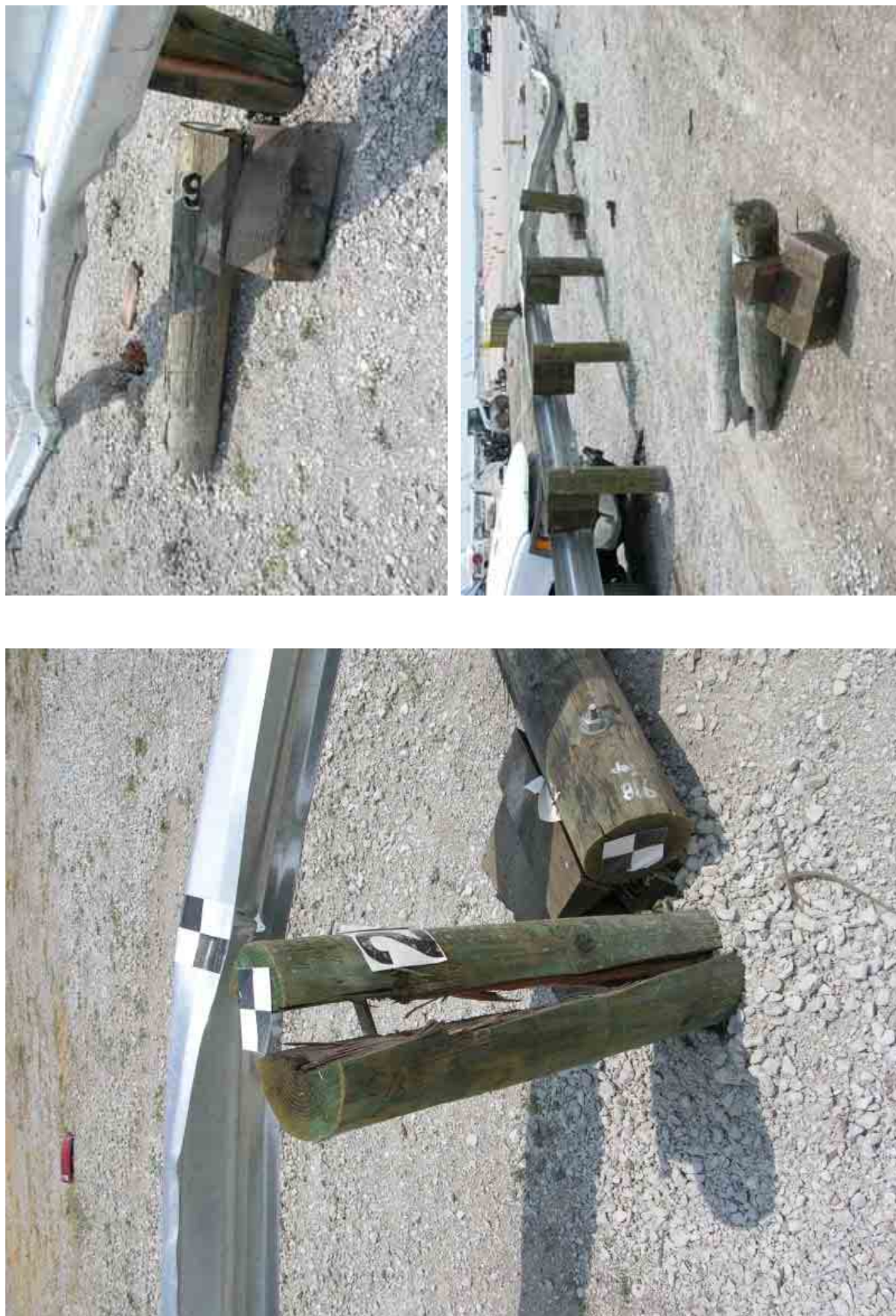
Figure 111. System Damage, Test MGSDf-1
