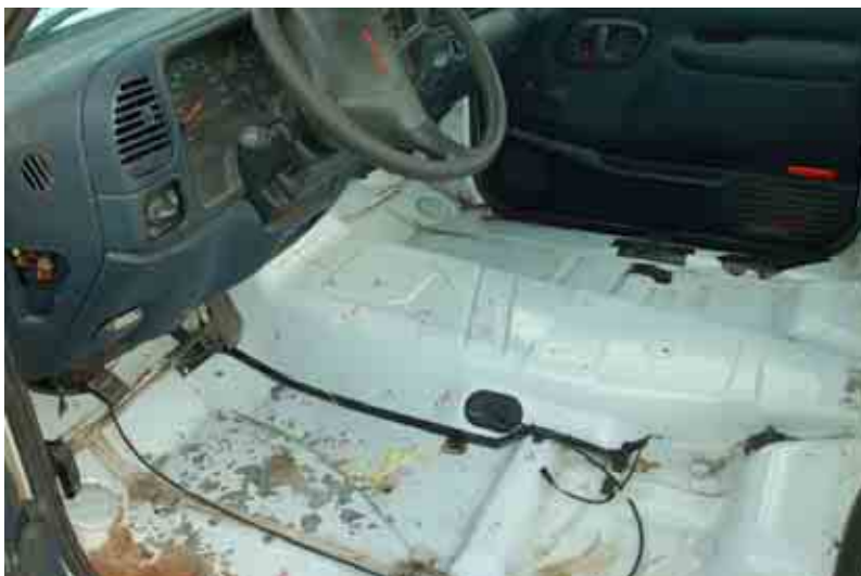
Figure 115. Occupant Compartment Damage, Test MGSDF-1
