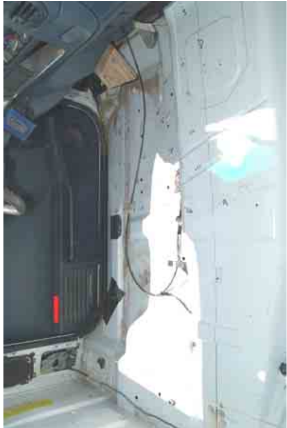
Figure 131. Occupant Compartment Damage, Test MGSPP-1
