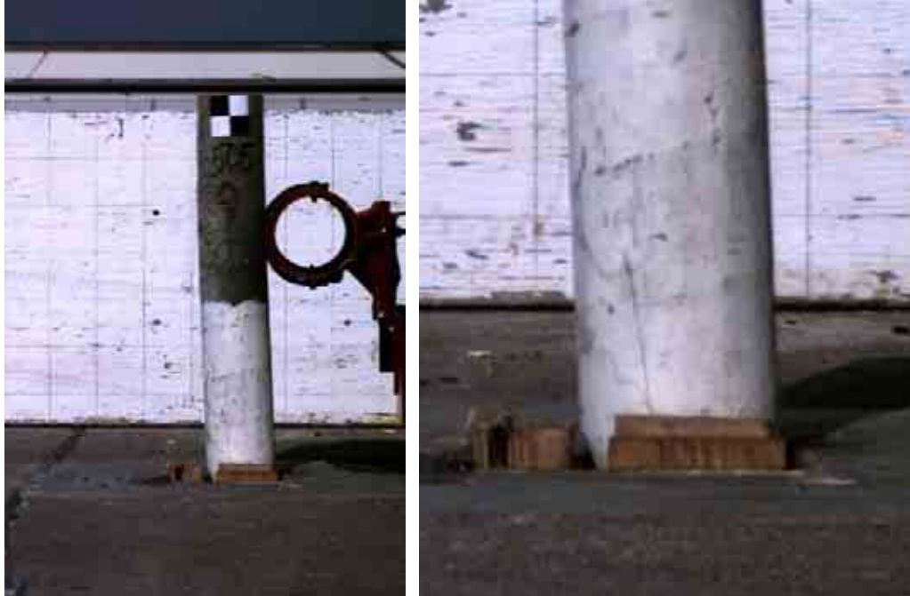
Figure 12. Post Bending Prior to Fracture - Frame 107
