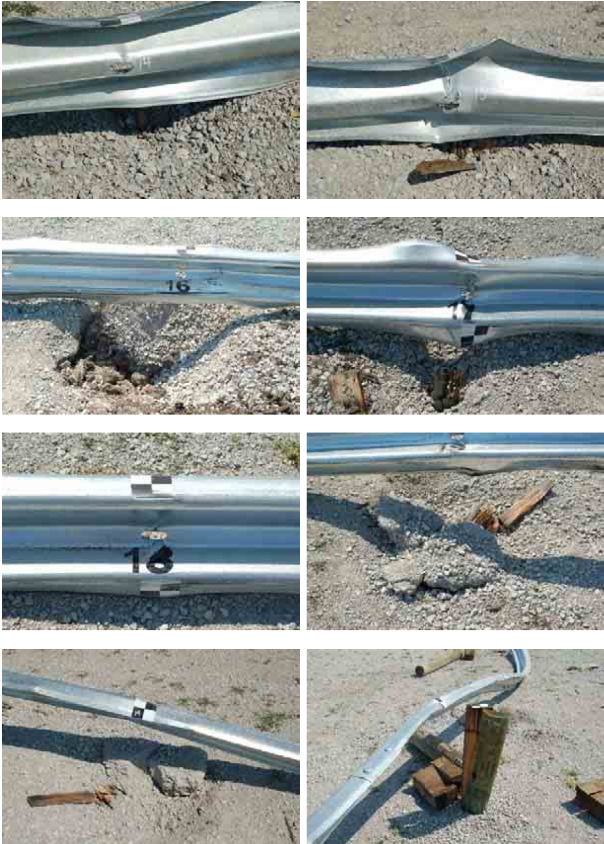
Figure 112. System Damage, Test MGSDF-1
