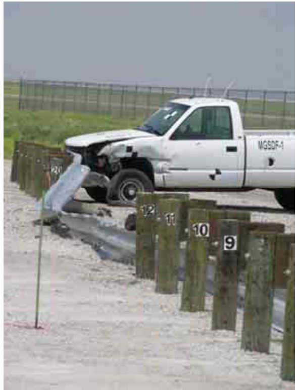
Figure 107. Vehicle Final Position and Trajectory, Test MGSDF-1
