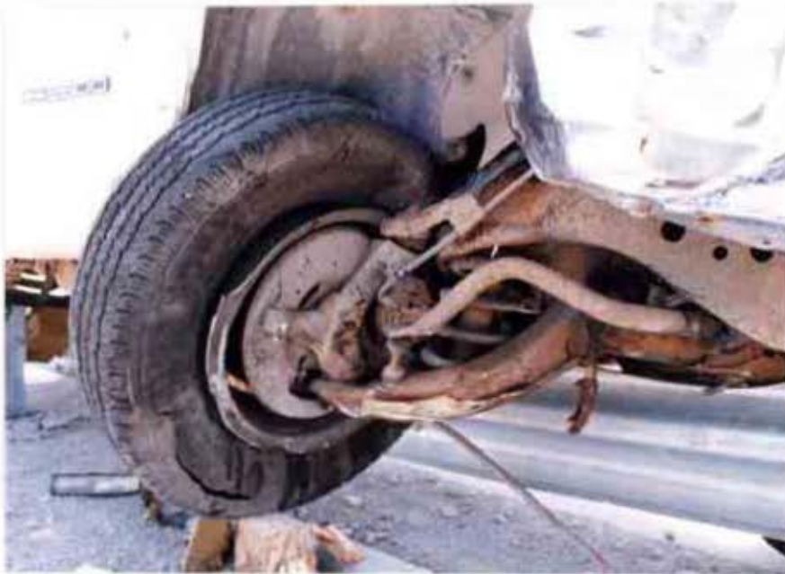
Figure 27. Front-End Vehicle and Rear-Tire Damage, Test MIW-2
