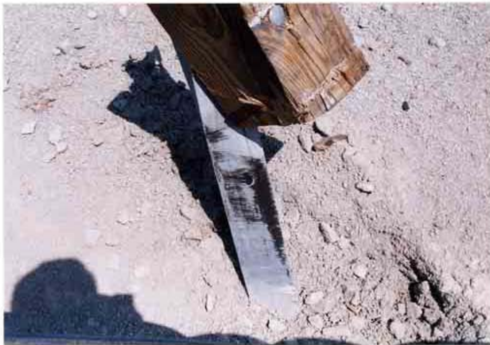
Figure 20. Type B Longitudinal Barrier Rail and Post Damage, Test MIW-2
