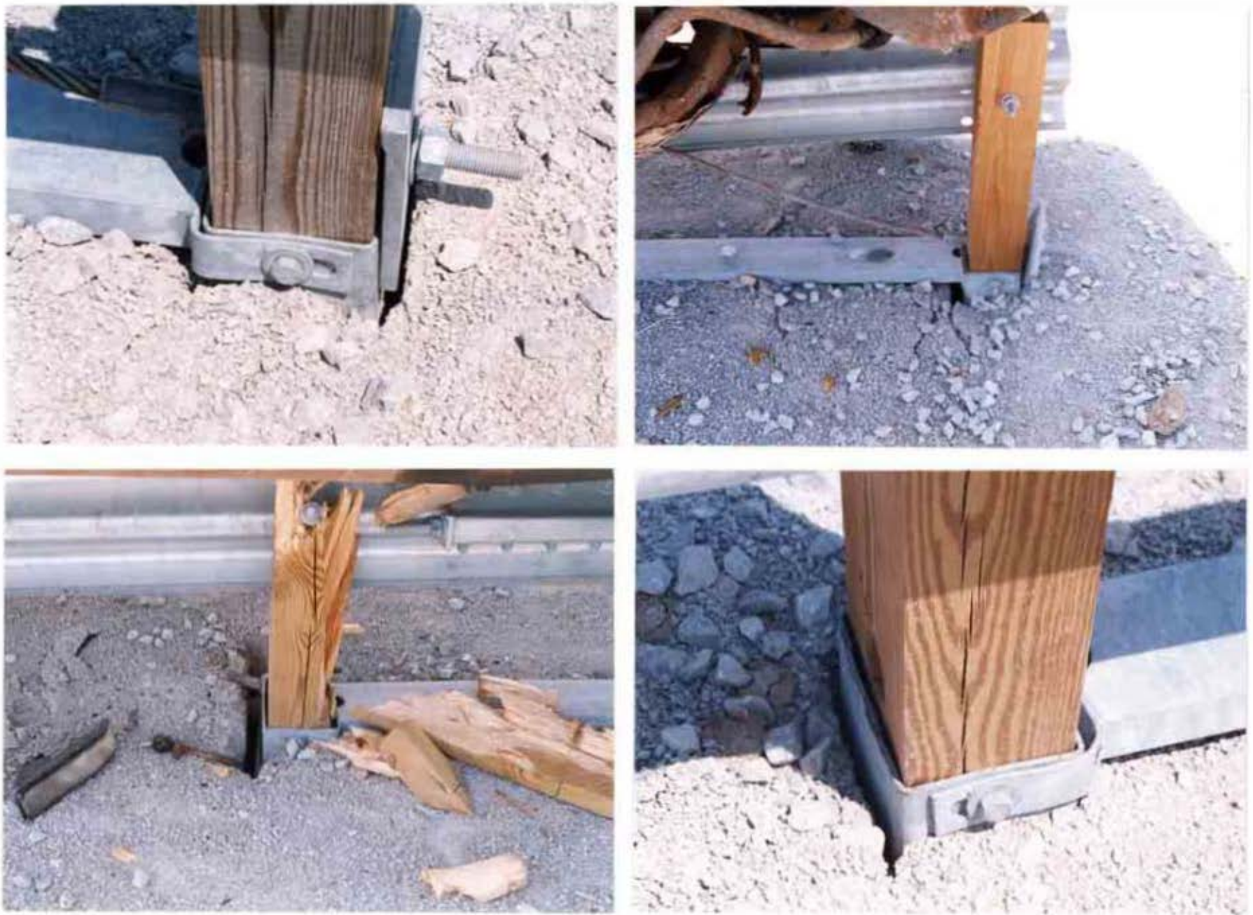
Figure 25. Permanent Set Deflections of End Anchorages, Test MIW-2
