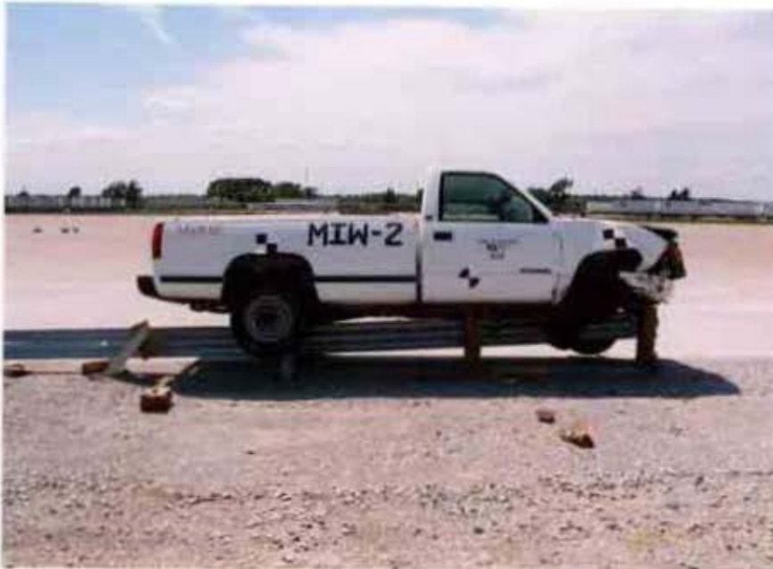
Figure 26. Vehicle Damage, Test MIW-2
