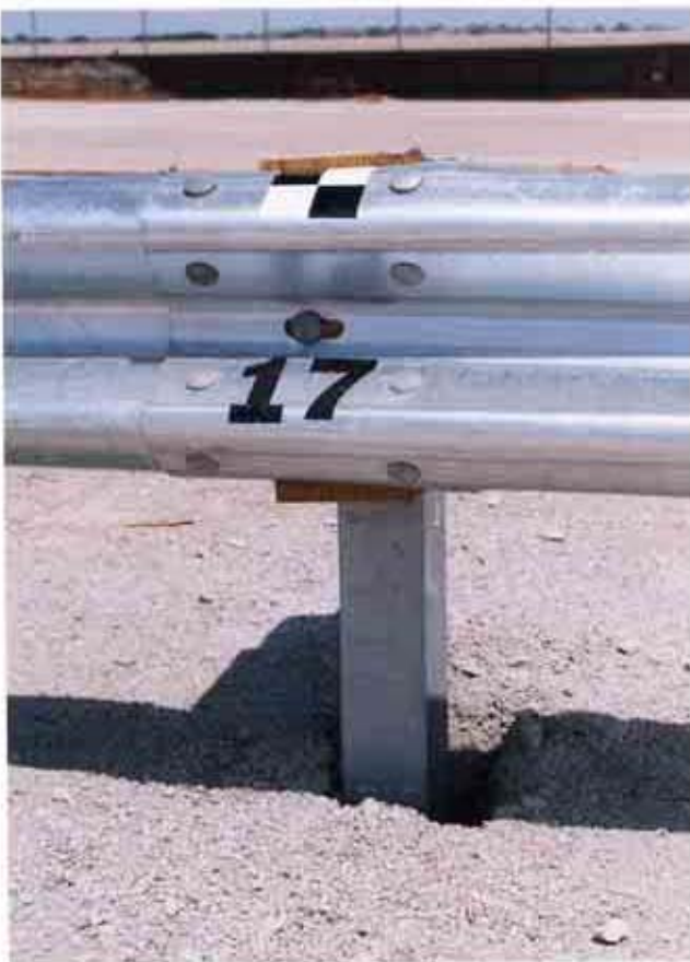
Figure 21. Type B Longitudinal Barrier Rail and Post Damage, Test MIW-2
