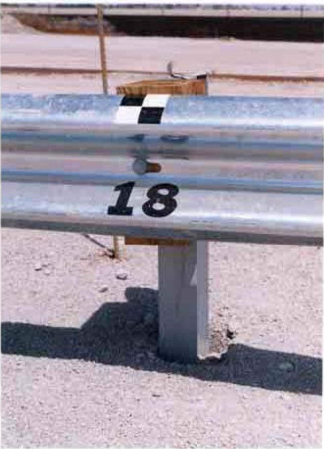
Figure 21. Type B Longitudinal Barrier Rail and Post Damage, Test MIW-2
