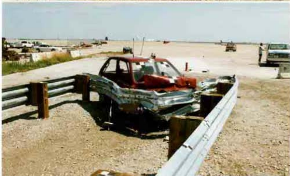
Figure 41. Barrier Damage, Test MBN-2
