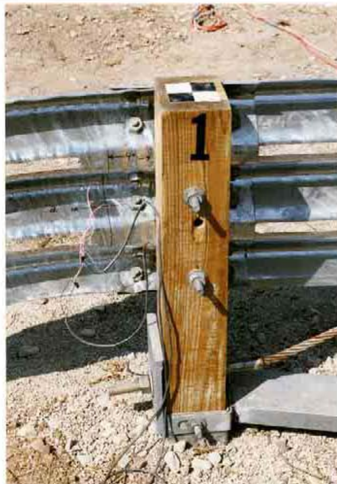
Figure 20. Strain Gauge Locations, Test MBN-1
