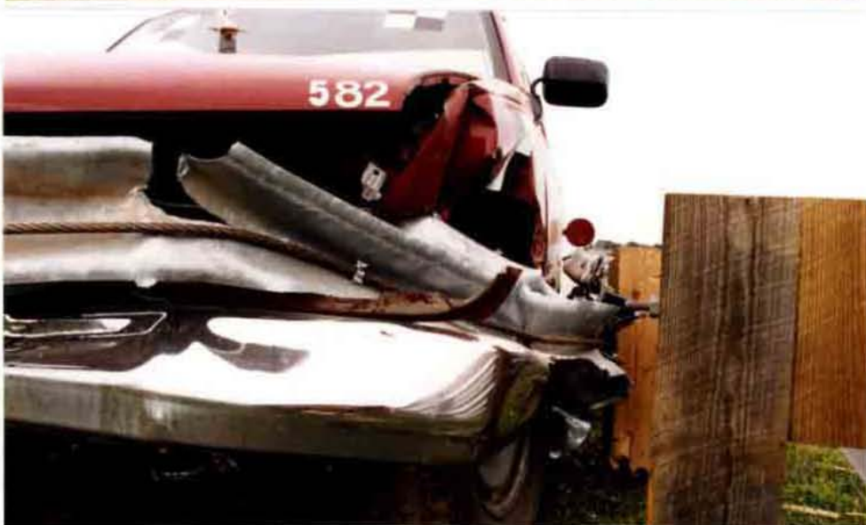
Figure 47. Barrier Damage, Test MBN-4
