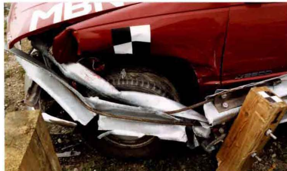
Figure 45. Vehicle Damage, Test MBN-4
