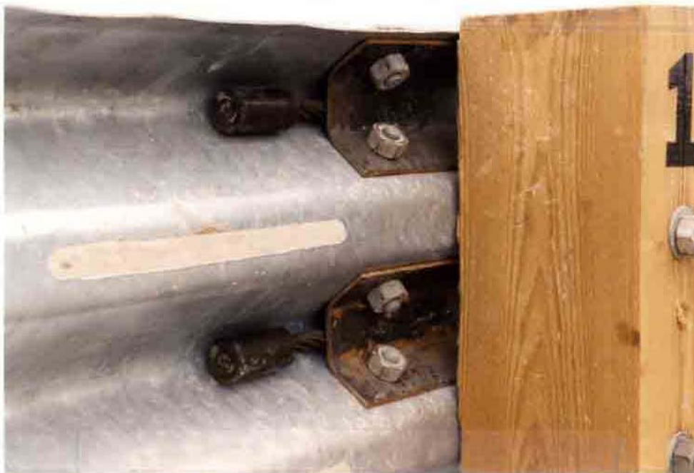
Figure 36. Bullnose Design, Test MBN-4
