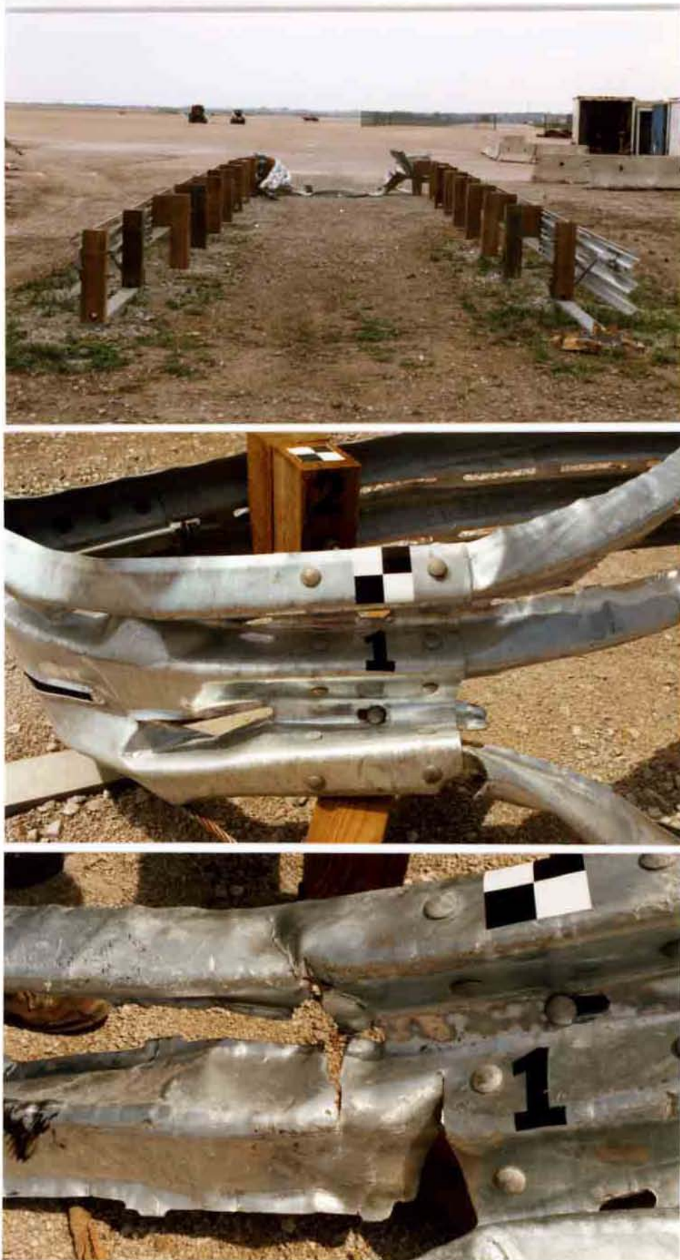
Figure 27. Barrier Damage, Test MBN-3
