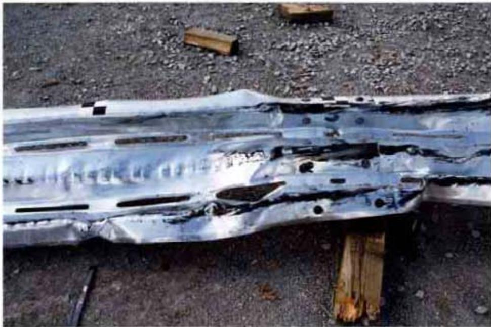
Figure 47. Barrier Damage, Test MBN-6
