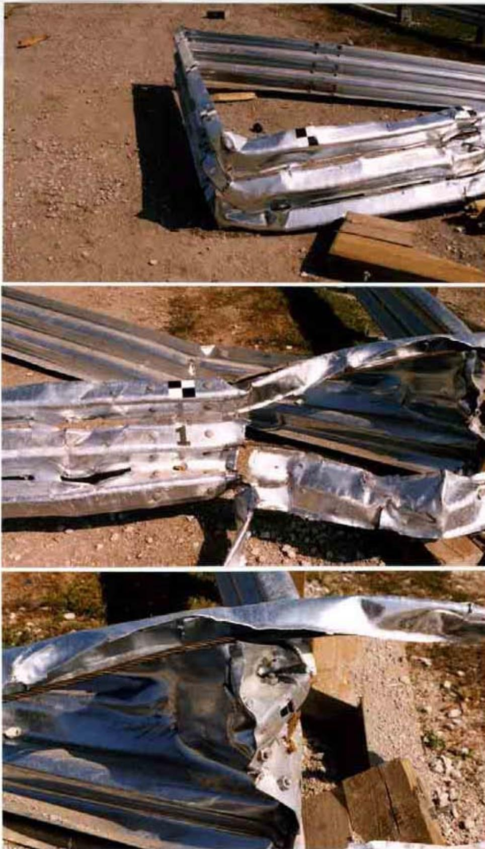
Figure 35. Barrier Damage, Test MBN-5
