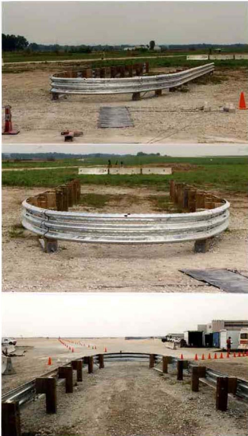
Figure 9. Bullnose Barrier Design, Test MBN-5
