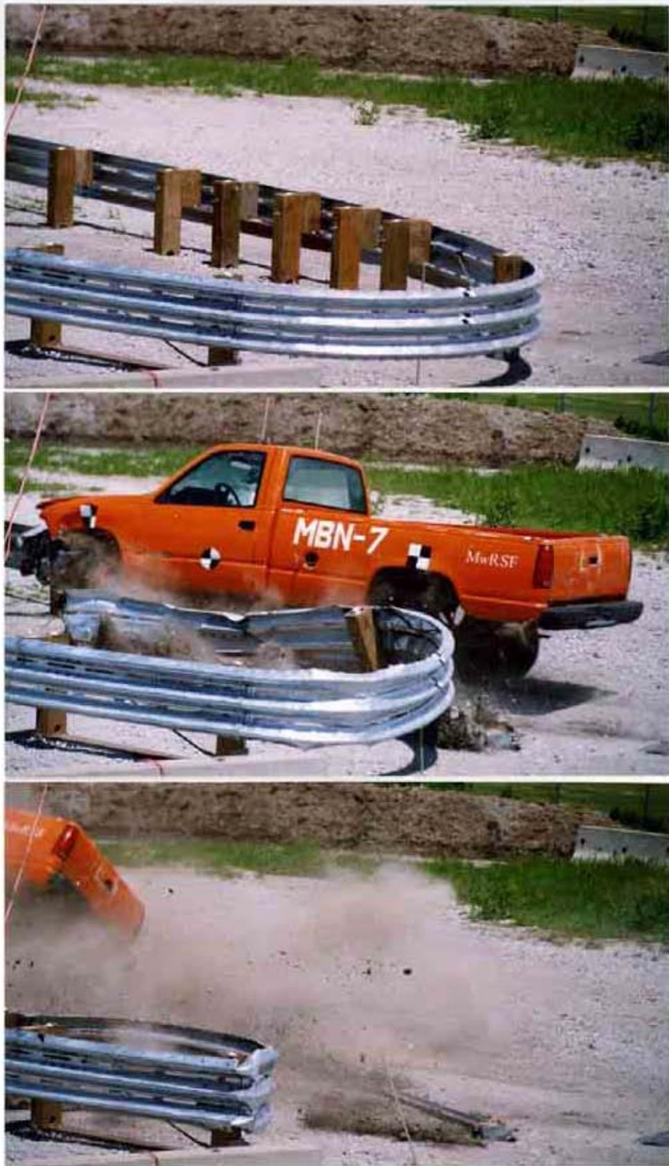
Figure 54. Full-Scale Crash Test, Test MBN-7
