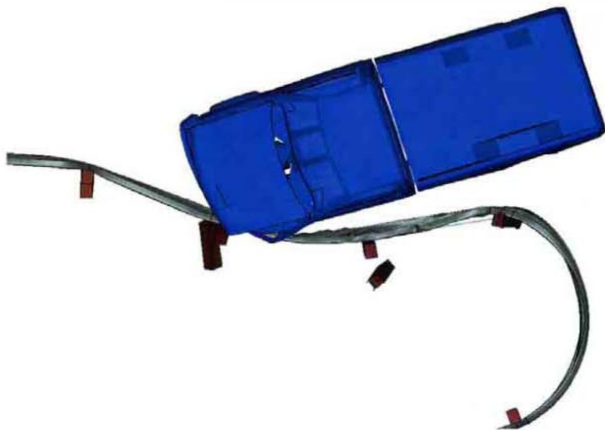
Figure 63. No Strut Simulation - Rail Does Not Roll Over
