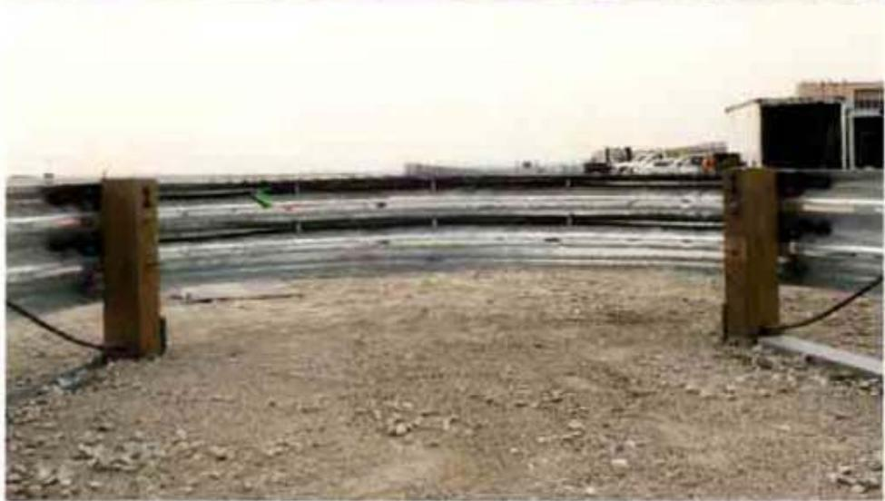
Figure 10. Bullnose Barrier Design, Test MBN-5
