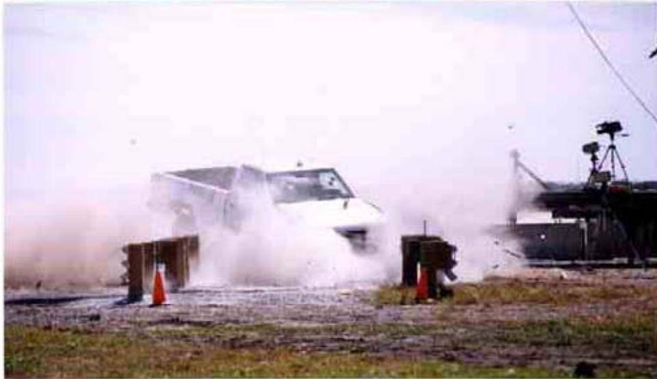
Figure 75. Full-Scale Crash Test MBN-8
