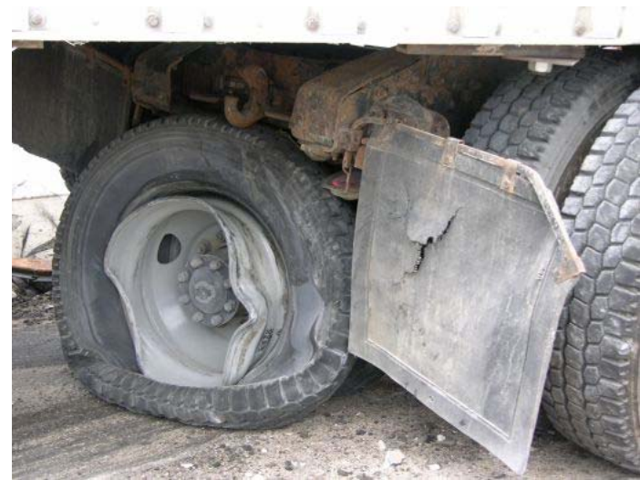
Figure 90. Vehicle Damage to Front Tandems, Test TL5CMB-2
