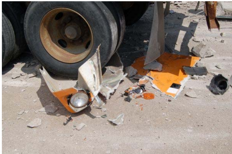
Figure 92. Damage to Rear of Vehicle, Test TL5CMB-2
