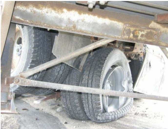
Figure 90. Vehicle Damage to Front Tandems, Test TL5CMB-2
