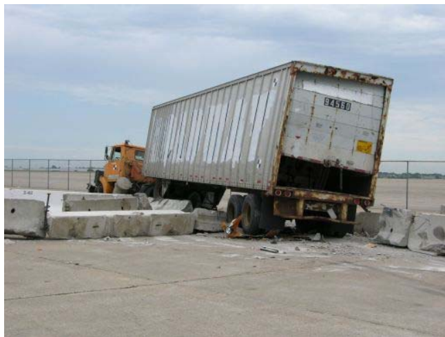
Figure 85. Vehicle Damage, Test, TL5CMB-2
