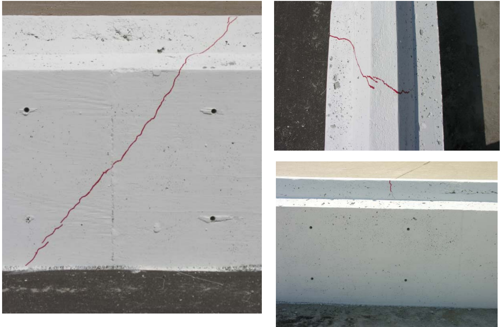
Figure 75. Barrier Cracks 4.6 m (15 ft) from Upstream End, Test TL5CMB-2
