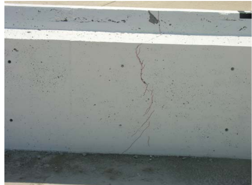
Figure 76. Barrier Cracks 5.8 m (19 ft) from Upstream End, Test TL5CMB-2
