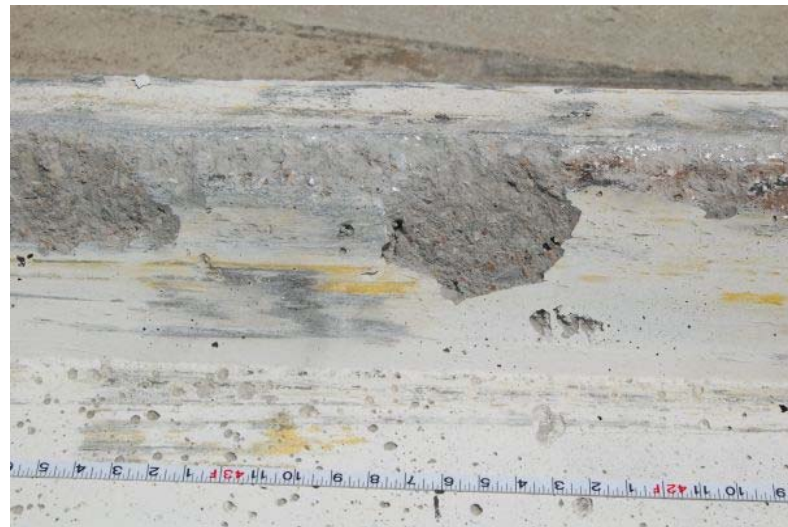
Figure 82. Barrier Damage to Top Protrusion 12.2 – 14.3 m (40 – 47 ft) from Upstream End, Test TL5CMB-2
