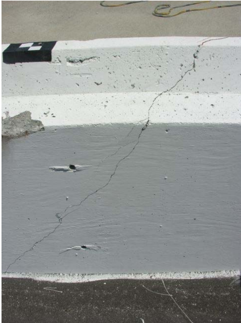
Figure 76. Barrier Cracks 5.8 m (19 ft) from Upstream End, Test TL5CMB-2
