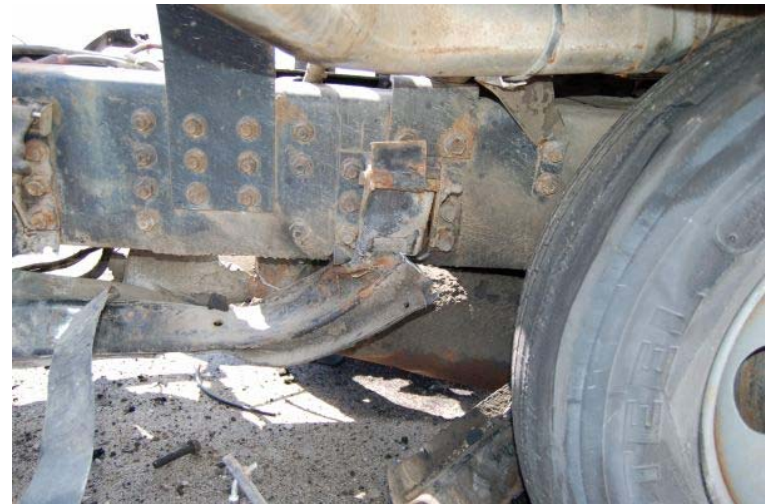
Figure 88. Right Side Tractor Damage, Test TL5CMB-2
