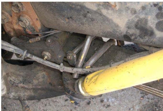
Figure 87. Front Right Tractor Damage, Test TL5CMB-2
