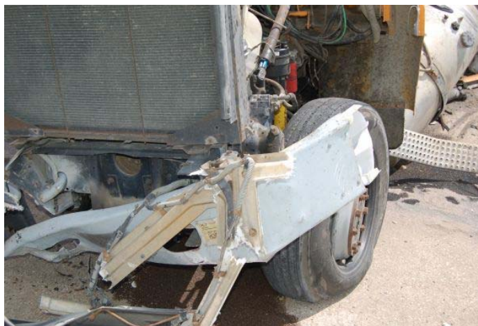
Figure 86. Front Bumper Damage, Test TL5CMB-2
