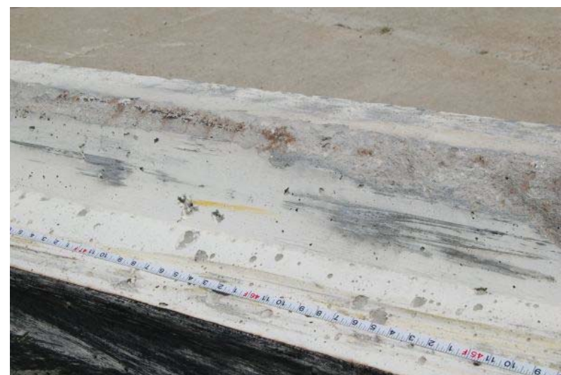
Figure 82. Barrier Damage to Top Protrusion 12.2 – 14.3 m (40 – 47 ft) from Upstream End, Test TL5CMB-2
