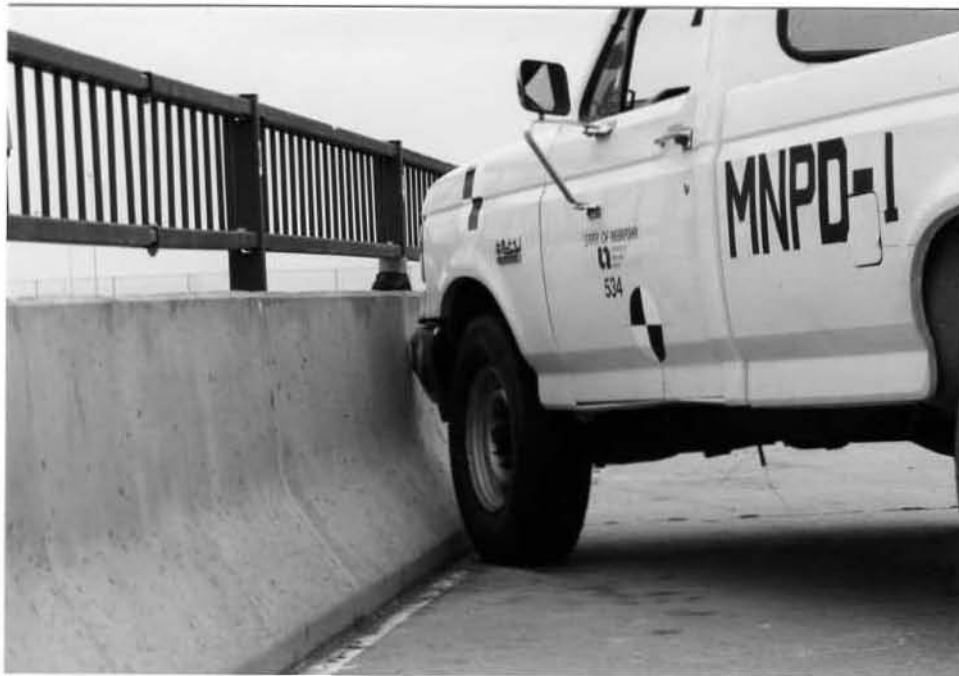
Figure 23. Impact Location, Test MNPD-1
