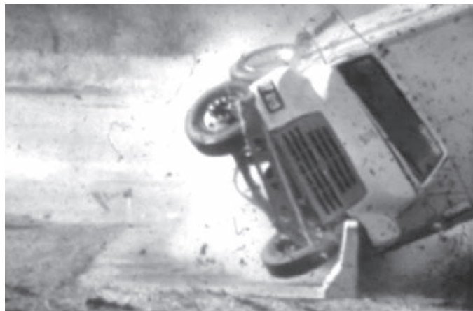
Figure 23. Example of a single-unit truck rolling over onto a 32-in.-tall concrete safety shaped barrier [Sheikh 2011].
