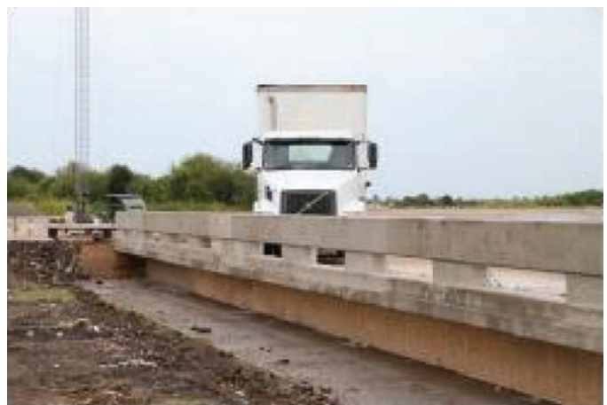
Figure 31. MASH Test 5-12 setup for the Texas T224 bridge rail [Williams 2017].
