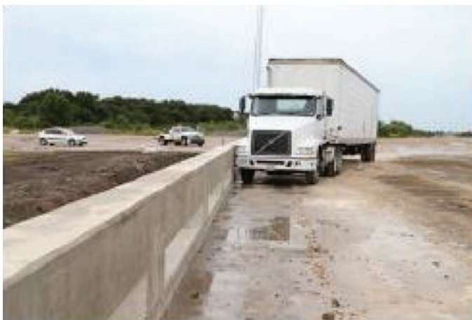
Figure 31. MASH Test 5-12 setup for the Texas T224 bridge rail [Williams 2017].
