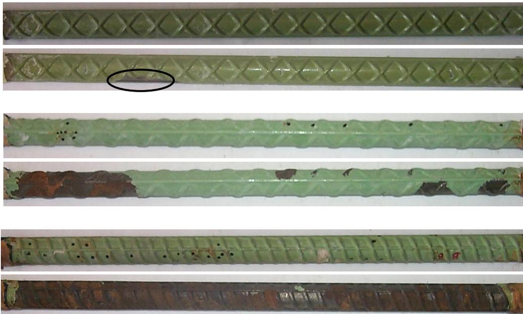
Figure 1: Three ECR bars after exposure in Cl<sup>-</sup> contaminated concrete, first, with coating holidays identified (upper photograph of each bar pair) and , second, showing bar appearance upon removal of disbonded coating (lower photograph of each bar pair).
