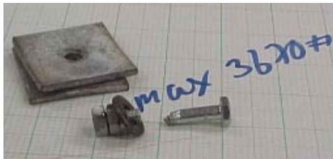
(C) Typical failure of improved connection detail
