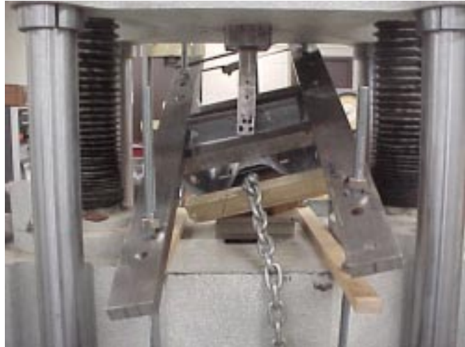
(A) Quasi-static test setup for rail-post connection.
