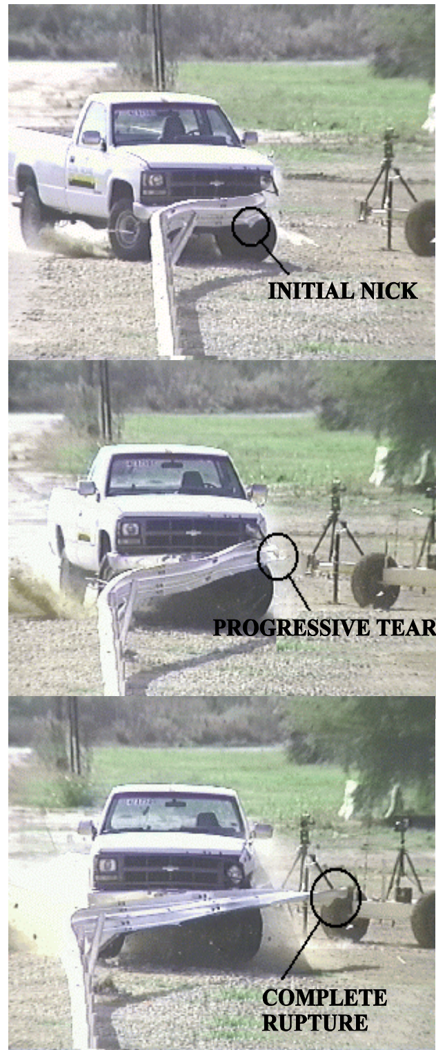
Figure 3. Test of a weak-post w-beam guardrail with splice at the mid-span and an improved connection showing the rupture of the guardrail.(3)
