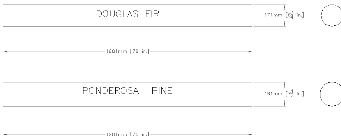
Figure 44. Major Dimensions of Round Wood Posts - Round Two Testing
