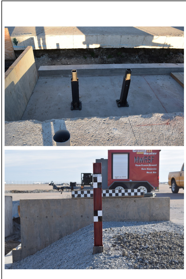
Figure 11. Test installation photographs for steel tube socket assemblies.
