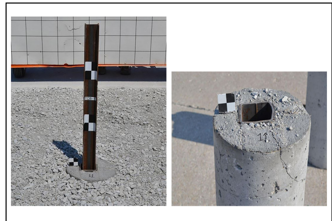
Figure 6. Cylindrical concrete foundations for S3x5.7 cable barrier posts (14).
