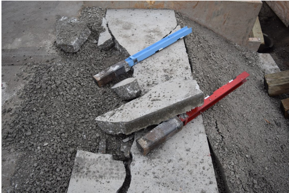
Figure 15. Post-test damage to 4 in.-thick concrete slab.
