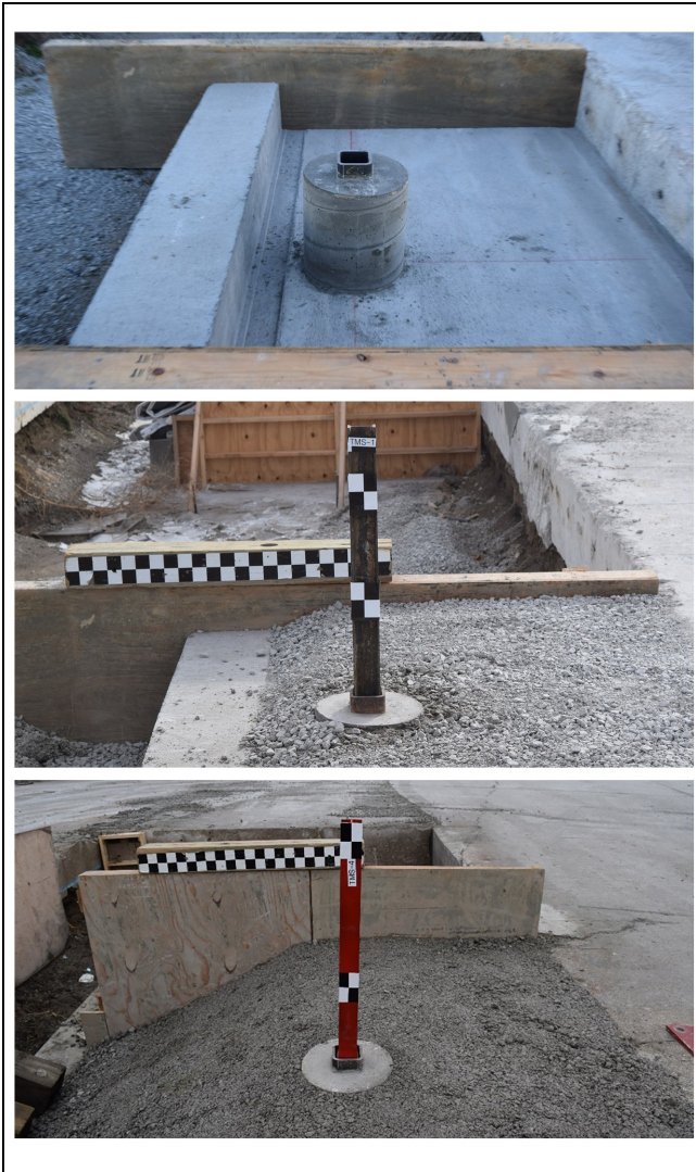
Figure 10. Test installation photographs for cylindrical concrete foundations.
