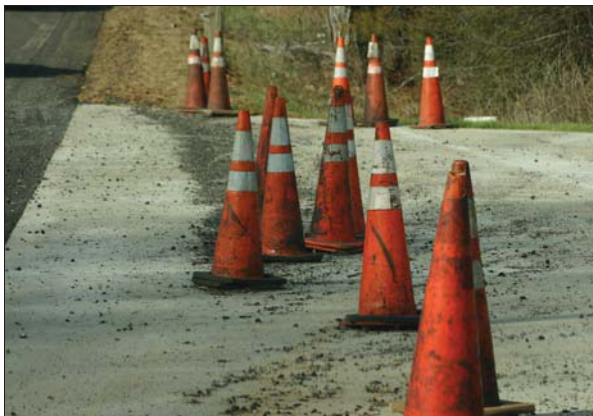
X Dirty and Poor Sheeting
