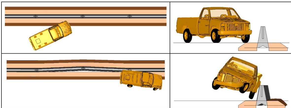
234 **Figure 4: Simulation results with 100-ft installation of single slope barrier embedded 10 inches in soil (initial**
