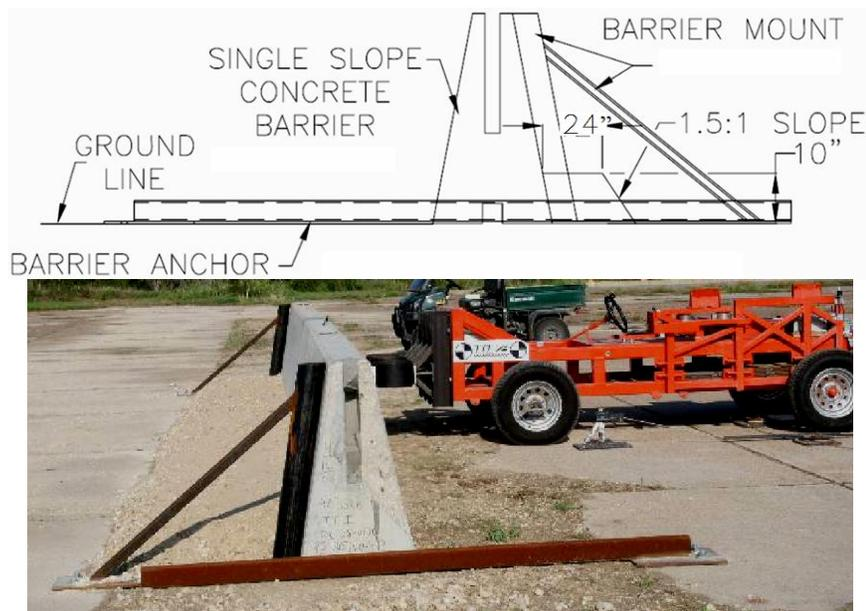
(a) Bogie test setup
