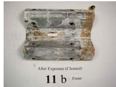
Figure 11 - Part B GSGR Disassembled Joint Cleaned
