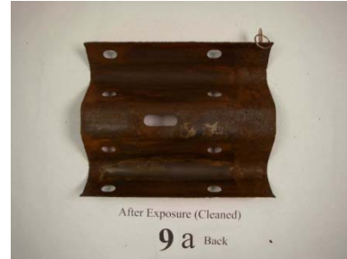
Figure 15 - Part A WSGR Disassembled Joint Cleaned
