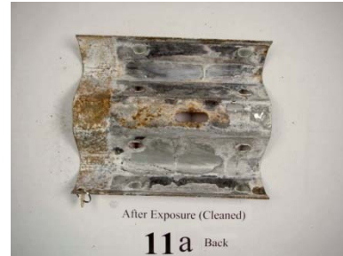
Figure 10 - Part A GSGR Disassembled Joint Cleaned
