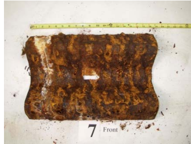
Figure 24 - WSGR with Zinc Foil Insert Assembled Joint after Exposure
