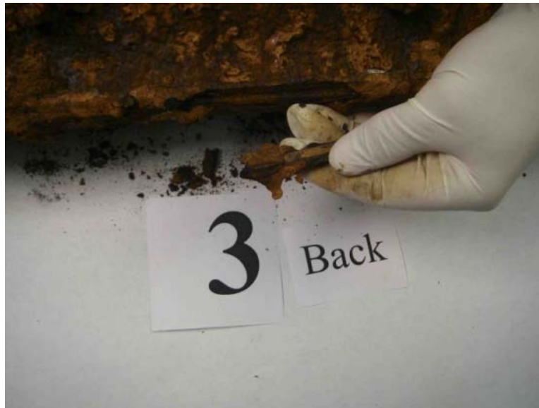
Figure 31 - WSGR with Flakey, Brittle Oxidized Surface
