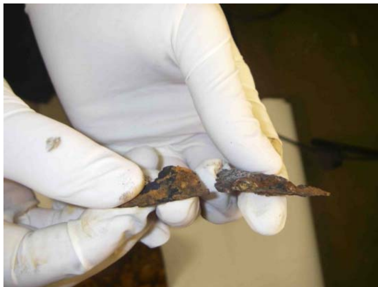
Figure 32 - Close-Up of WSGR Oxidized Debris
