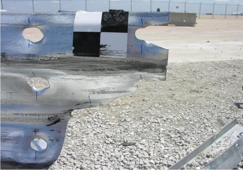
FIGURE 3 Sequential photos and system damage, test no. MWTC-1.
