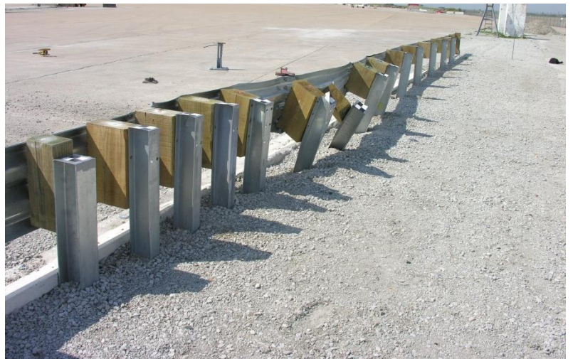
FIGURE 8 Sequential photos and system damage, test no. MWTC-3.
