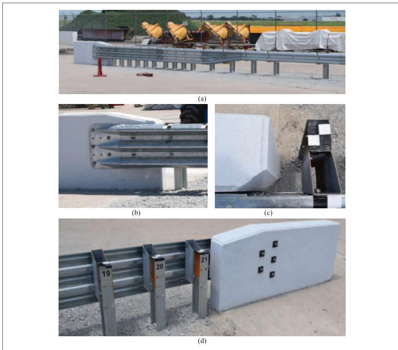
Figure 6. Test installation photographs: (a) layout, (b) buttress connection, (c) buttress overhead, and (d) adjacent posts.
