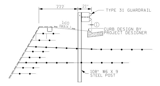
1 USE CAUTION WHEN PLACING CURB WITH GUARDRAIL. CURBS ADVERSELY AFFECT THE PERFORMANCE OF THE GUARDRAIL.
