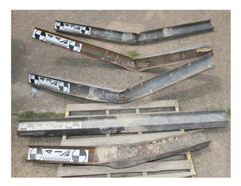
Figure 2.3. Extracted posts after first set of the bogies tests.
