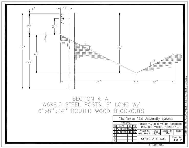
Figure 3.4. Cross section of guardrail on 2H:1V slope.
