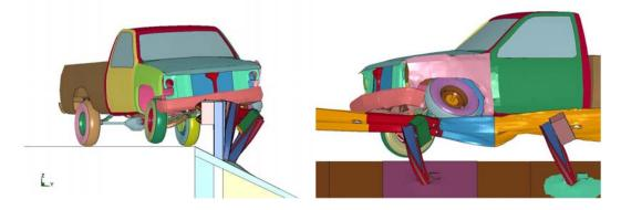
Figure 2.13. Vehicle-barrier interaction associated with test 3-11 impact of a guardrail on 2H:1V slope with 8-ft long posts spaced at 6 ft-3 inch.
