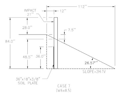
Figure 2.17. Placement of the new post design (Case 7).
