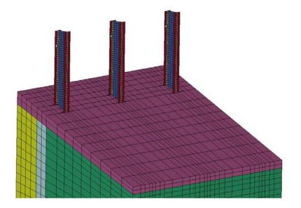
Figure 2.5. Soil model with posts embedded on the sloped face.
