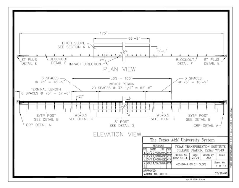
Figure 3.13. Target impact point for test on guardrail on 2H:1V slope.
