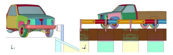
Figure 2.8. Guardrail on slope system with 6 ft-3 inch post spacing.
