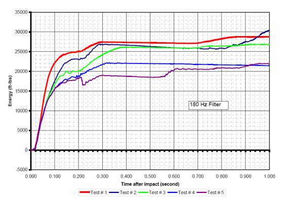
Figure 2.2. Energy plots for bogie tests.
