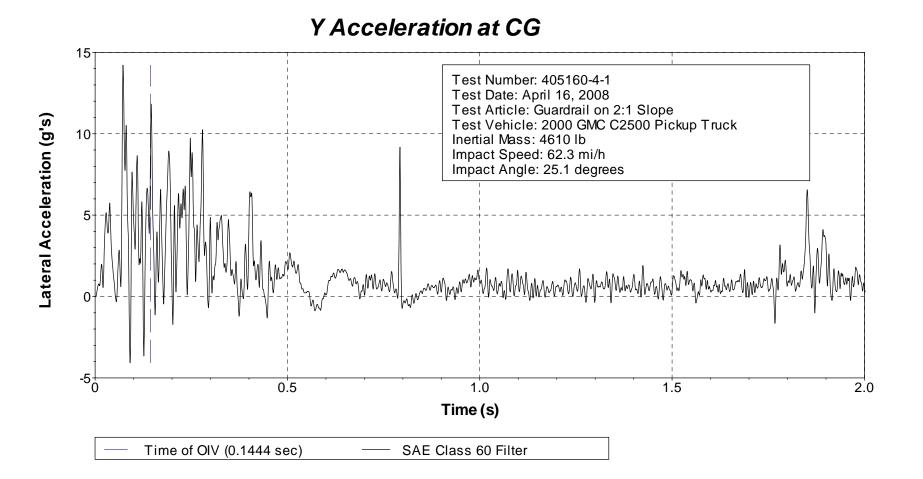
Figure D3. Vehicle lateral accelerometer trace for test 405160-4-1 (accelerometer located at center of gravity).
