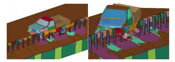
Figure 2.14. Simulation with 3 ft-1.5 inch post spacing.
