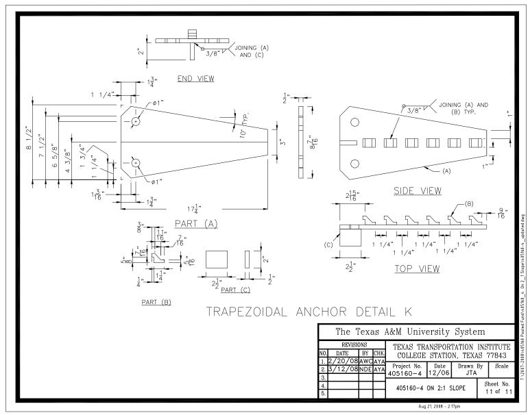
Figure 3.11. Anchor bracket details.
