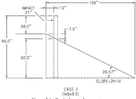
Figure 2.1. Typical post placement.
