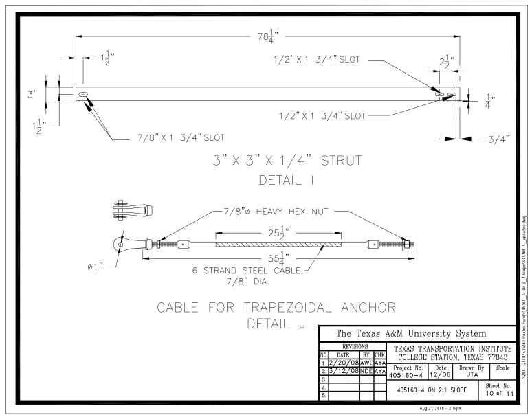
Figure 3.10. Strut and cable anchor details.
