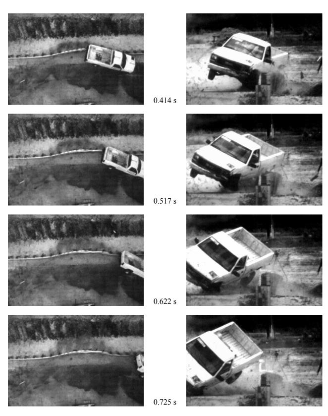
Figure C2. Sequential photographs for test 405160-4-1 (overhead and frontal views) (continued).
