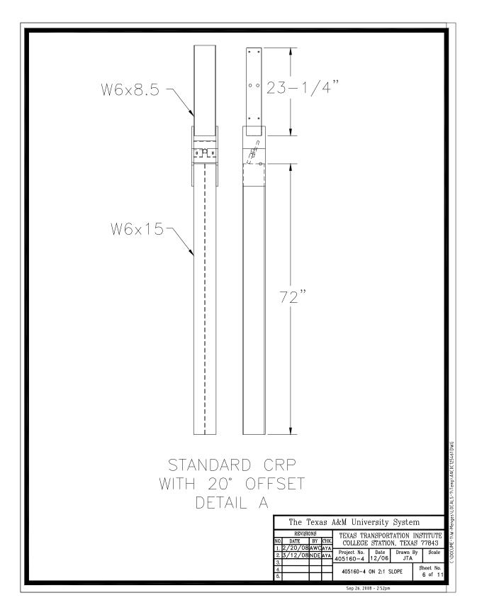
Figure 3.6. Standard CRP post detail.
