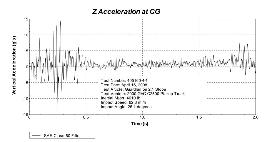
Figure D4. Vehicle vertical accelerometer trace for test 405160-4-1 (accelerometer located at center of gravity).
