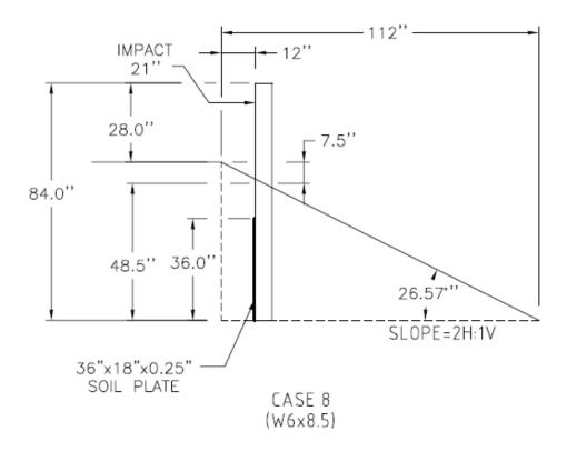
Figure 2.18. Placement of the new post design (Case 8).
