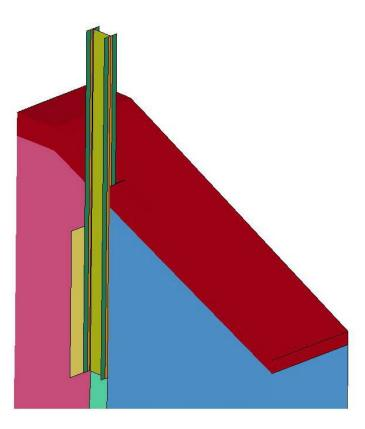
Figure 2.22. Model of steel post with soil plate.
