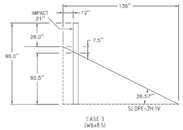
Figure 2.12. Cross section of post placement.
