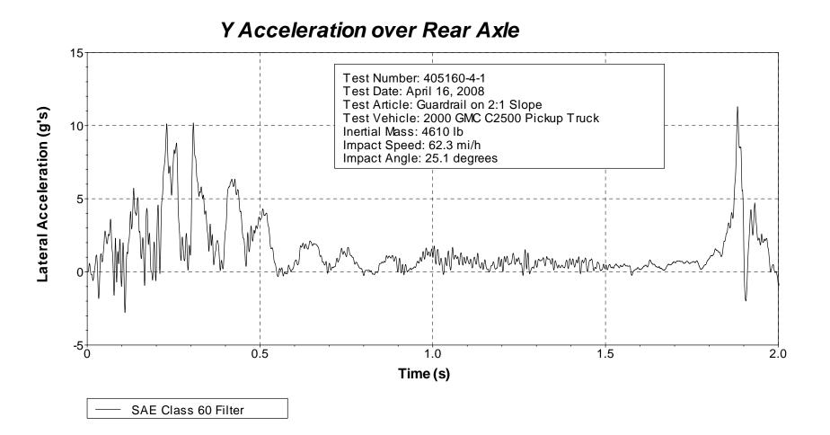
Figure D6. Vehicle lateral accelerometer trace for test 405160-4-1 (accelerometer located over rear axle).
