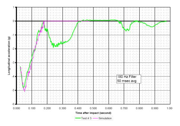
Figure 2.7. Acceleration for both bogie test 3 and its simulation.
