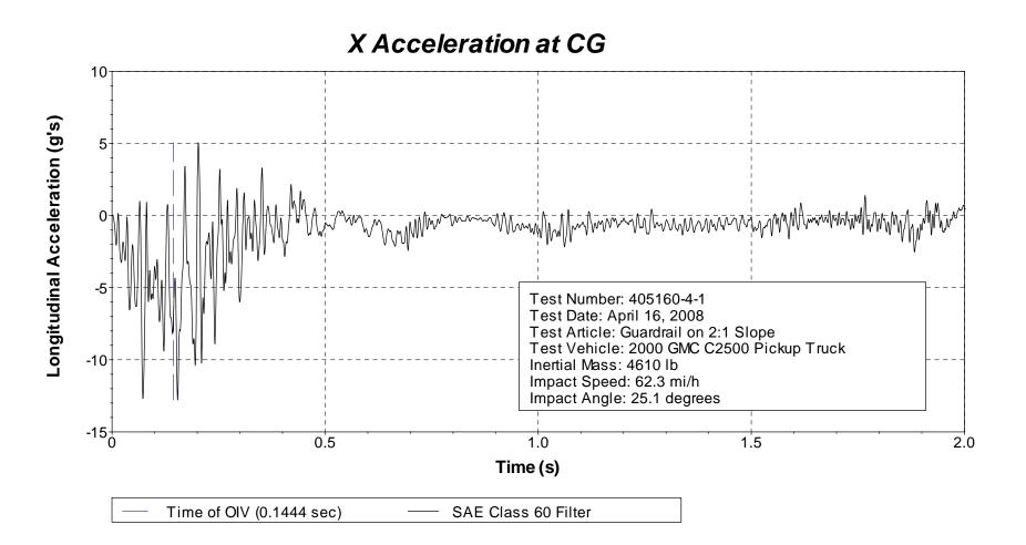
Figure D2. Vehicle longitudinal accelerometer trace for test 405160-4-1 (accelerometer located at center of gravity).
