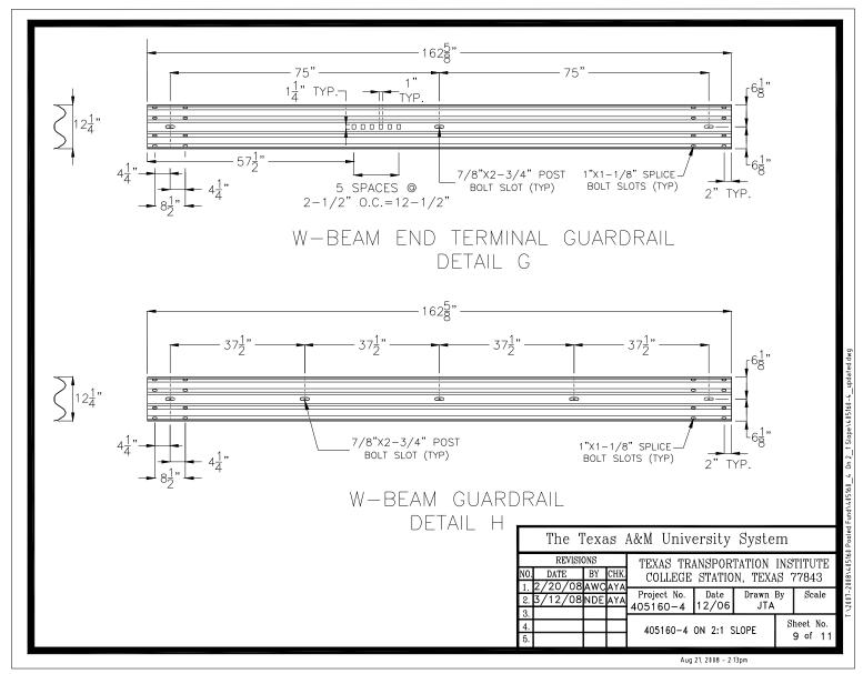
Figure 3.9. W-Beam rail element details.
