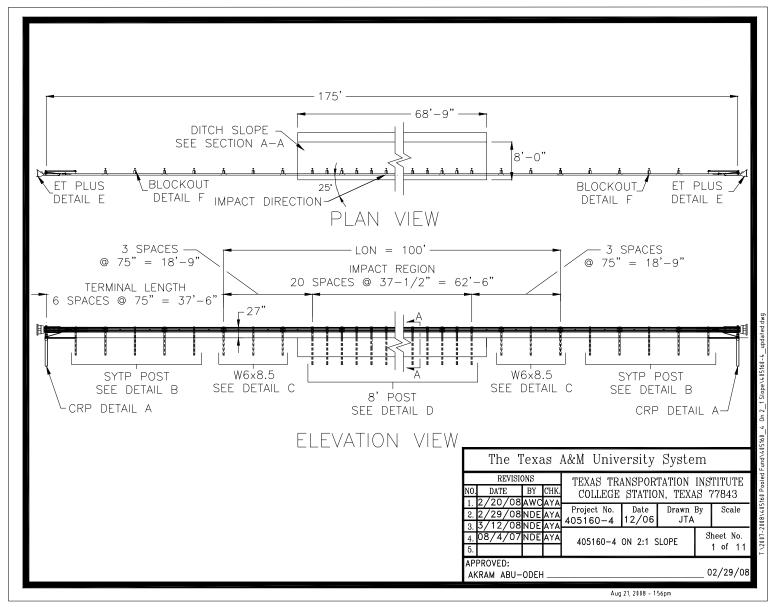
Figure 3.1. Details of guardrail on 2H:1V slope.
