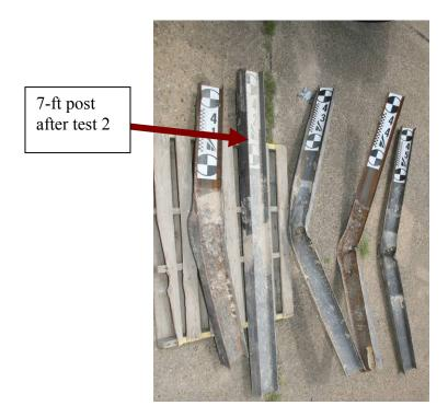
Figure 2.21. Pull posts from test 1,2,3,4 and 5.
