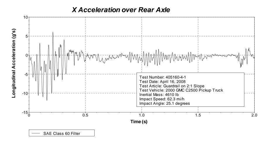
Figure D5. Vehicle longitudinal accelerometer trace for test 405160-4-1 (accelerometer located over rear axle).
