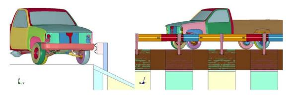
Figure 2.10. Guardrail on slope system with 6 ft-3 inch post spacing.
