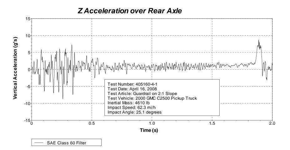
Figure D7. Vehicle vertical accelerometer trace for test 405160-4-1 (accelerometer located over rear axle).
