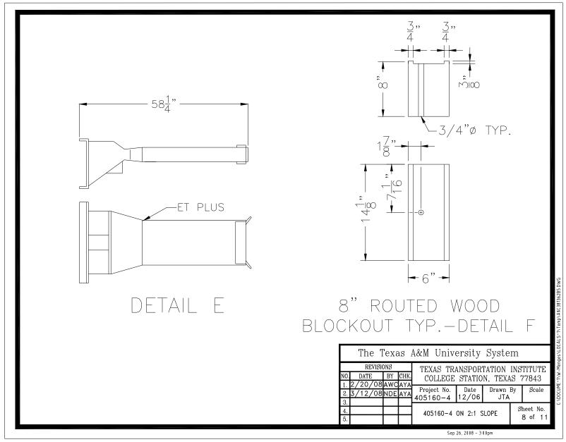
Figure 3.8. ET PLUS head and 8-inch block details.
