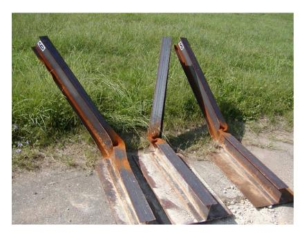
Figure 2.20. Deformed posts after test 6, 7 and 8.
