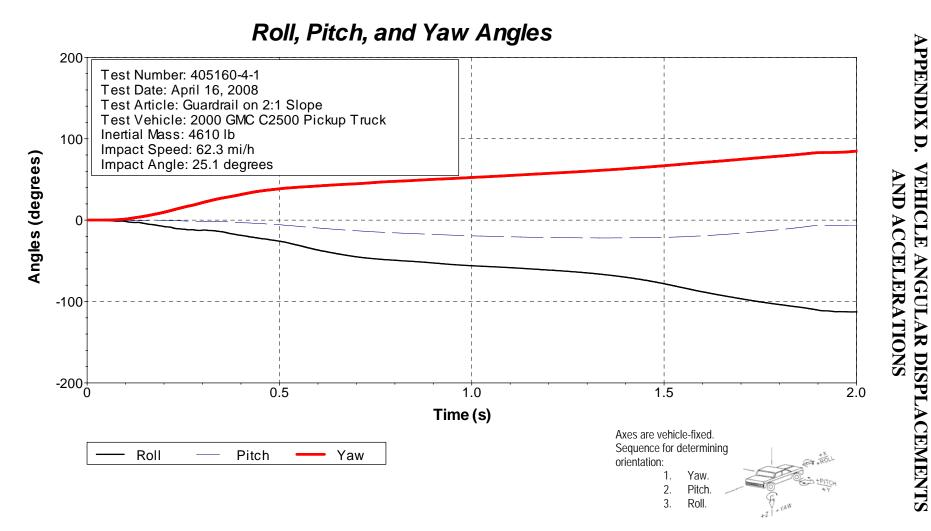
Figure D1. Vehicle angular displacements for test 405160-4-1.
