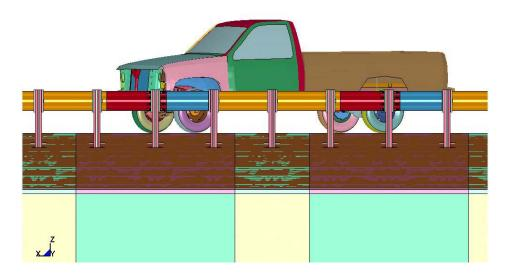
Figure 2.11. Guardrail on slope system with 3 ft-1.5 inch post spacing.
