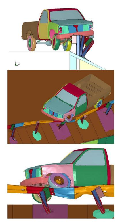
Figure 2.9. Vehicle-barrier interaction associated with test 3-11 impact of a guardrail on 2H:1V slope with 8-ft long posts spaced at 6 ft-3 inch.
