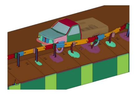
Figure 2.15. Guardrail on slope system with 6 ft-3 inch post spacing and 10-Gauge W-Beam.
