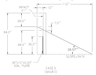
Figure 2.16. Placement of the new post design (Case 6).
