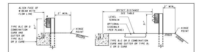
\* FACE OF W-BEAM CAN BE MOVED BACK 6" WITH EITHER 12" OR 8" OFFSET BLOCK WITH ENGINEER'S APPROVAL. WHEN USED WITH TRAFFIC BARRIER END TREATMENT. CURB SHALL BE TAPERED DOWN AND CURB HEIGHT SHALL NOT EXCEED 2".
