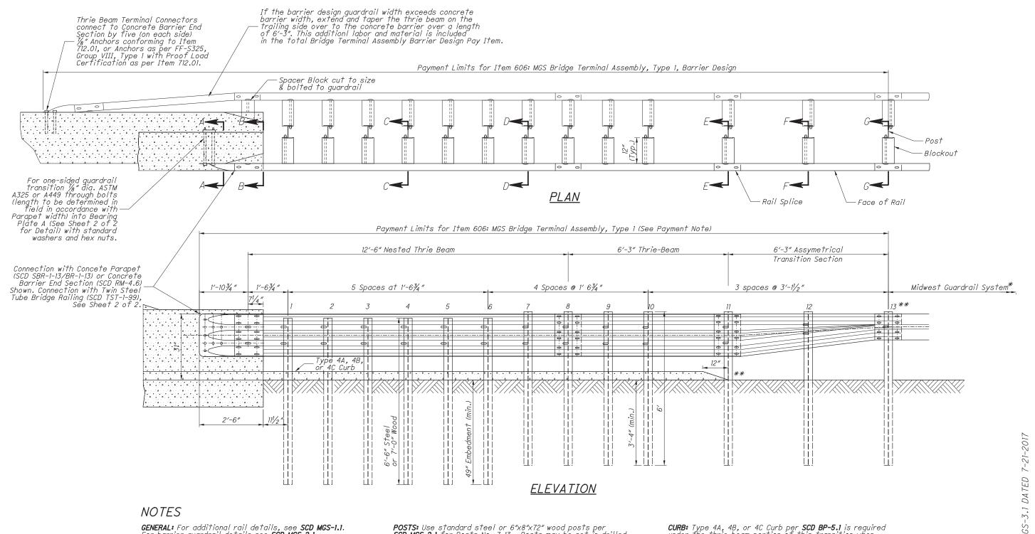
GENERAL: For additional rail details, see SCD MGS-1.1. For barrier guardrail details see SCD MGS-2.1. See Sheet 2 for Sections (single sided BTA shown).
