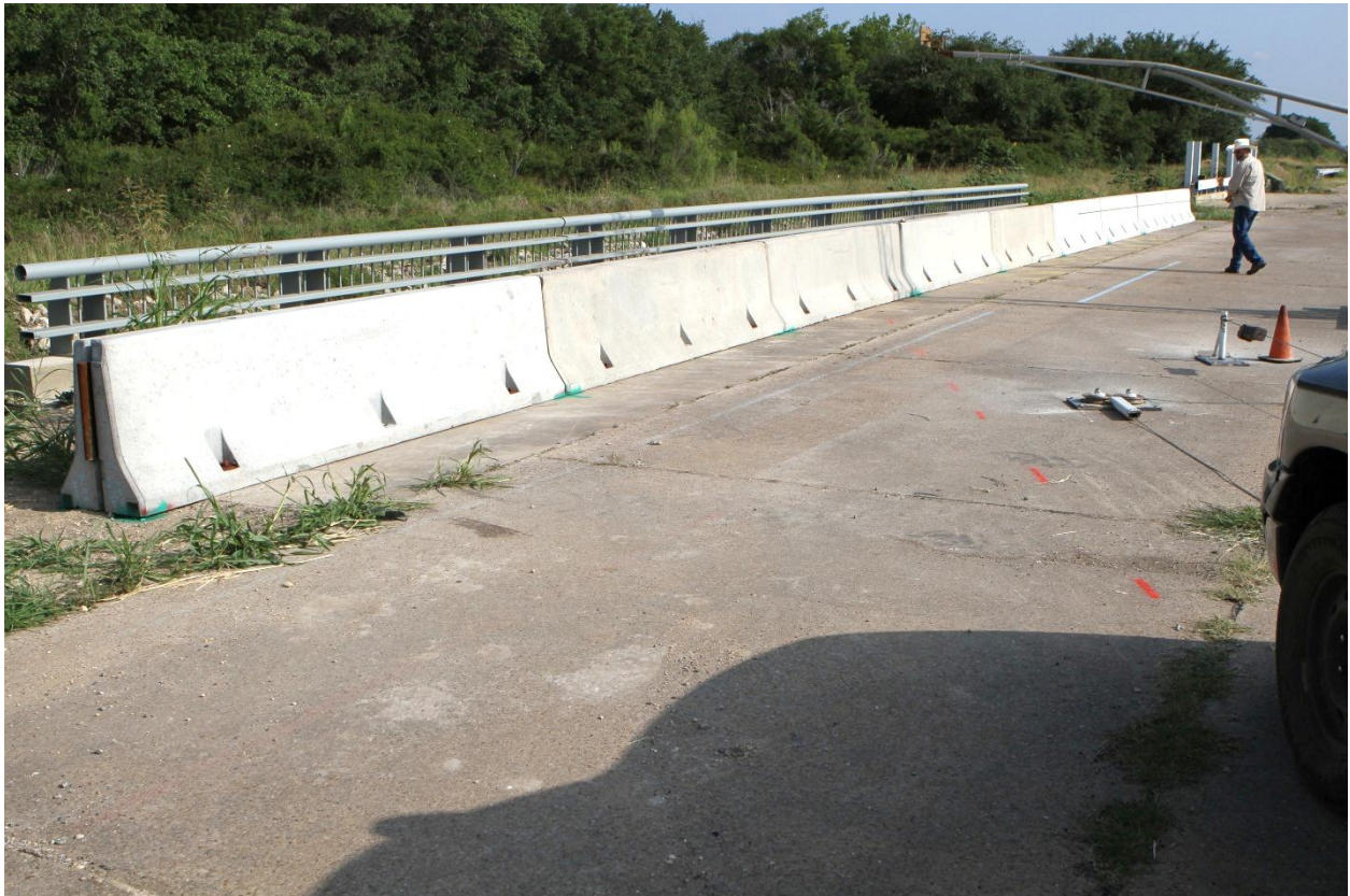
Figure 2.2. EASI-SET ® Industries J-J Hooks/ MASH proprietary bolt-down barrier system prior to testing.
