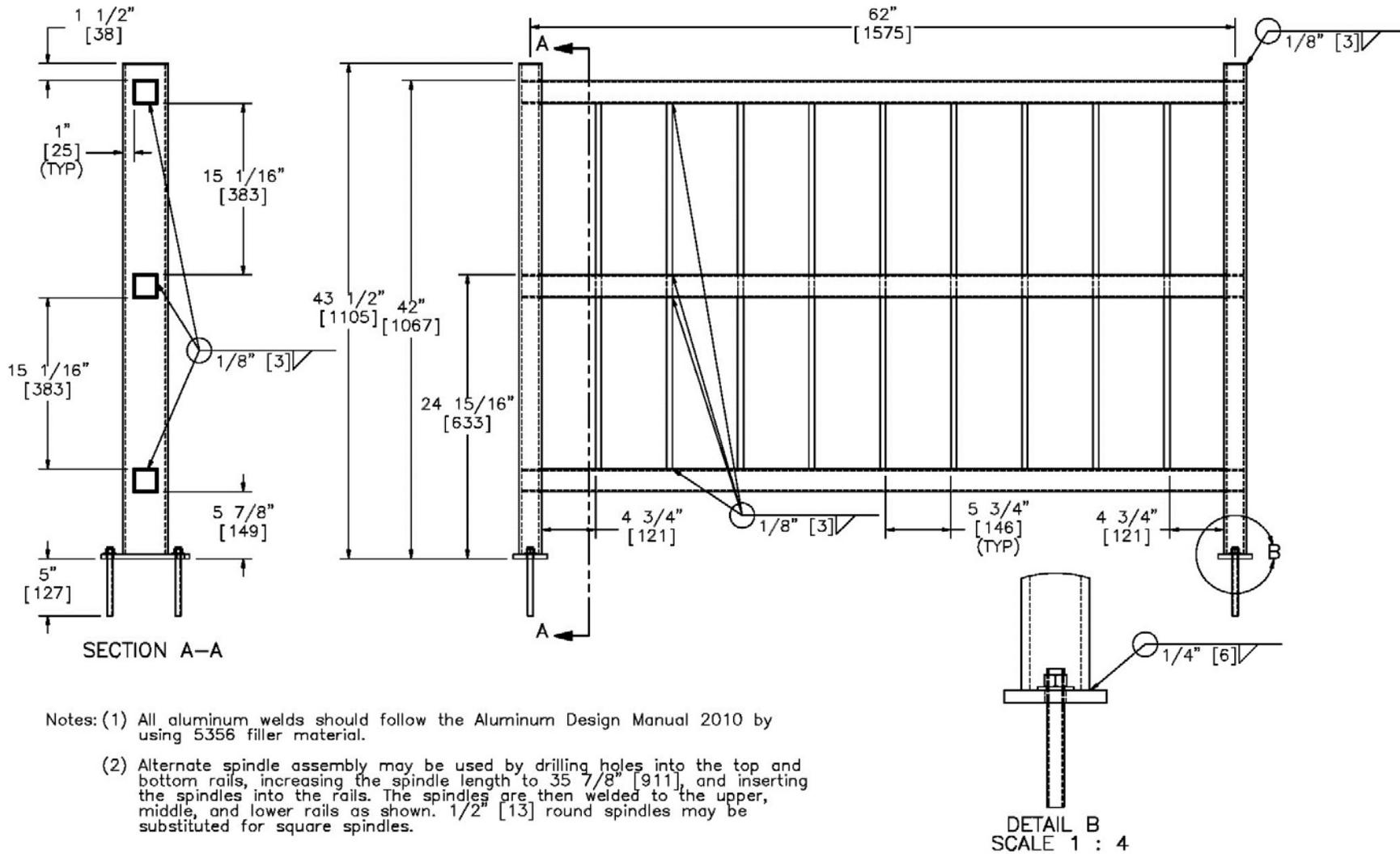
Figure 6. Schematic of Aluminum Pedestrian Rail - Final Design.
