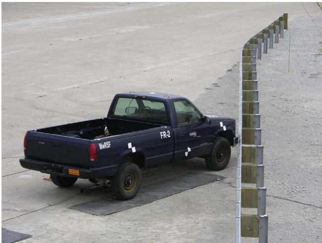
Fig. 2. MGS installed with a 7:1 flare.
