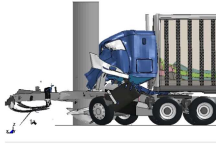
Figure 62. [CONTINUED] Sequential Views of Test 429730-2 and the FEA Results.
