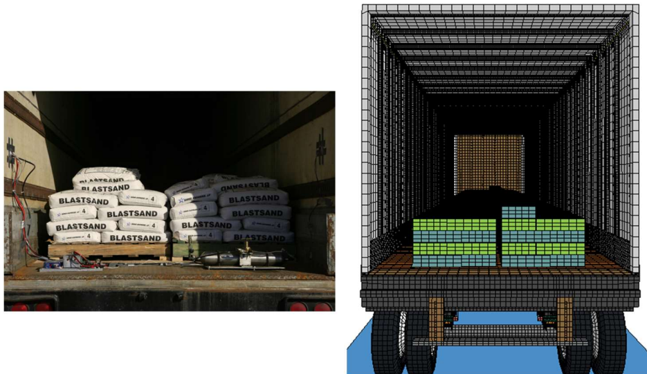
Figure 59. Test and FE Model Ballast.
