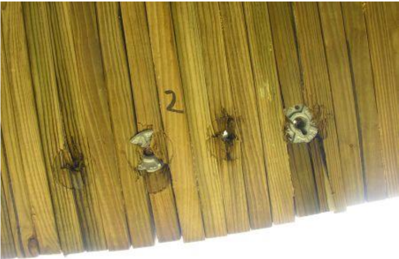
Figure 14. Bridge Deck Damage, Test No. WVS-2
