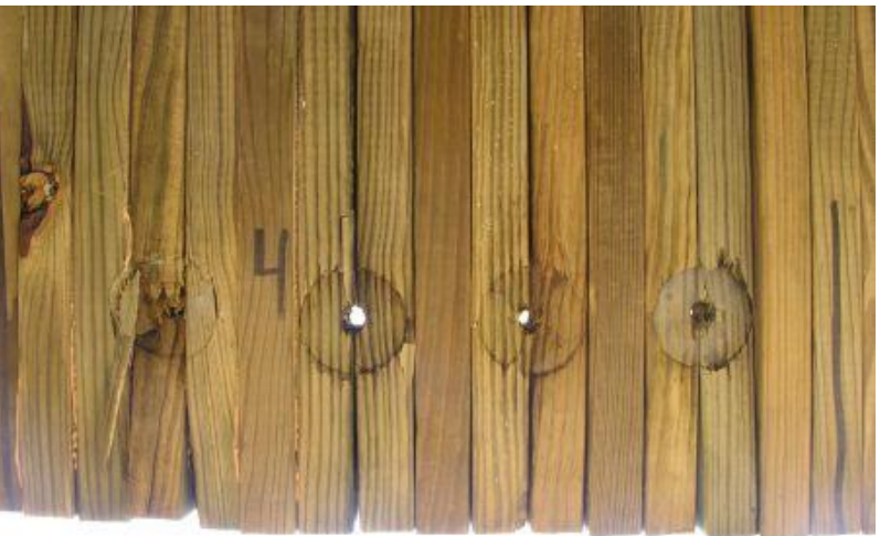
Figure 20. Bridge Deck Damage, Test No. WVS-4
