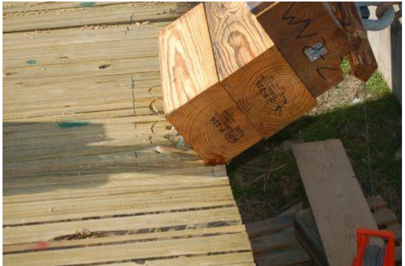
Figure 13. Component Damage and Permanent Set Deflection, Test No. WVS-2
