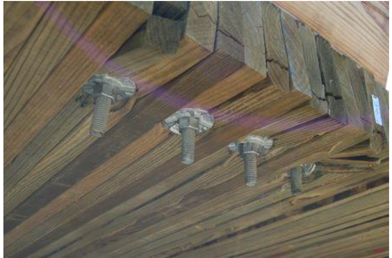
Figure 19. Component Damage and Permanent Set Deflection, Test No. WVS-4
