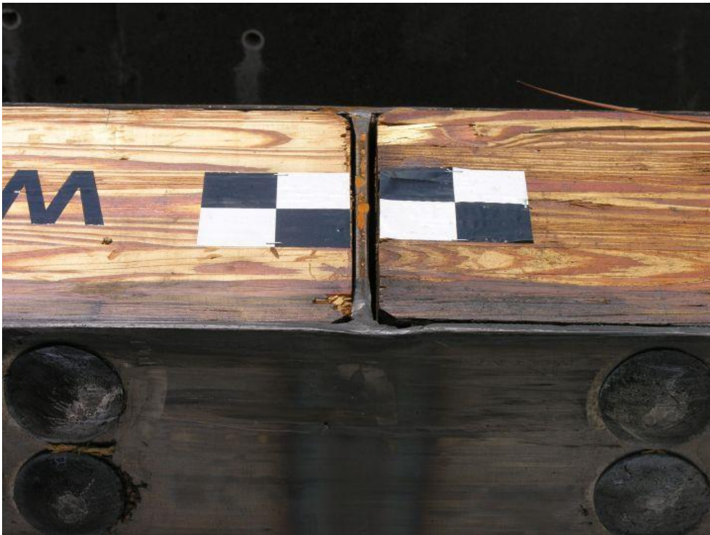
Figure 74. System Damage at Joint Between Post Nos. 4 and 5, Test No. WVBR-1
