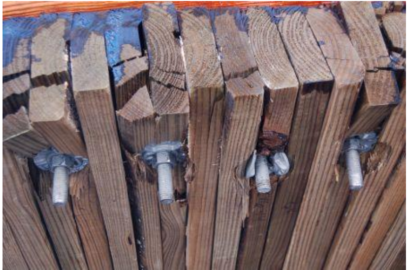
Figure 16. Component Damage and Permanent Set Deflection, Test No. WVS-3
