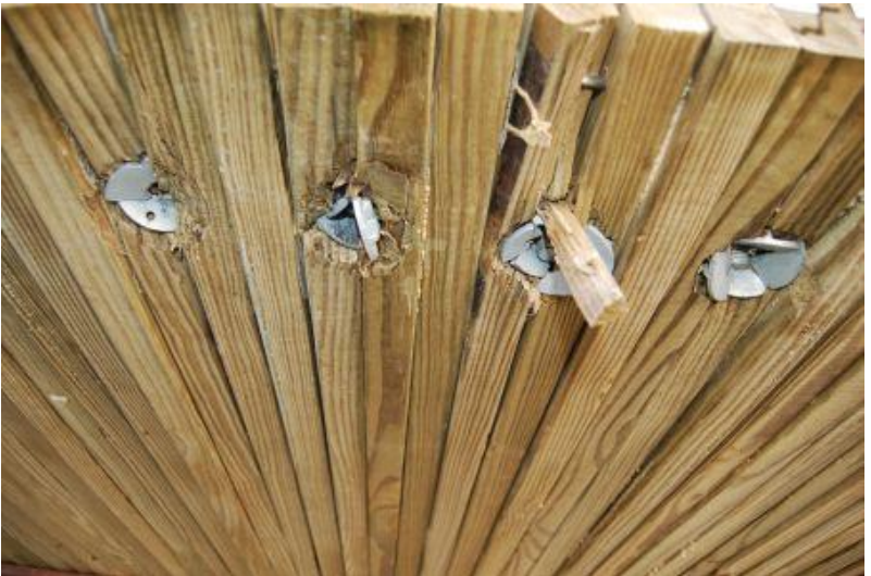
Figure 10. Component Damage and Permanent Set Deflection, Test No. WVS-1
