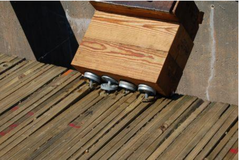
Figure 16. Component Damage and Permanent Set Deflection, Test No. WVS-3
