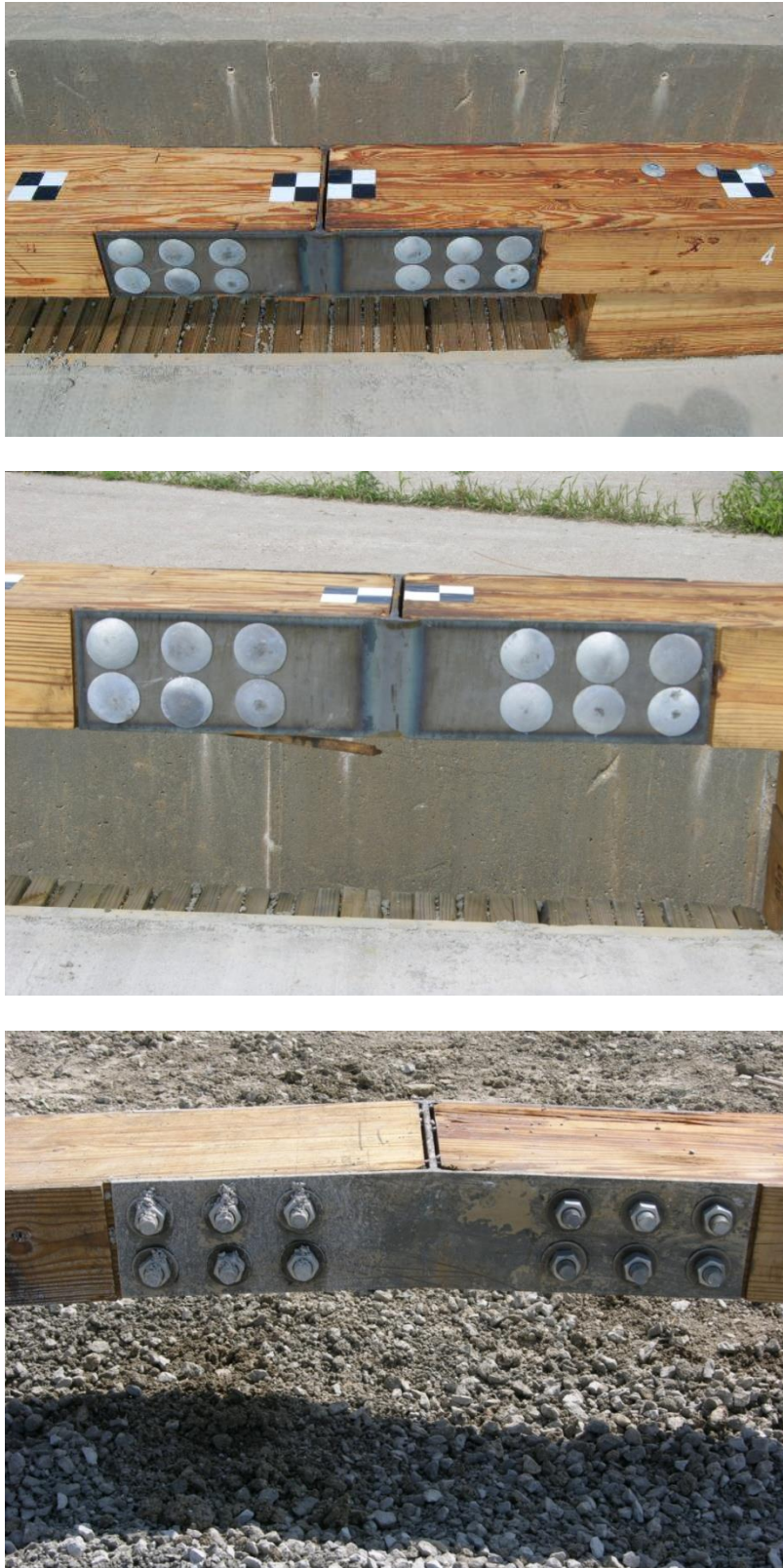
Figure 59. Splice Plate Connections for Glulam Rail, Test No. WVBR-1
