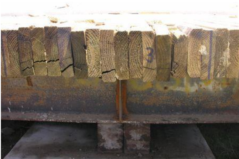
Figure 17. Bridge Deck Damage, Test No. WVS-3
