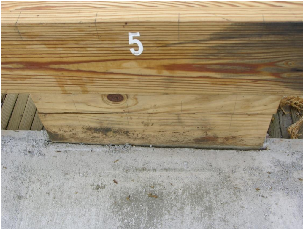
Figure 75. Concrete Gaps at Post Nos. 4 and 5, Test No. WVBR-1
