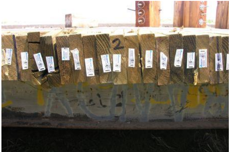
Figure 14. Bridge Deck Damage, Test No. WVS-2
