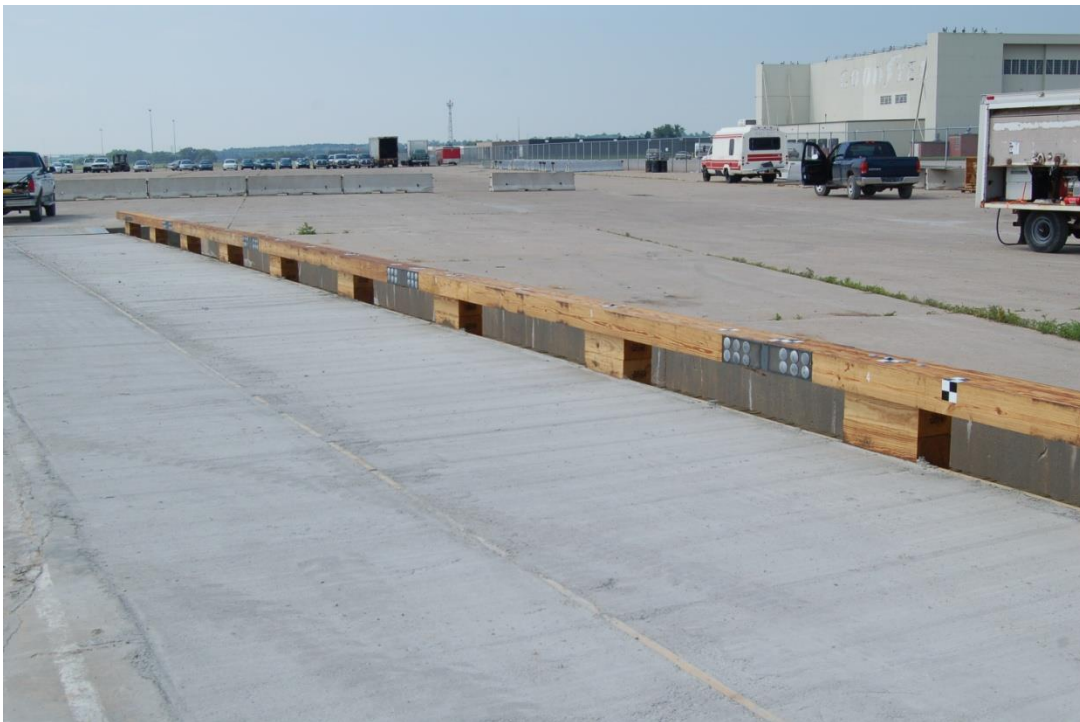
Figure 57. Curb-Type Bridge Railing System, Test No. WVBR-1
