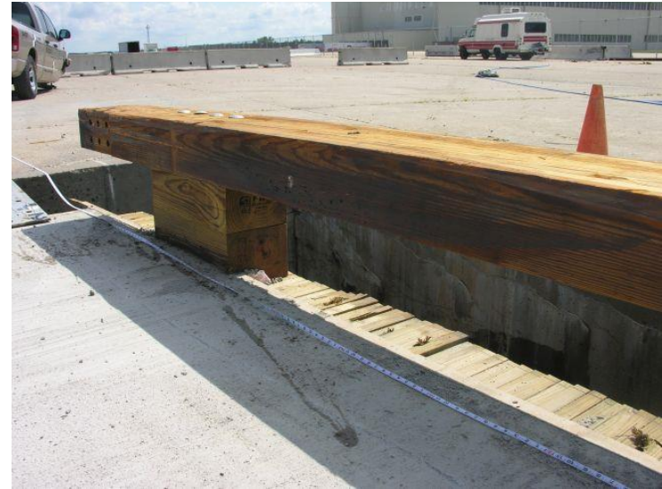
Figure 73. Rail Damage and Displacement, Test No. WVBR-1
