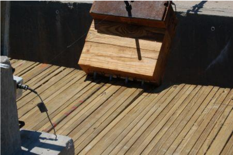
Figure 19. Component Damage and Permanent Set Deflection, Test No. WVS-4
