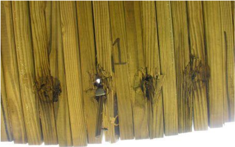
Figure 11. Bridge Deck Damage, Test No. WVS-1
