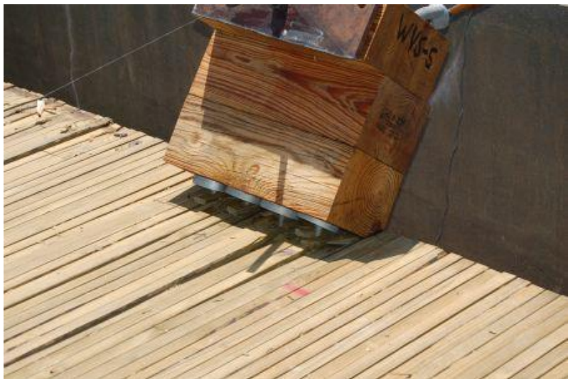
Figure 22. Component Damage and Permanent Set Deflection, Test No. WVS-5
