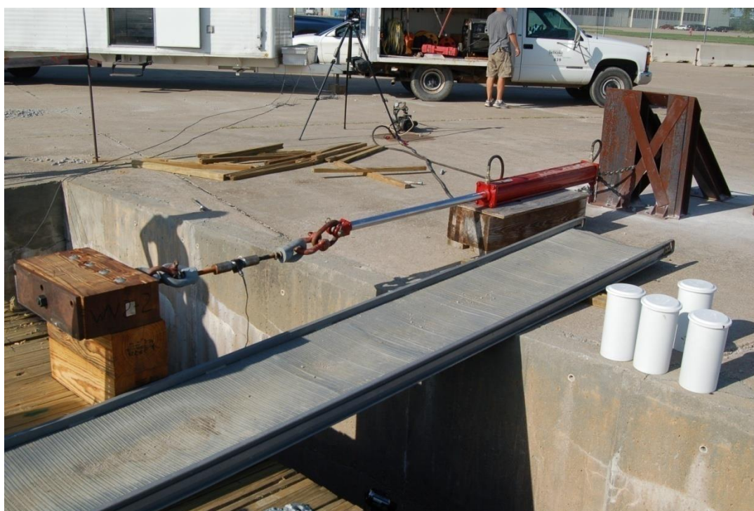
Figure 8. Modified Static Test Setup - Test Nos. WVS-1 through 5
