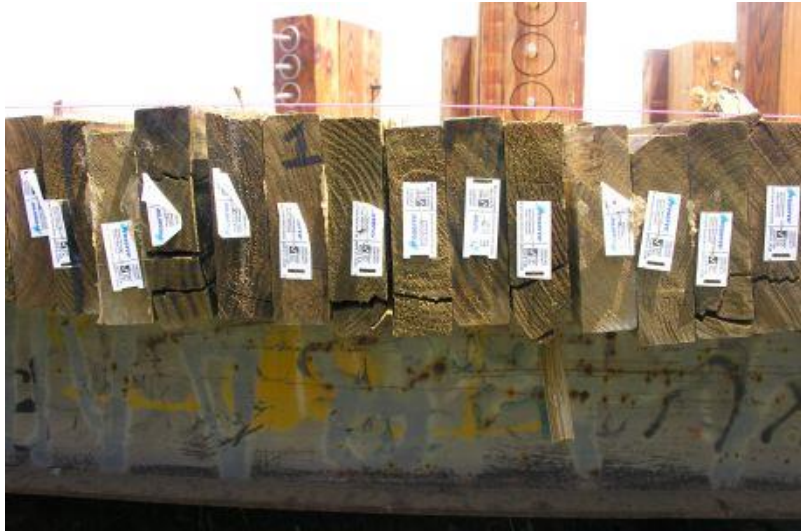
Figure 11. Bridge Deck Damage, Test No. WVS-1
