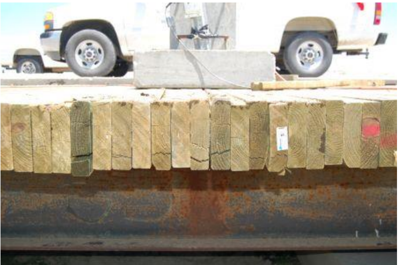
Figure 20. Bridge Deck Damage, Test No. WVS-4
