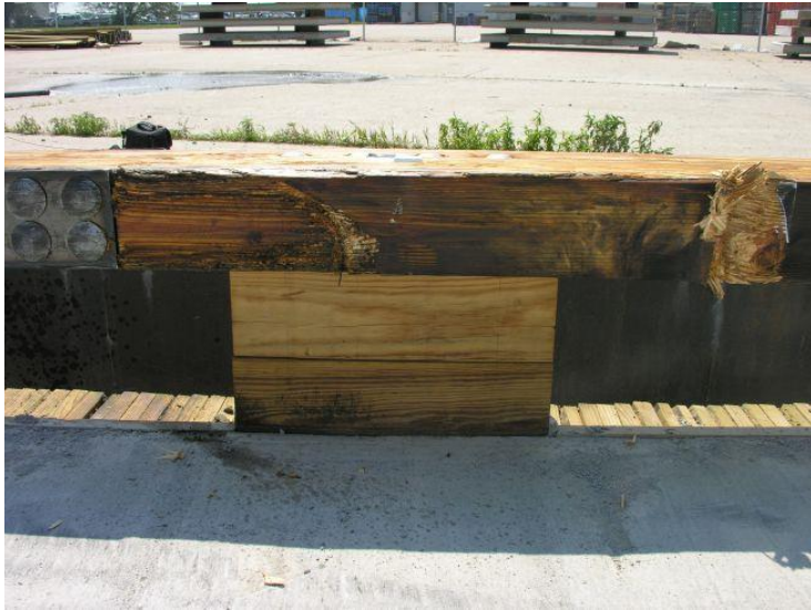
Figure 73. Rail Damage and Displacement, Test No. WVBR-1
