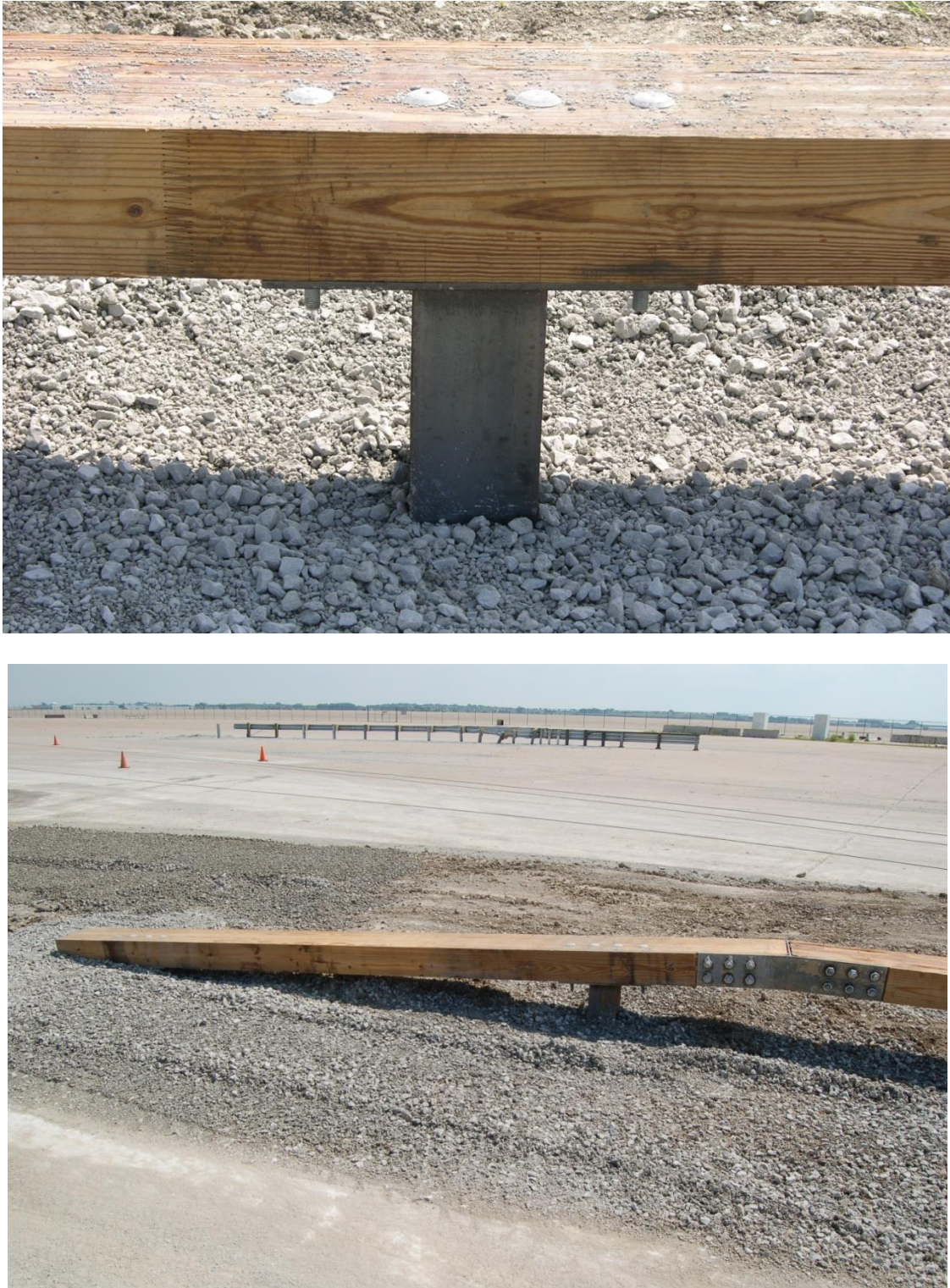
Figure 60. Sloped End Treatment, Test No. WVBR-1
