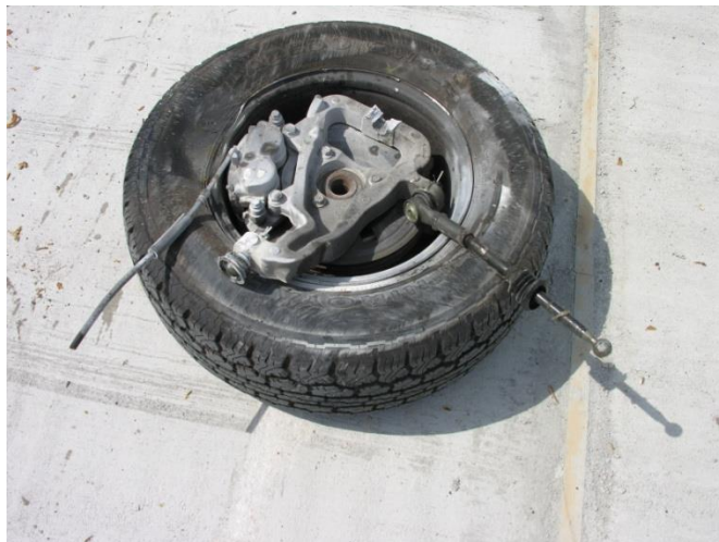
Figure 77. Vehicle Damage at Right-Front Corner, Test No. WVBR-1
