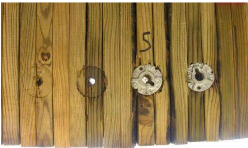
Figure 23. Bridge Deck Damage, Test No. WVS-5
