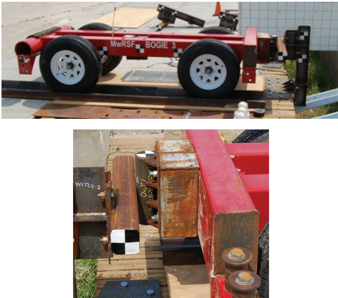
Figure 13. Bogie Vehicle and Bogie Impact Head
