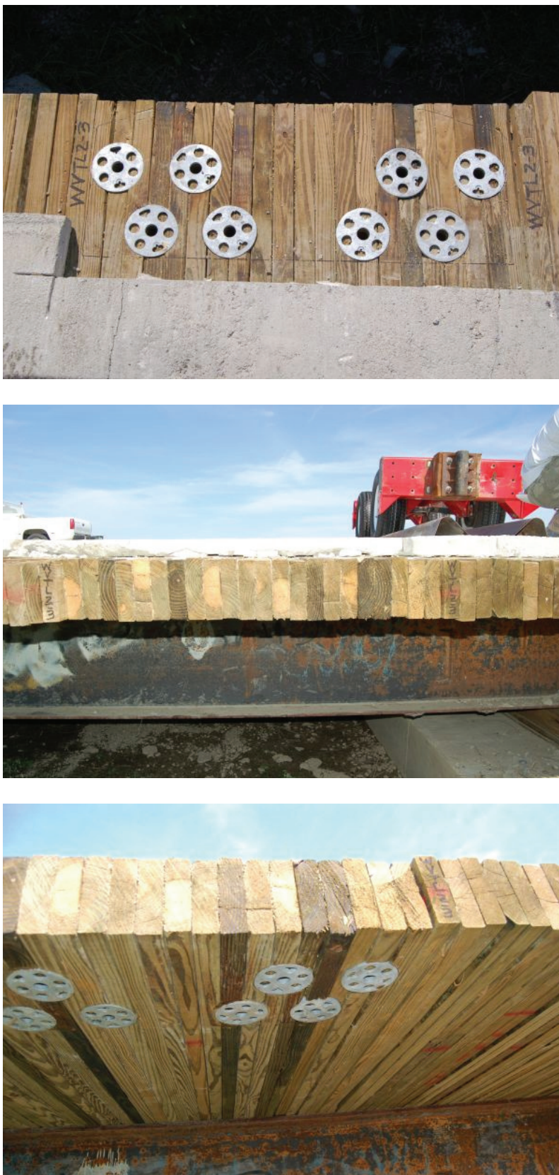
Figure 27. Deck Damage, Test No. WVTL2-3
