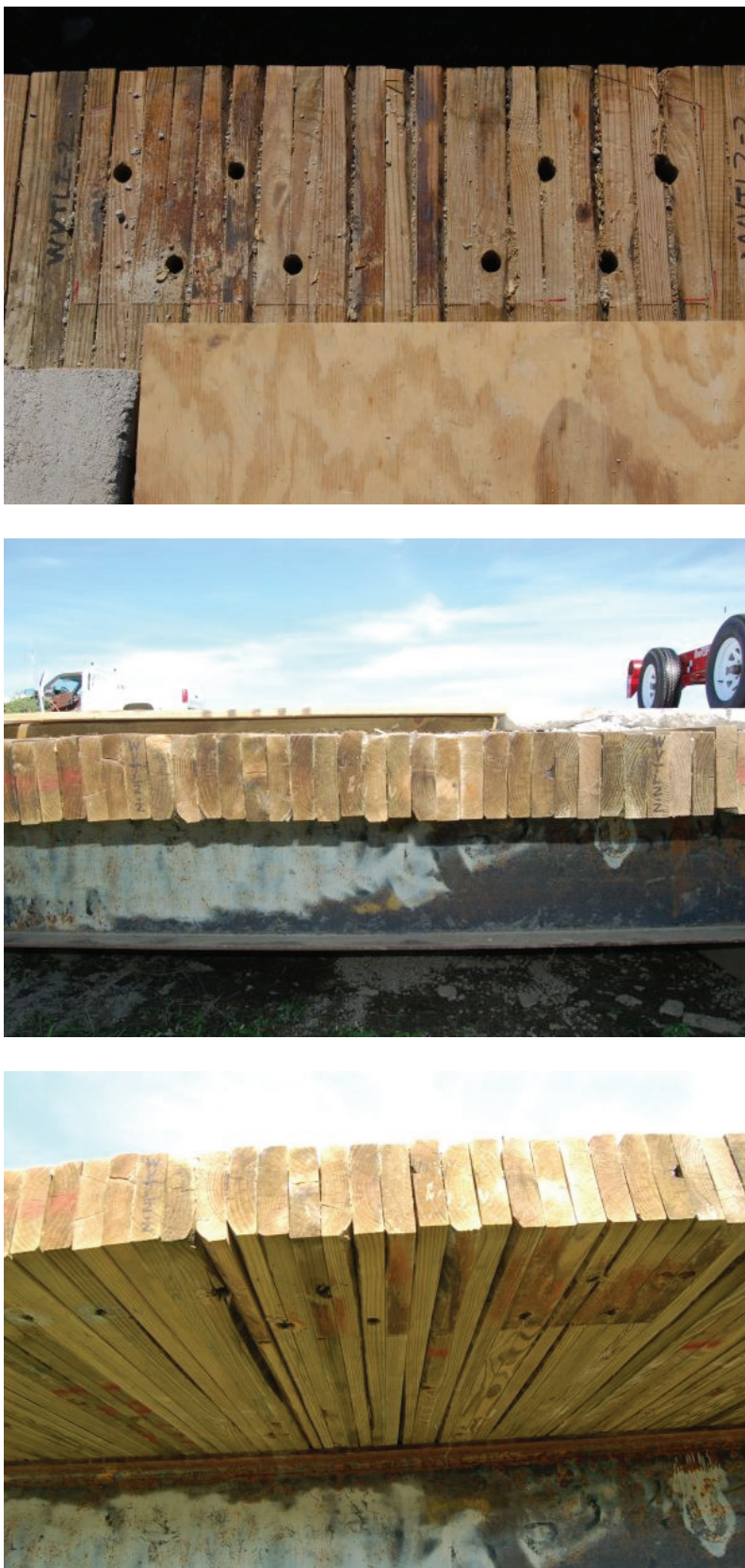
Figure 23. Deck Damage, Test No. WVT2-2
