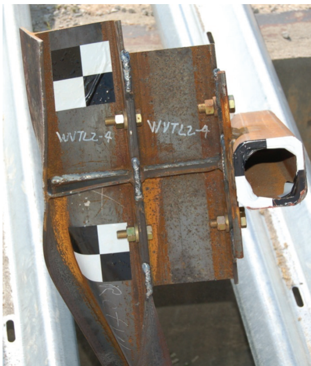
Figure 30. Post Assembly Damage, Test No. WVT2-4
