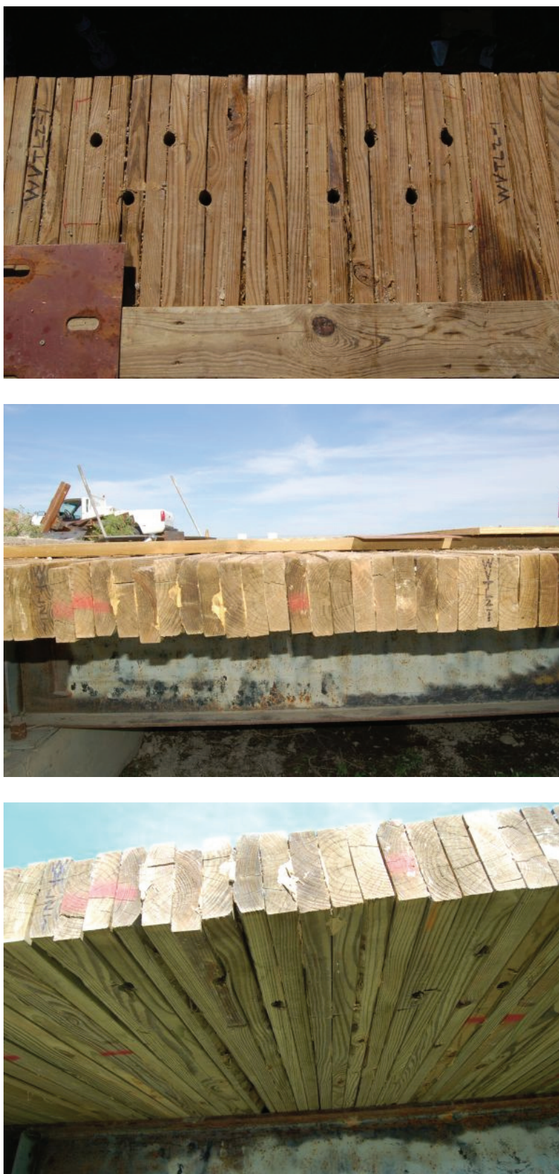
Figure 19. Deck Damage, Test No. WVT2-1
