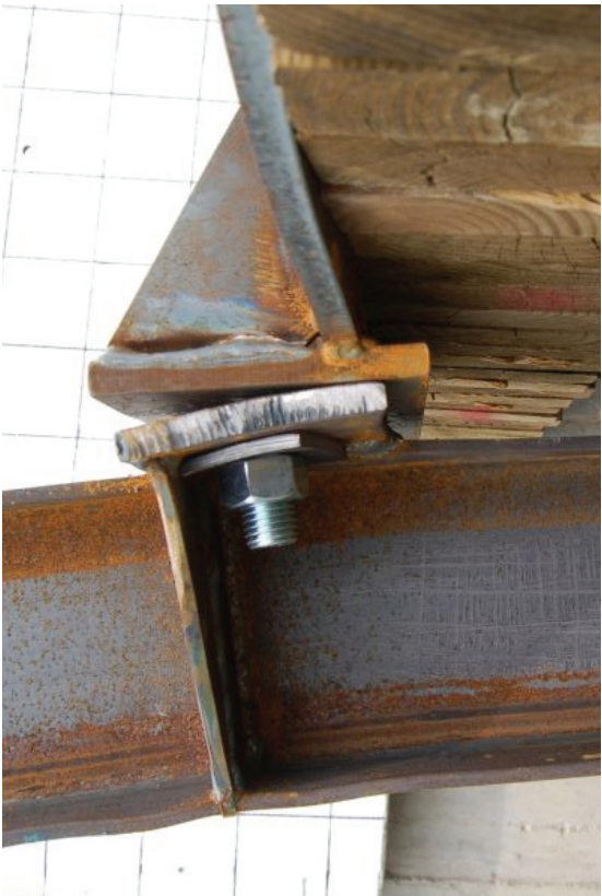
Figure 18. Post Assembly Damage, Test No. WVTL2-1
