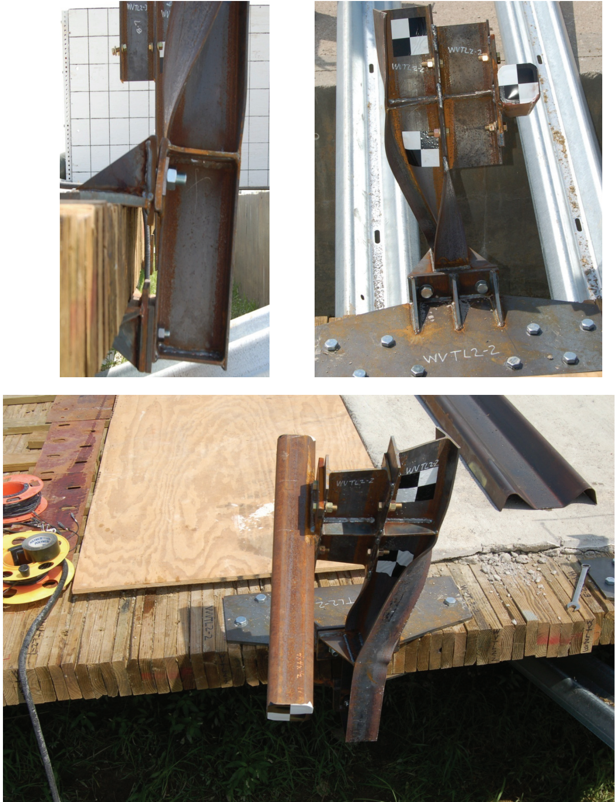
Figure 22. Post Assembly Damage, Test No. WVTL2-2
