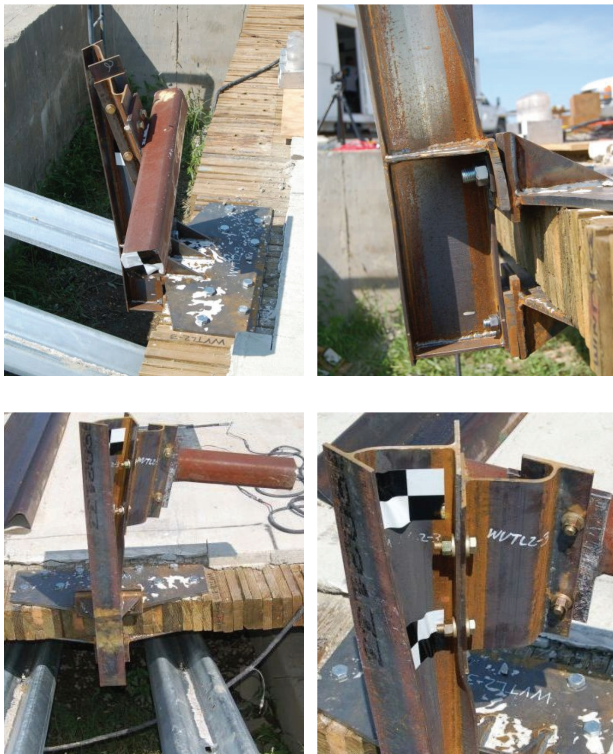
Figure 26. Post Assembly Damage, Test No. WVT2-3
