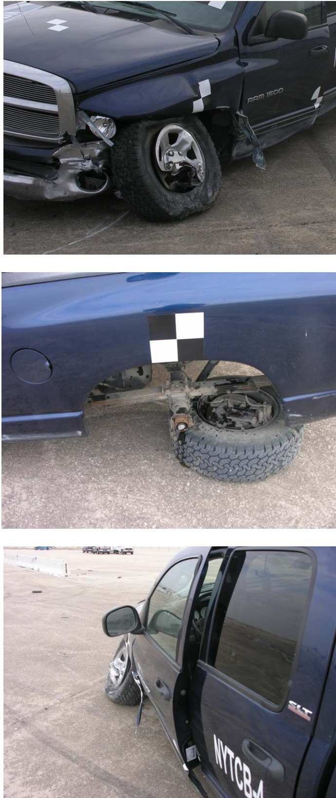
Figure 35. Vehicle Damage, Test NYTCB-4
