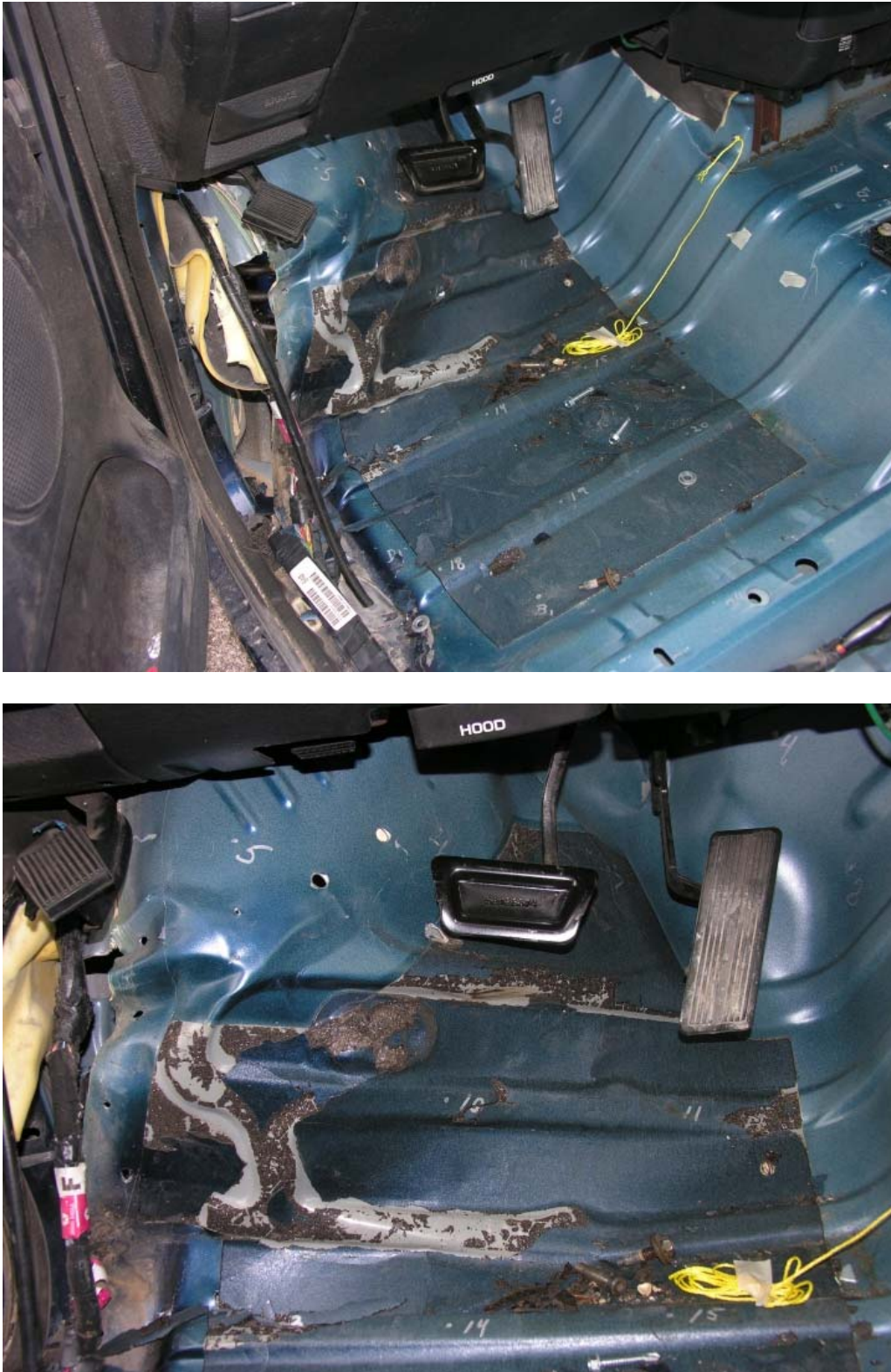
Figure 37. Occupant Compartment Deformation, Test NYTCB-4
