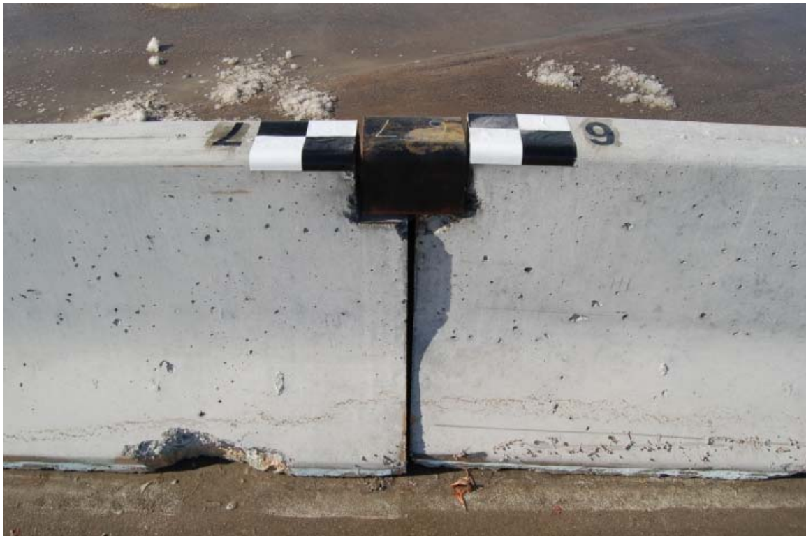
Figure 33. Joint 6-7 Connection Damage, Test NYTCB-4
