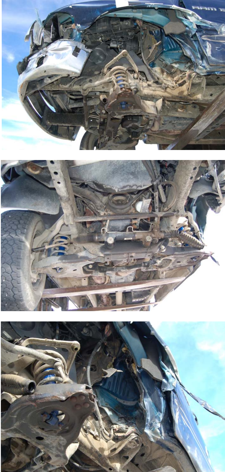
Figure 36. Undercarriage Damage, Test NYTCB-4
