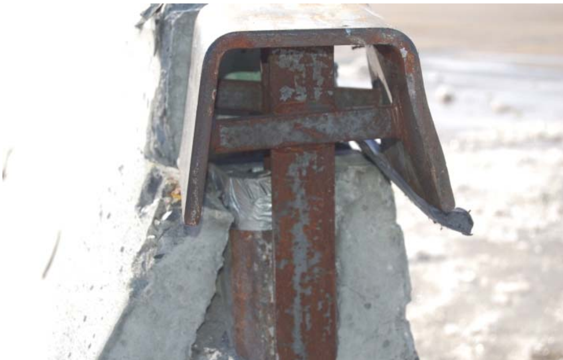
Figure 31. Joint 4-5 Connection Damage (Cont'd), Test NYTCB-4
