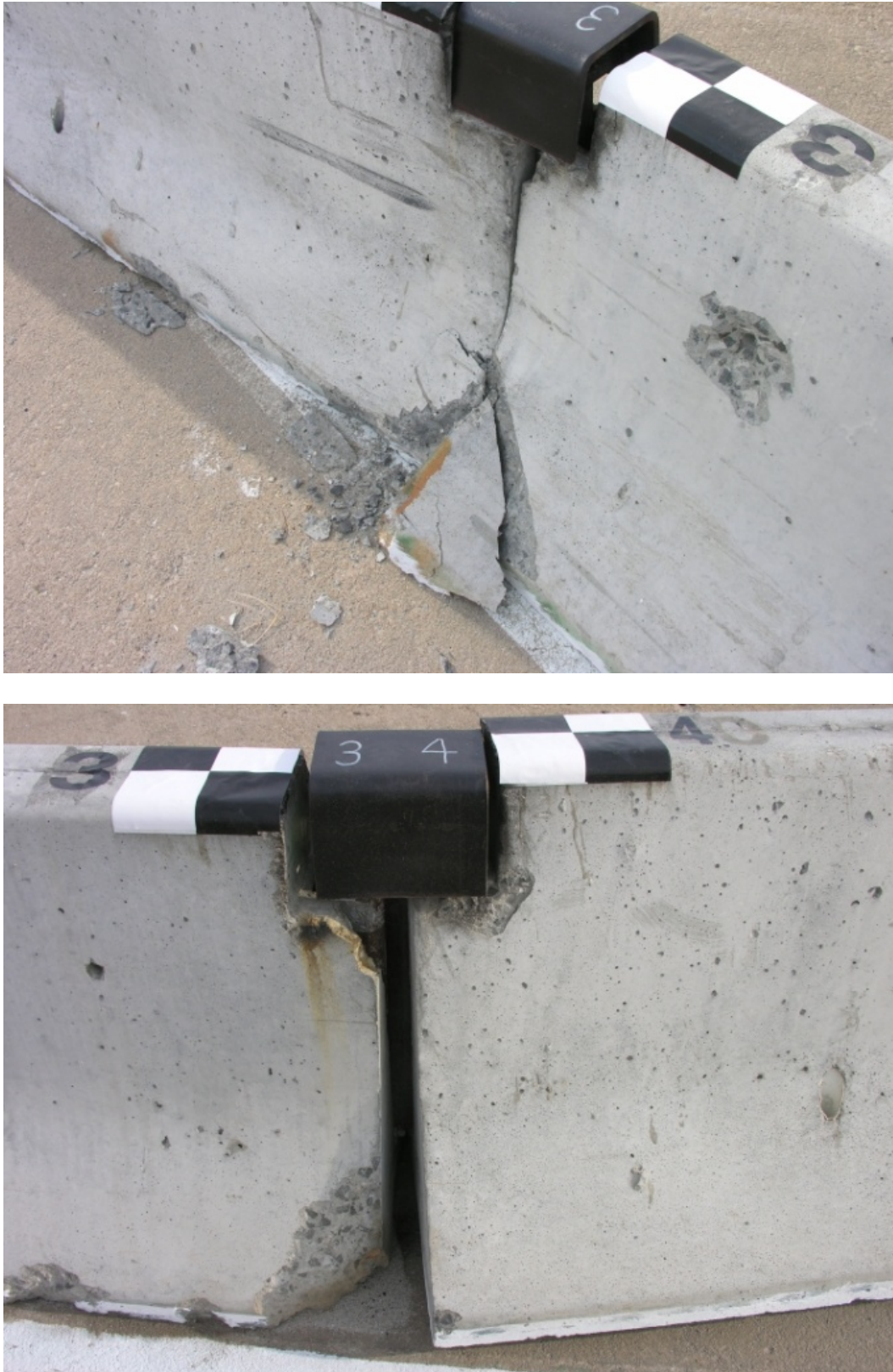
Figure 29. Joint 3-4 Connection Damage, Test NYTCB-4
