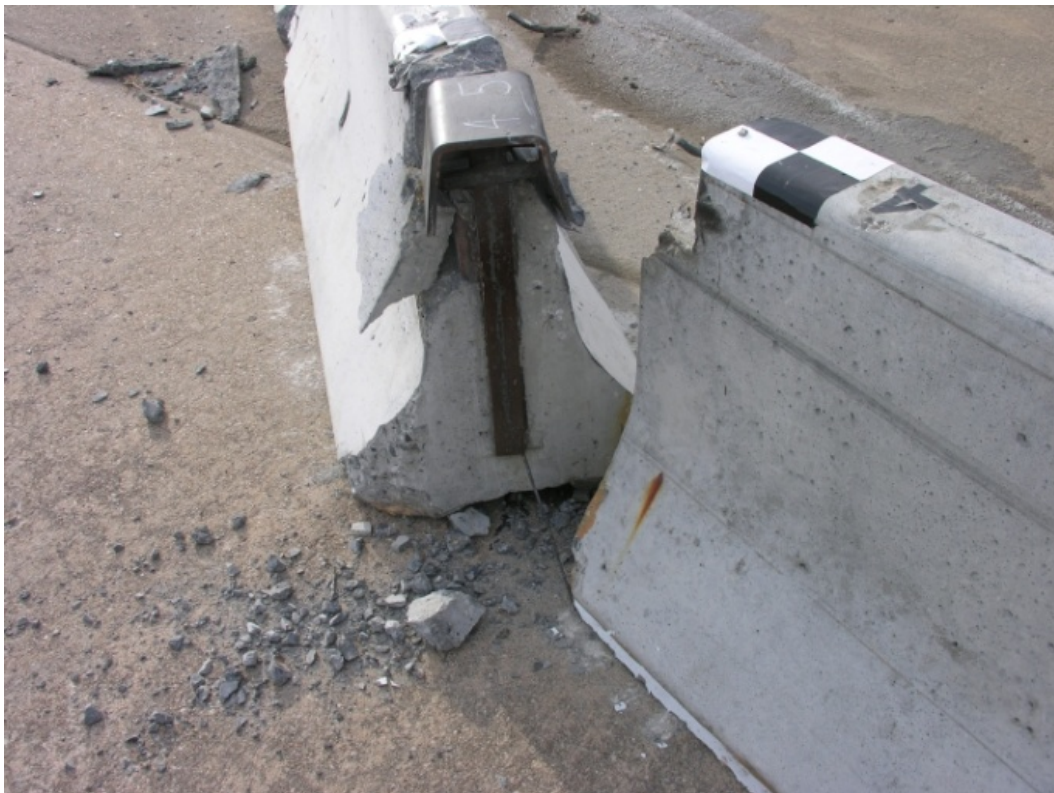
Figure 30. Joint 4-5 Connection Damage, Test NYTCB-4
