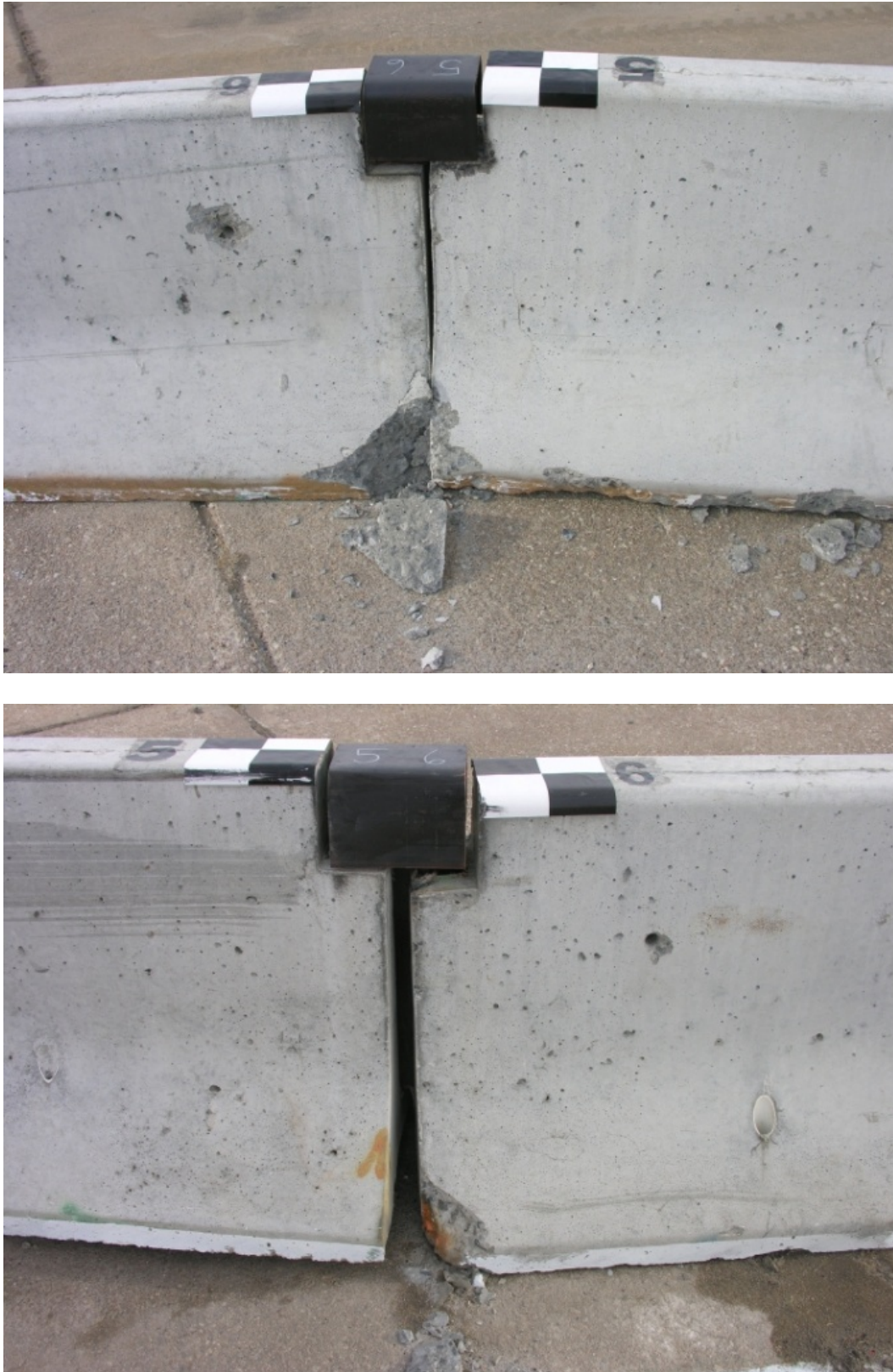
Figure 32. Joint 5-6 Connection Damage, Test NYTCB-4
