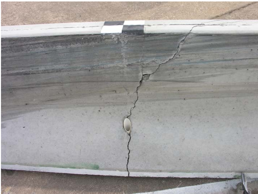
Figure 27. Barrier No. 5 Damage, Test NYTCB-4
