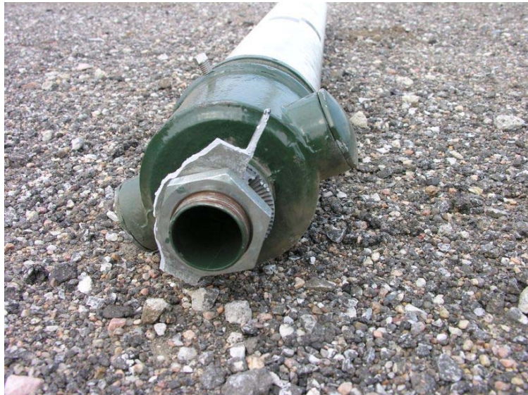
Figure 37. System Damage - Signal and Attachment Bracket, Test No. NYPP-1
