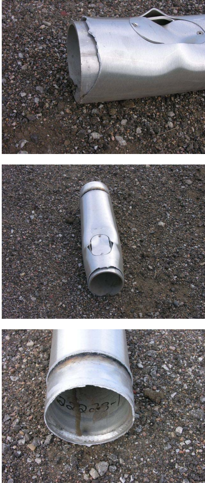
Figure 35. System Damage - Bottom Piece of Pole and Internal Sleeve, Test No. NYPP-1
