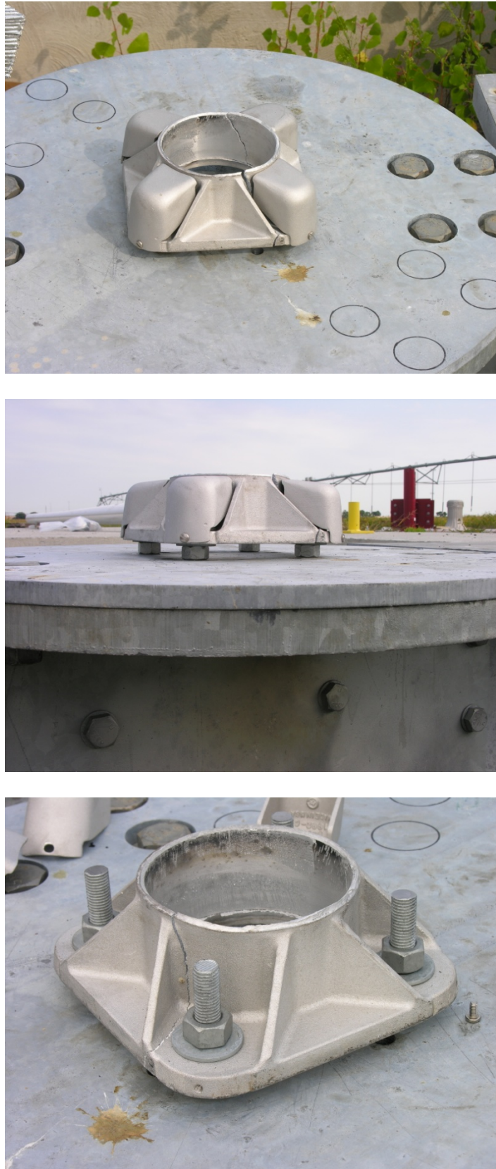
Figure 34. System Damage - Base Plate Cracks and Fractures, Test No. NYPP-1
