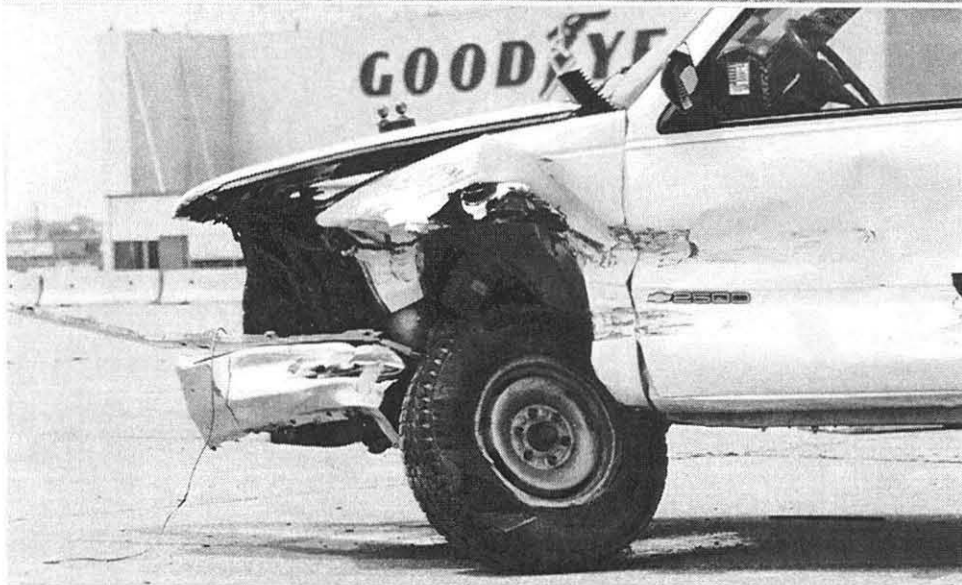
Figure 46. Vehicle Damage, Test ITNJ-2 (Design No. 2)
