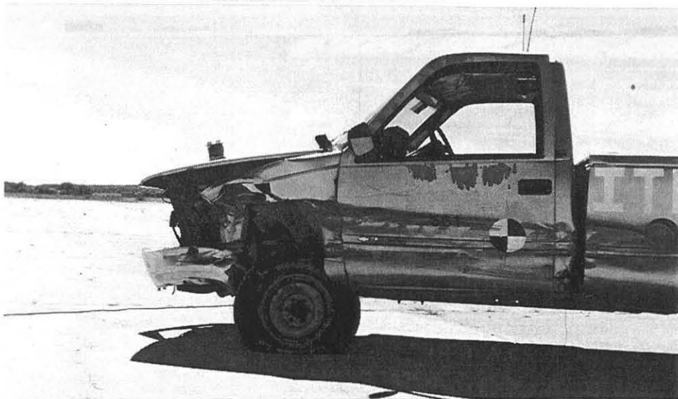
Figure 71. Vehicle Damage, Test ITNJ-4 (Design No. 4)
