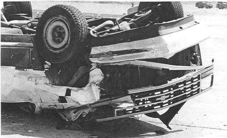
Figure 34. Vehicle Damage, Test ITNJ-1 (Design No. 1)
