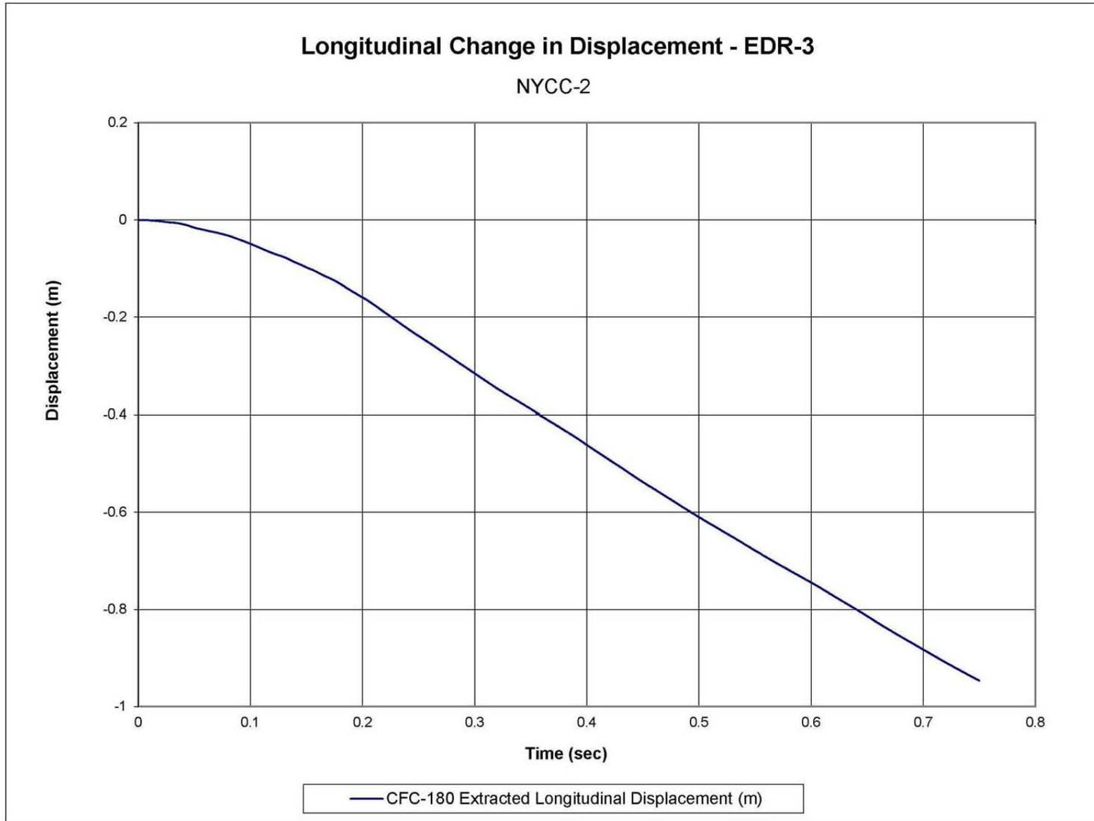
Figure F-11. Longitudinal Occupant Displacement (EDR-3), Test No. NYCC-2
