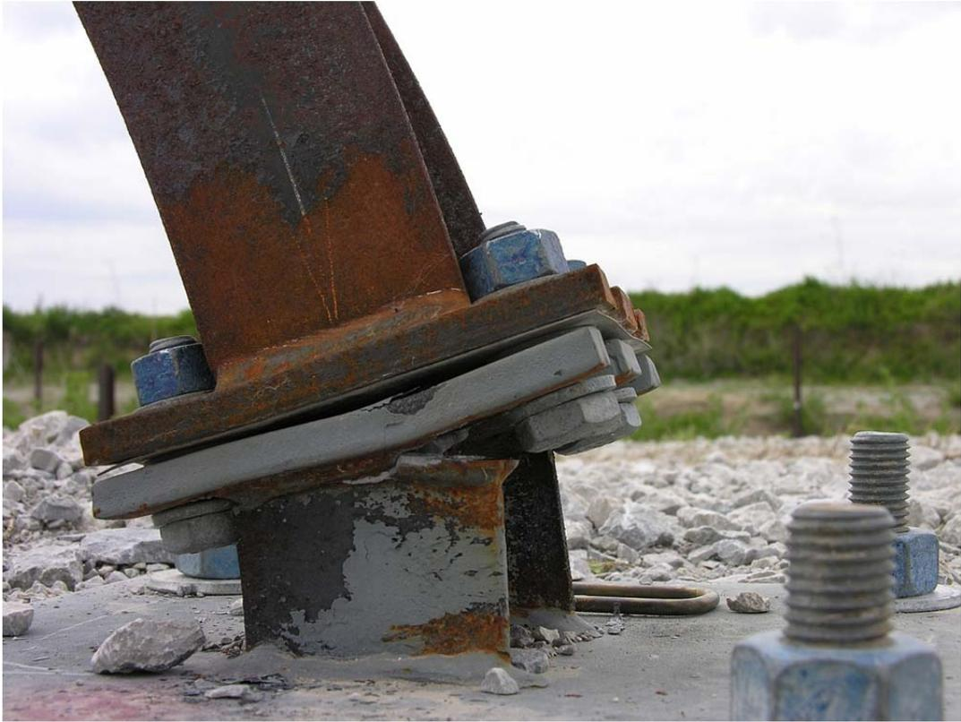
Figure 108. System Damage: Post No. 1, Test No. NYCC-3
