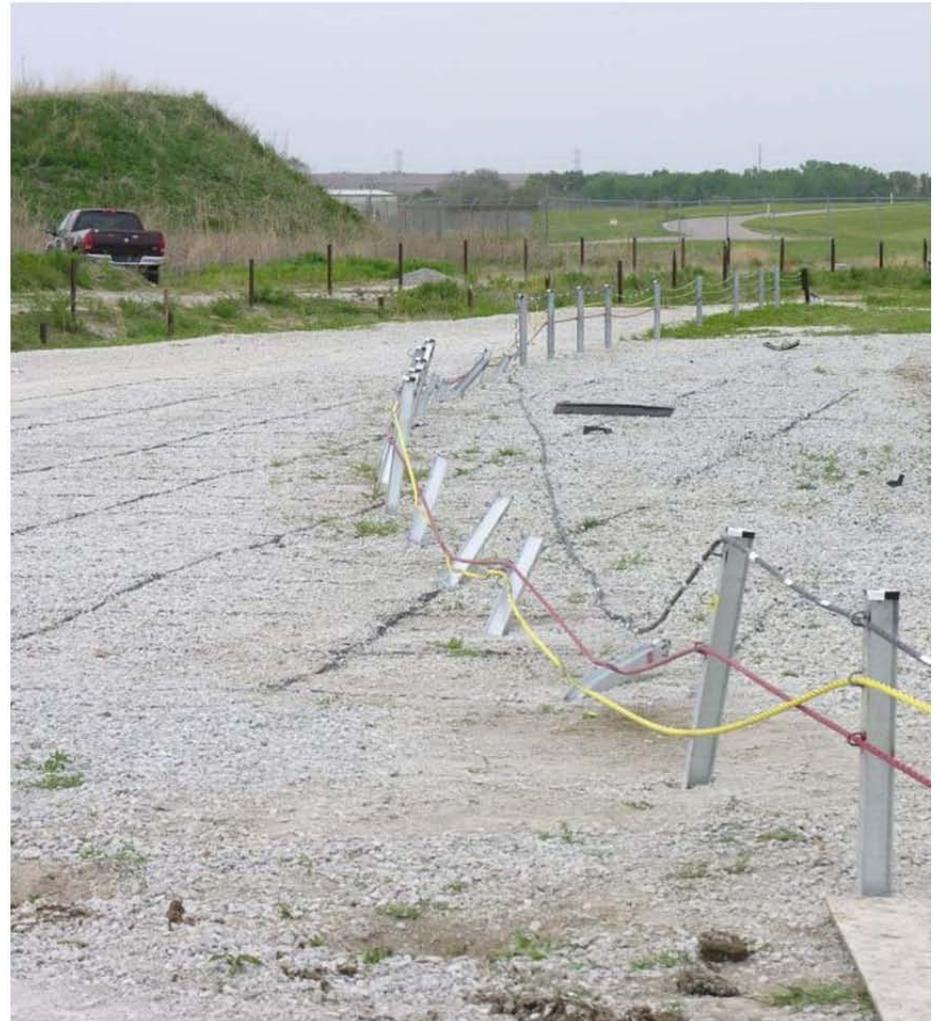
Figure 106. Vehicle Final Position and Trajectory Marks, Test No. NYCC-3
