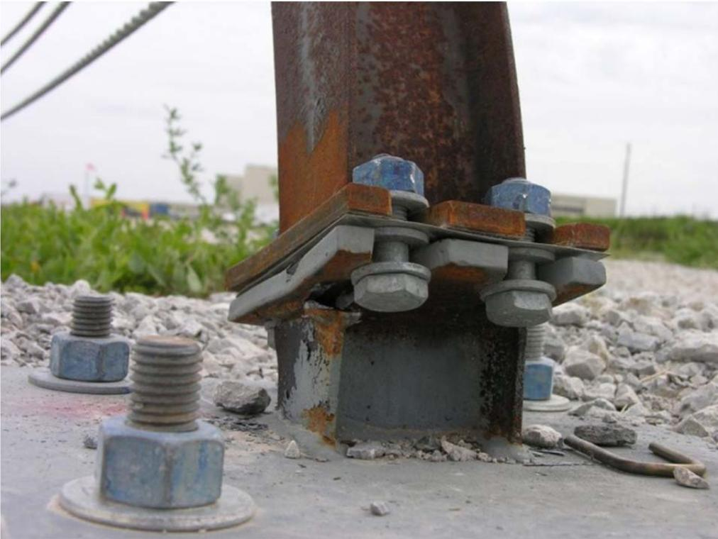
Figure 116. System Damage: Post No. 40, Test No. NYCC-3
