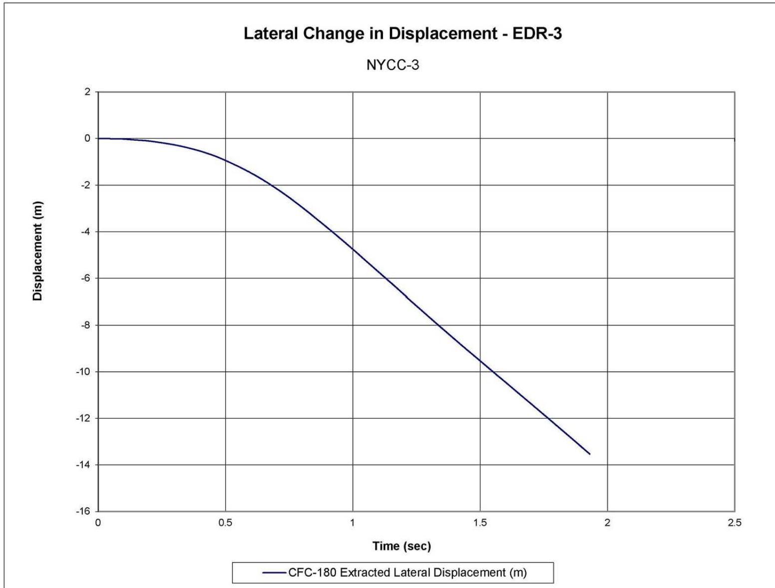
Figure G-22. Lateral Occupant Displacement (EDR-3), Test No. NYCC-3
