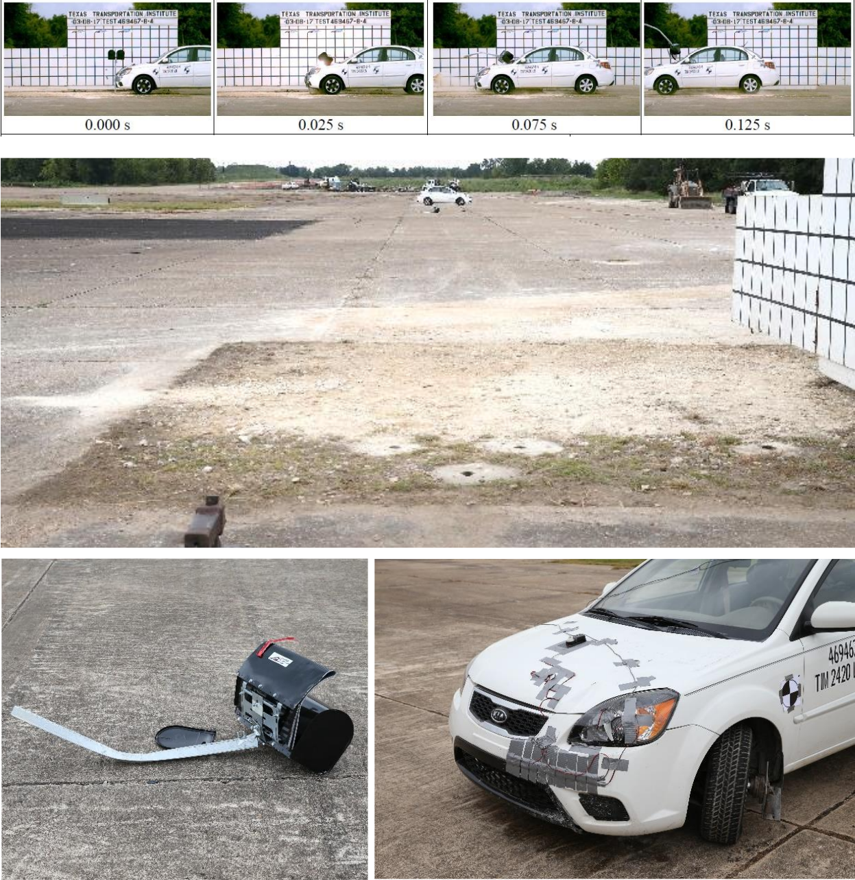
Figure 3. TxDOT Winged-Channel Mailbox Support - Test No. 469467-8-4, Test Results [5]
