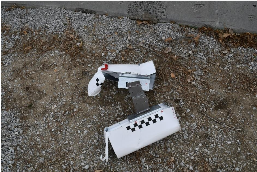
Figure 55. System Damage, Test No. NMB-1B
