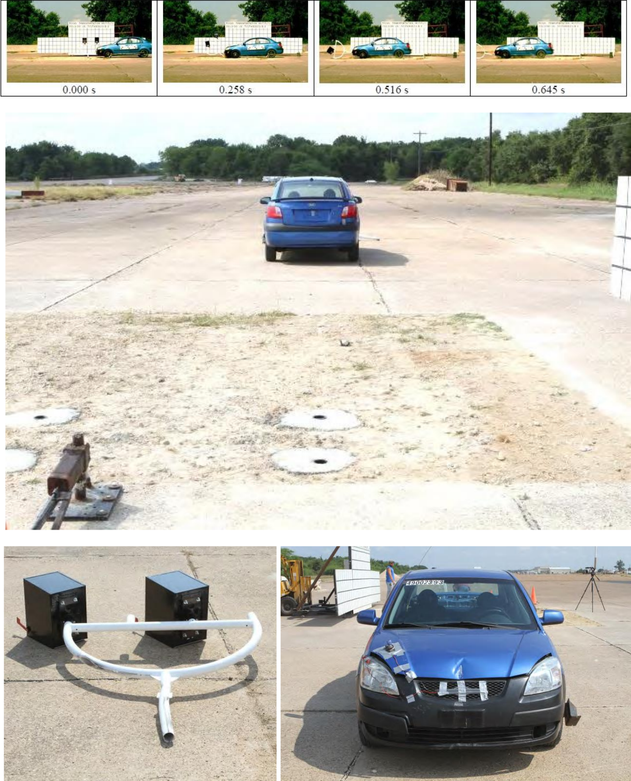
Figure 16. Locking Architectural Mailbox on Dual Mount Post - Test No. 490023-9-3, Test Results [7]
