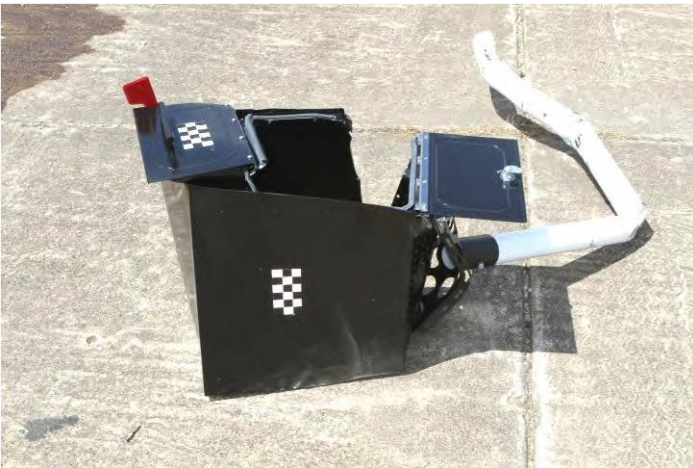
Figure 14. Locking Architectural Mailbox on Single Mount Post - Test No. 490023-9-2, Test Results [7]
