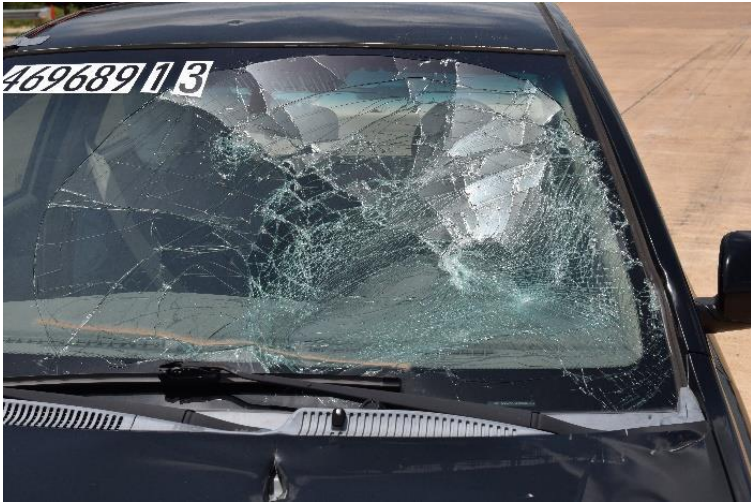
Figure 7. TxDOT Large Mailbox on Type 3 Support - Test No. 469689-1-3, Test Results [6]
