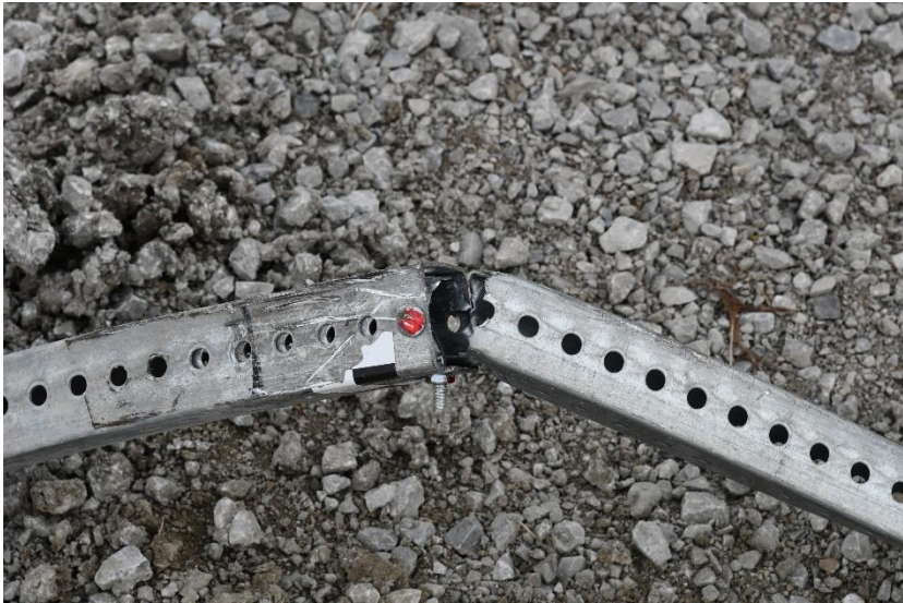
Figure 54. System Damage, Test No. NMB-1B
