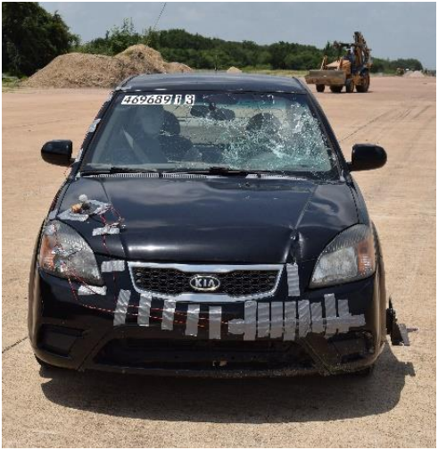
Figure 7. TxDOT Large Mailbox on Type 3 Support - Test No. 469689-1-3, Test Results [6]
