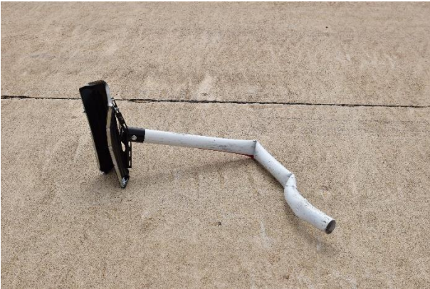
Figure 11. TxDOT Large Mailbox on Type 4 Support - Test No. 469689-1-1, Test Results [6]
