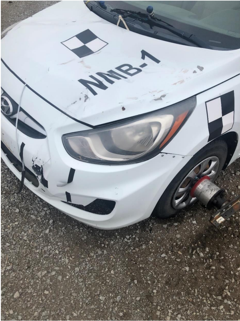
Figure 56. Vehicle Damage Test No. NMB-1
