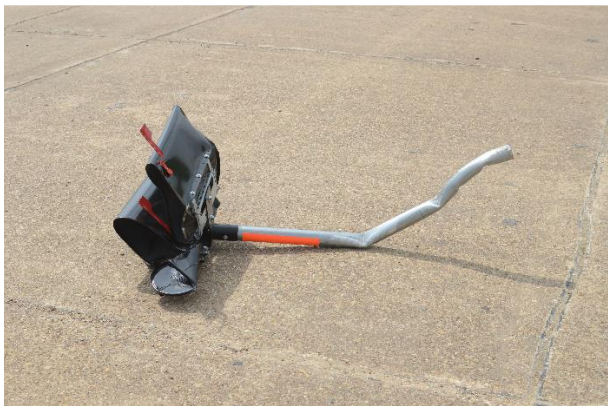
Figure 21. Double Mailbox with Thin-Wall Galvanized Support Post in Type 4 Foundation - Test No. 469468-8-2, Test Results [8]
