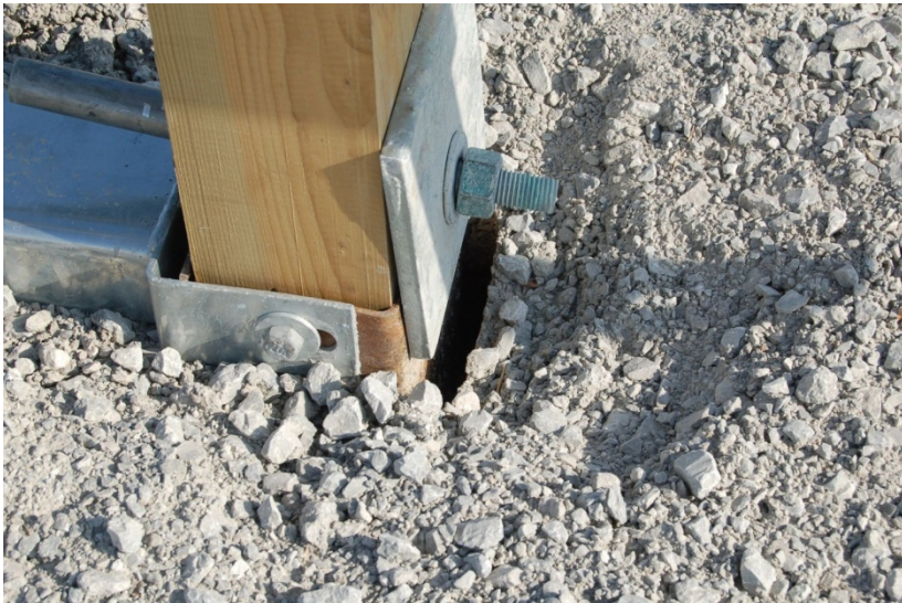
Figure 33. Anchorage Damage, Test No. MGSC-6
