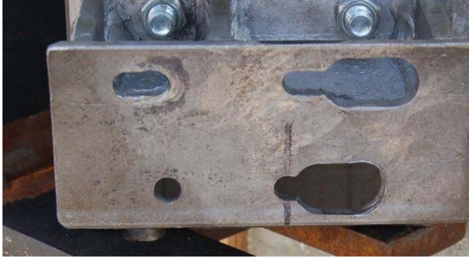
Figure 1. Slot and Keyway Designs (Top=Type 1, Bottom=Type 2)
