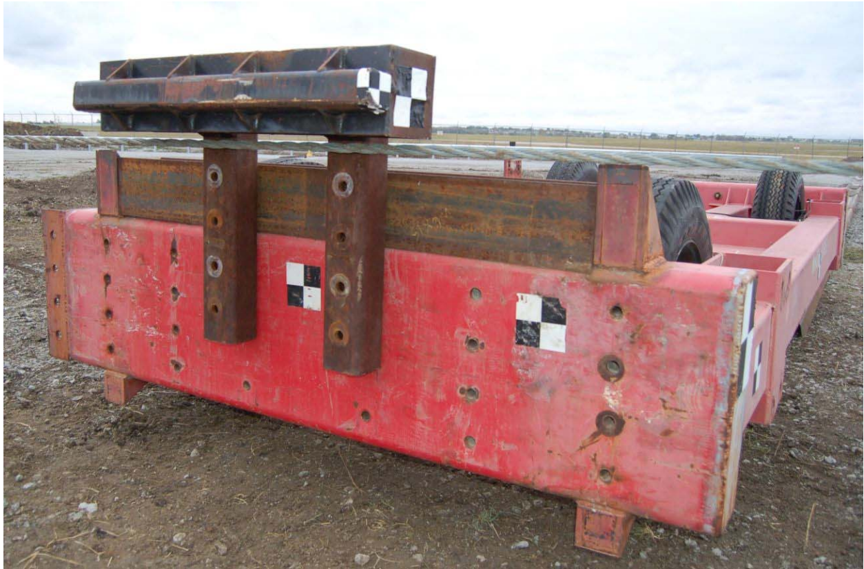
Figure 120. Rigid Frame Bogie with Head Attachment and Cable Height
