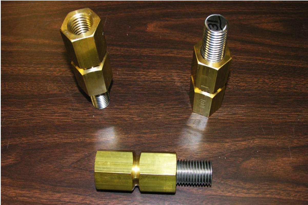
Figure 19. Brass Couplings (Version 1), Test Nos, BBC-1 and BBC-2
