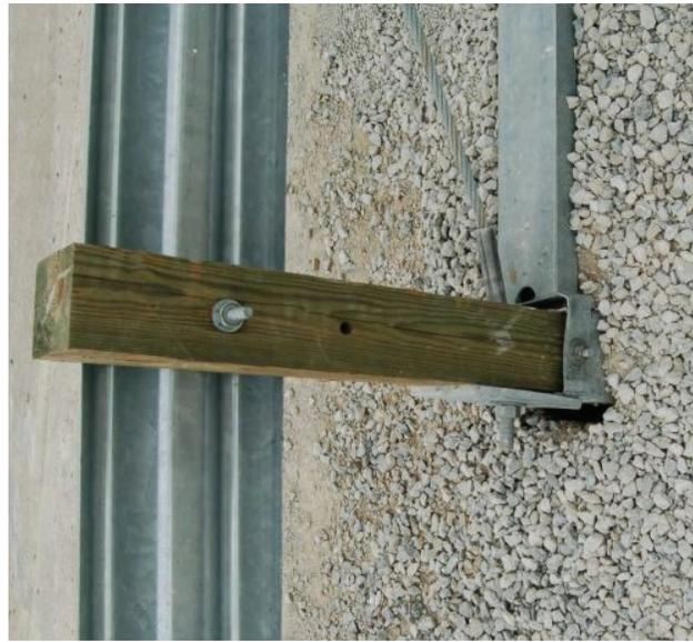
Figure 71. Upstream Anchorage Damage, Test No. MWTSF-2
