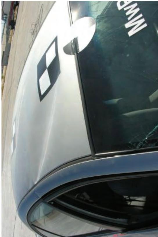
Figure 91. Occupant Compartment Deformation and Windshield Damage, Test No. MWTSP-3
