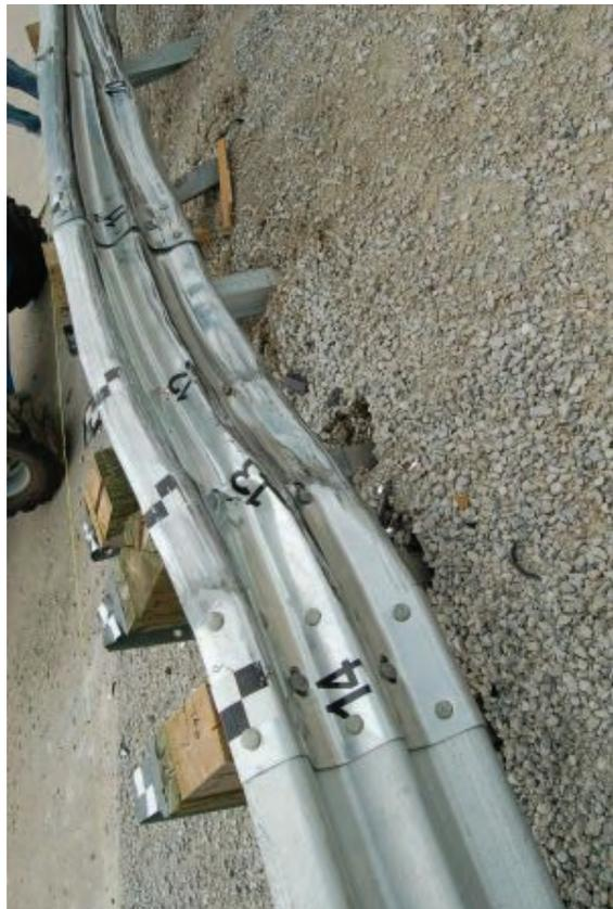
Figure 74. Post Nos. 12 through 14 Damage, Test No. MWTSP-2
