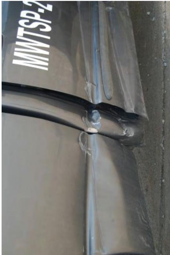
Figure 77. Vehicle Damage, Test No. MWTSP-2
