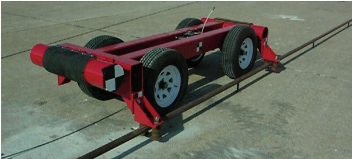
Figure 2. Rigid Frame Bogie on Guidance Track
