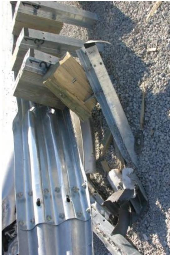
Figure 88. Post Nos. 12 through 14 Damage, Test No. MWTSP-3
