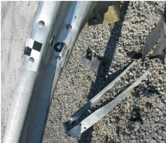
Figure 86. Posts Nos. 7 through 9 Damage, Test No. MWTSP-3
