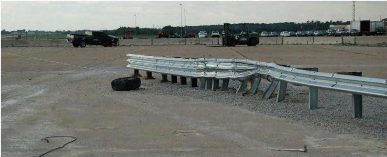
Figure 69. Vehicle Trajectory and Final Position, Test No. MWTSP-2
