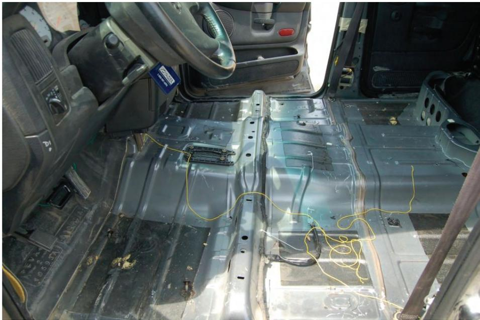
Figure 78. Occupant Compartment Damage, Test No. MWTSP-2
