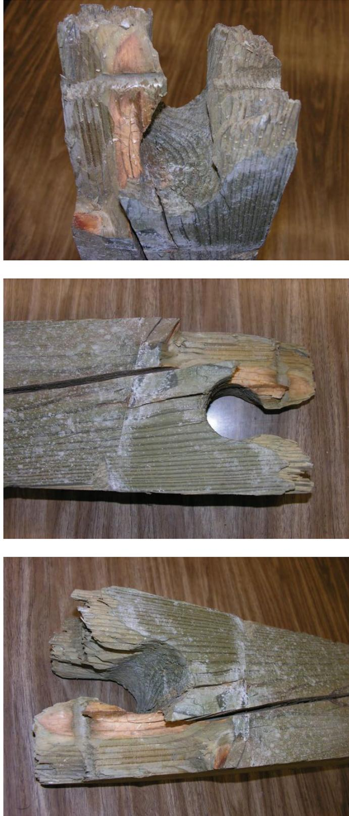
Figure 61. Anchorage Post No. 1 Damage, Test No. MWTSP-1
