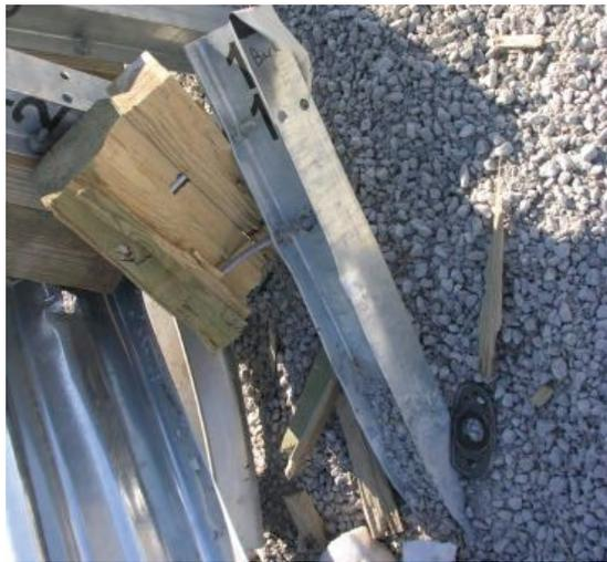
Figure 87. Posts Nos. 10 and 11 Damage, Test No. MWTSP-3
