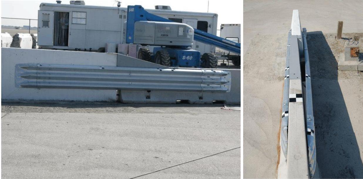
Figure 3. Temporary Concrete Barrier to Permanent Concrete Barrier Transition, Test Nos. TCBT-1 and TCBT-2 [11]
