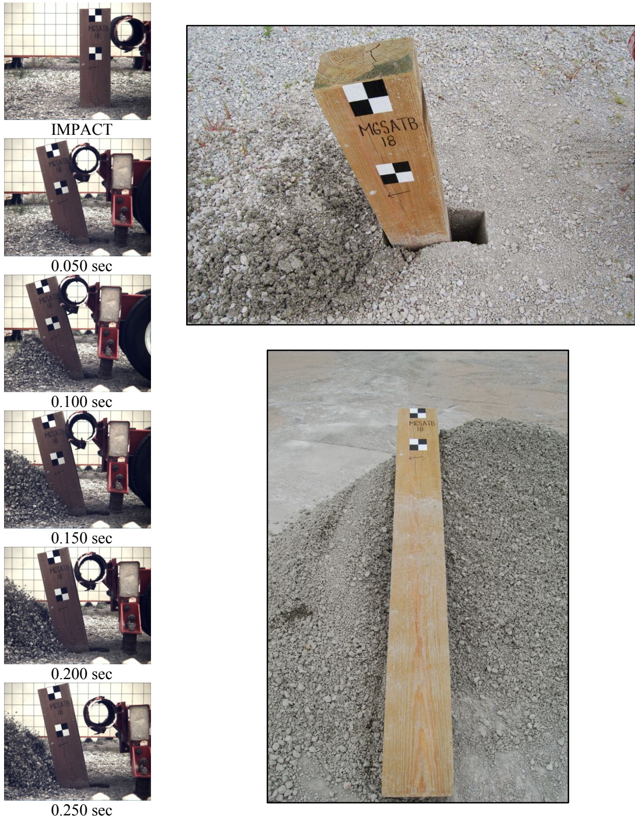
Figure 40. Time Sequential and Post-Impact Photographs, Test No. MGSATB-18
