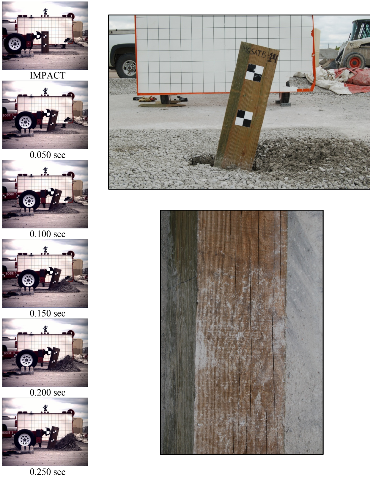
Figure 32. Time Sequential and Post-Impact Photographs, Test No. MGSATB-14
