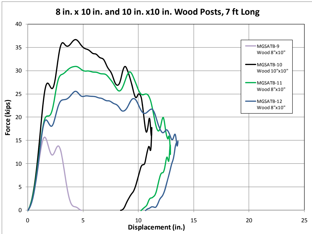
Figure 47. Force vs. Deflection Comparison, 7-ft (2.1-m) 8-in. x 10-in (203-mm x 254-mm). and 10-in. x 10-in. (254-mm x 254-mm) Wood Posts
