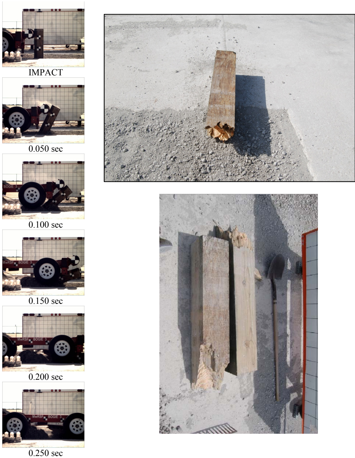
Figure 22. Time Sequential and Post-Impact Photographs, Test No. MGSATB-9
