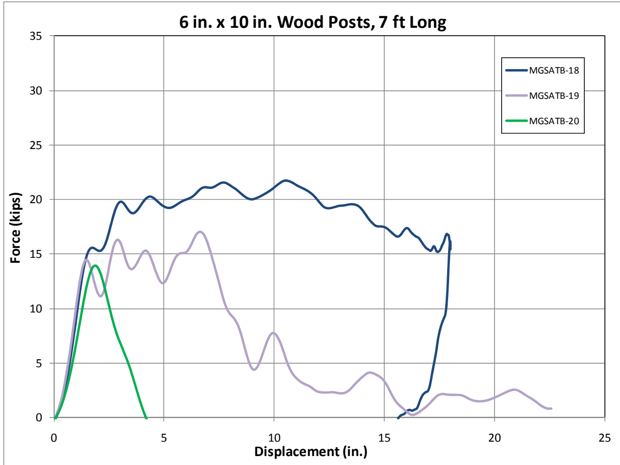
Figure 48. Force vs. Deflection Comparison, 7-ft (2.1-m) Long 6-in. x 10-in. (152-mm x 254-mm) Wood Posts
