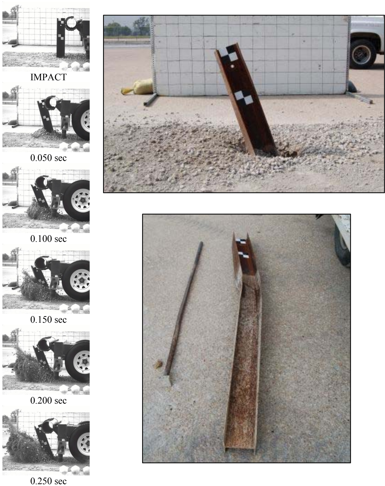
Figure 6. Time Sequential and Post-Impact Photographs, Test No. MGSATB-1
