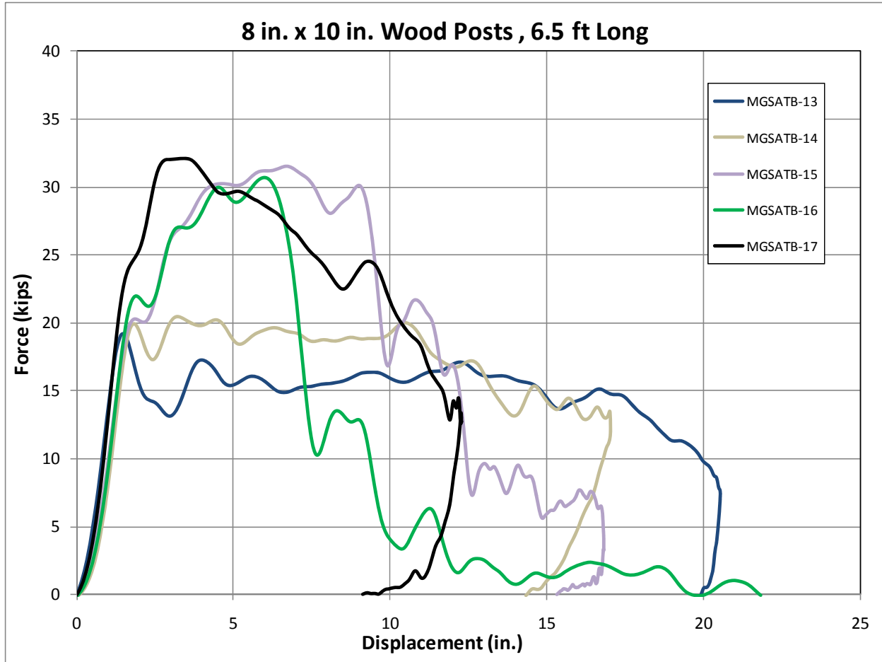
Figure 49. Force vs. Deflection Comparison, 6.5-ft (2.0-m) Long 8-in. x 10-in. (203-mm x 254-mm) Wood Posts
