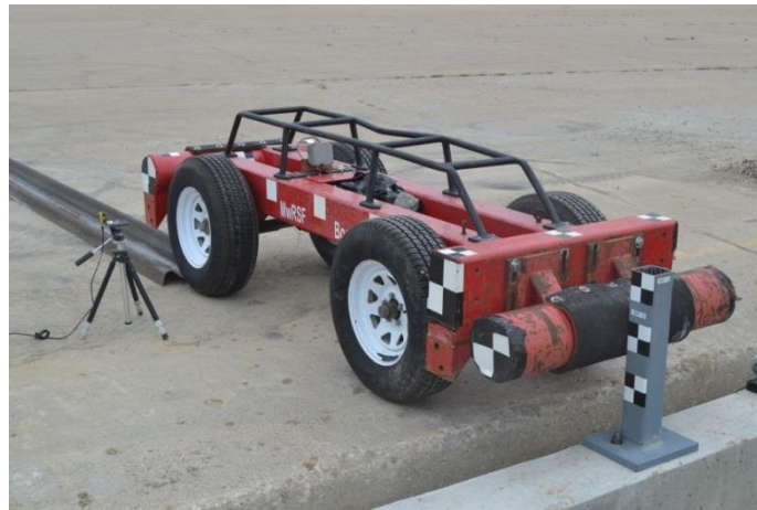
Figure 35. Rigid-Frame Bogie on Guidance Track
