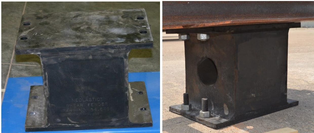
Figure 3. 11 \frac{5}{8} -in. (295-mm) Tall Shear Fender
