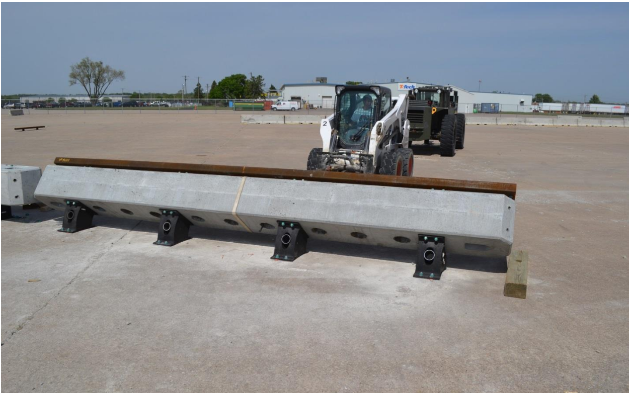
Figure 68. Barrier Deflection with Steel Pipe Inserts
