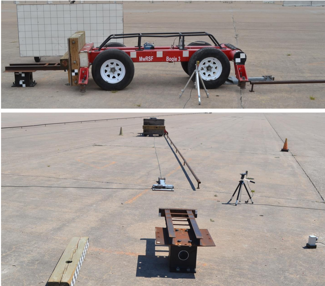
Figure 23. Rigid-Frame Bogie on Guidance Track
