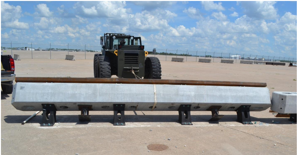
Figure 71. Maximum Barrier Deflection with Two Support Skids with Shims
