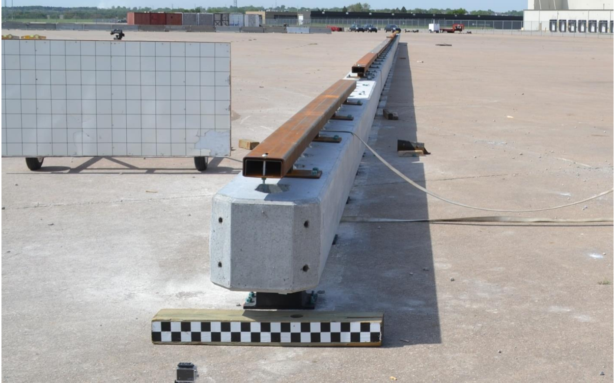
Figure 67. Barrier Stability with Steel Pipe Inserts
