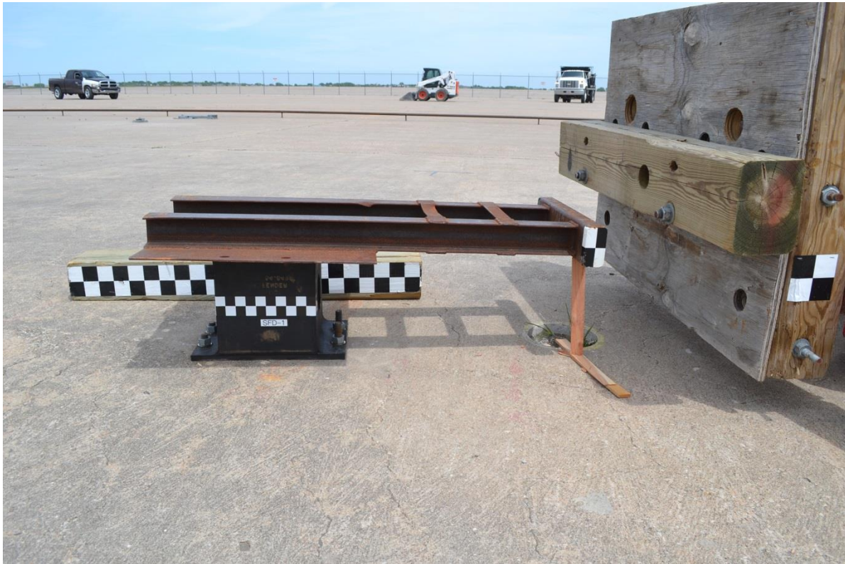
Figure 4. Bogie Test Setup, All Tests
