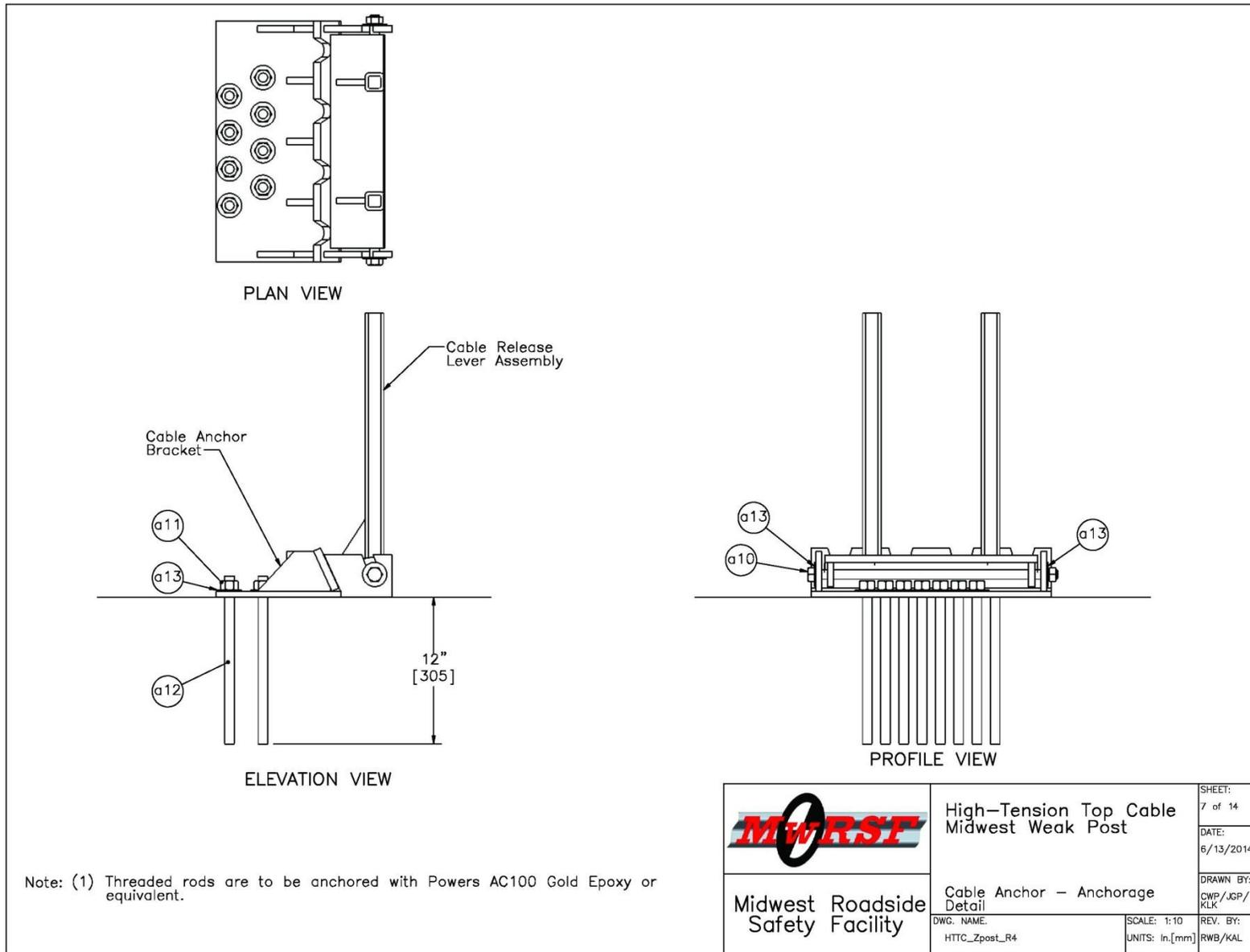
Figure 90. Cable Anchor - Anchorage Detail, Test No. HTTC-2
