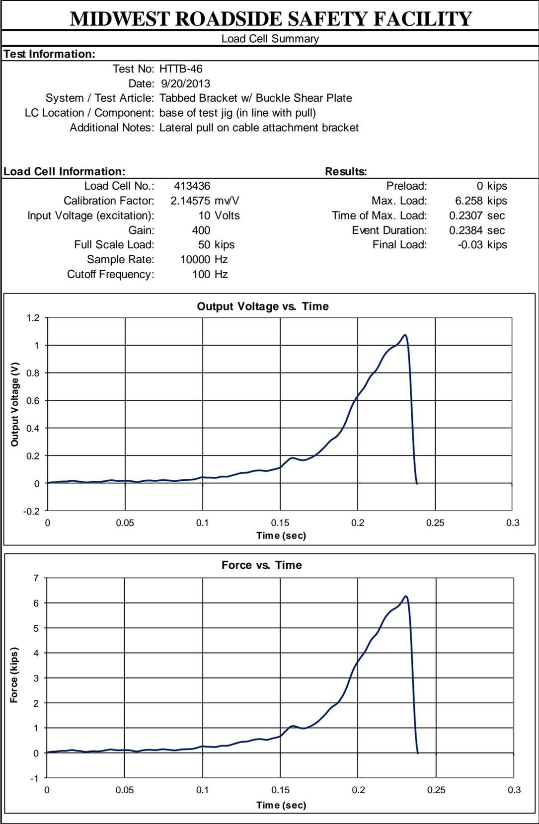
Figure B-6. Load Cell Results, Test No. HTTP-46
