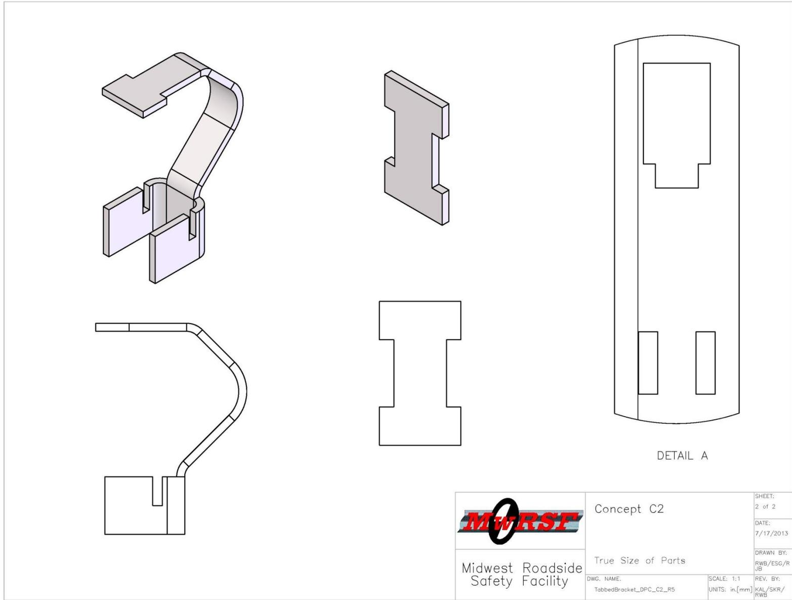
Figure 32. Concept C2, Drop-In Shear Plate, Continued
