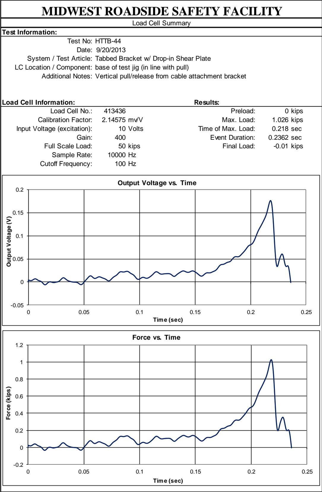
Figure B-4. Load Cell Results, Test No. HTTP-44
