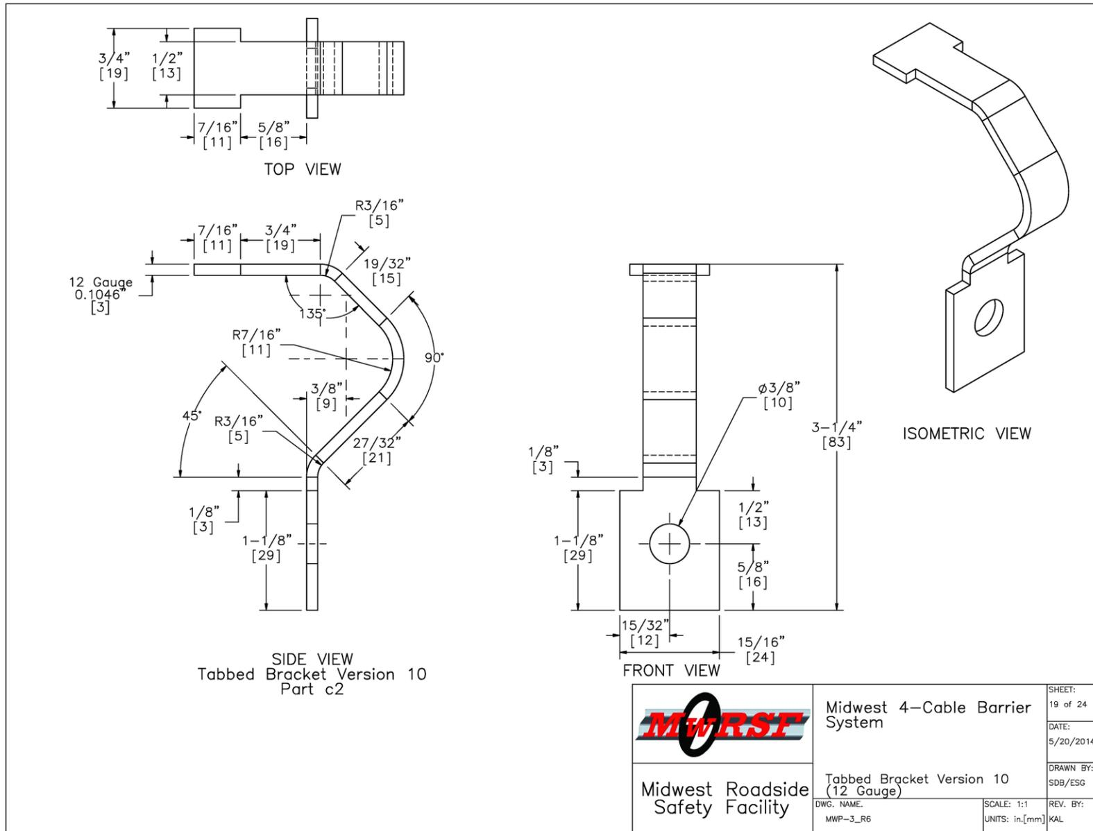
Figure 2. Bolted Tabbed Bracket V-10, Design Details
