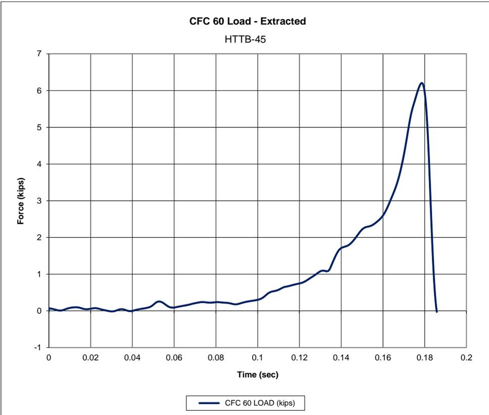
Figure 67. Force vs. Time Data, Test No. HTTPB-45
