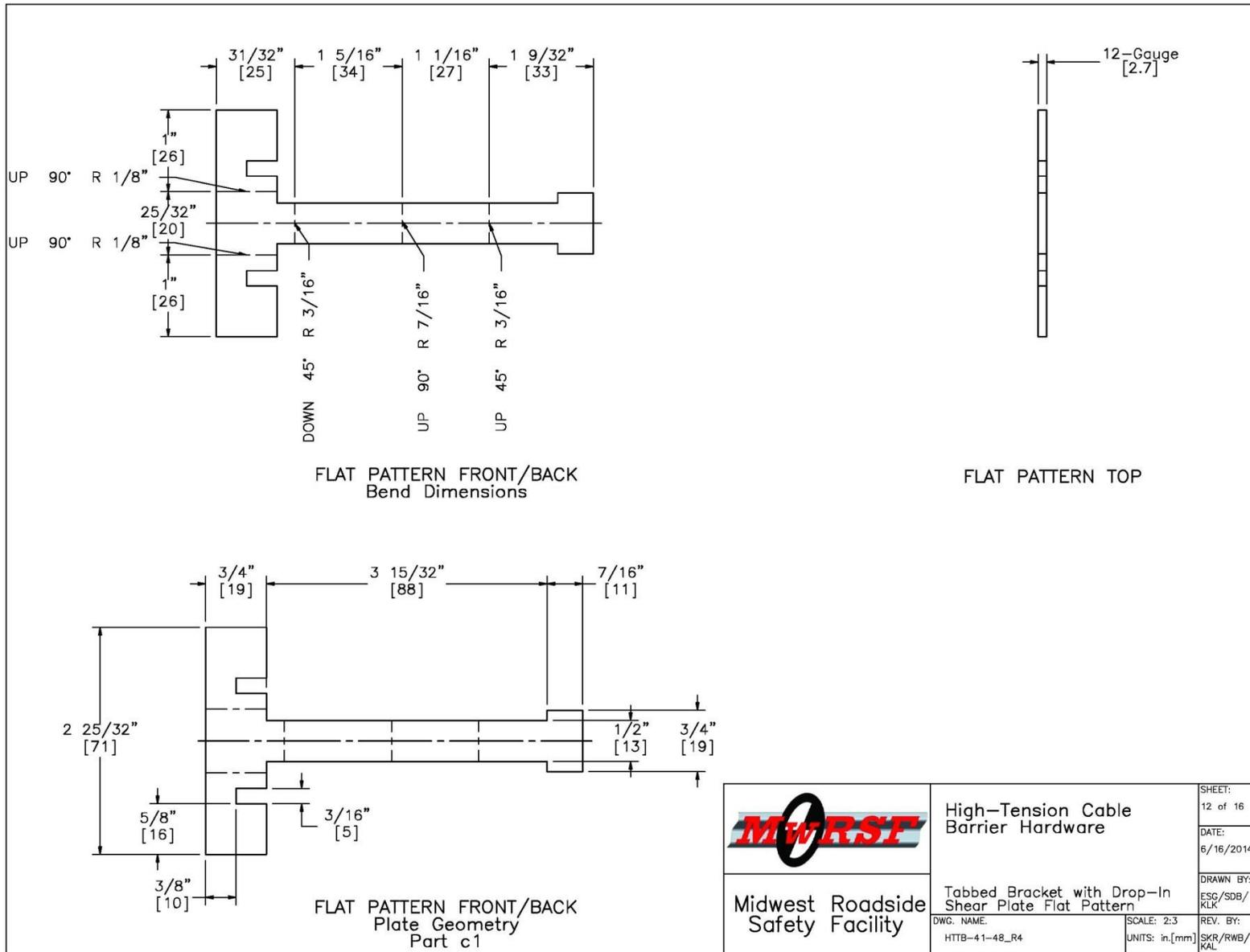
Figure 48. Tabbed Bracket with Drop-In Shear Plate Flat Pattern, Test Nos. HTTB-43, HTTB-44, HTTB-47, and HTTB-48
