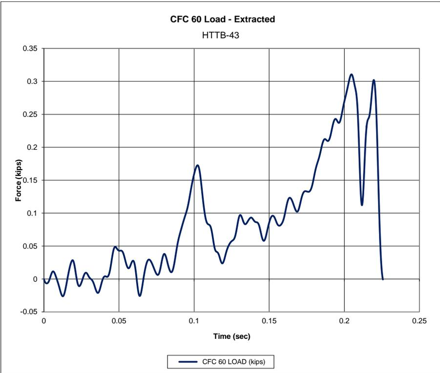
Figure 61. Force vs. Time Data, Test No. HTTPB-43
