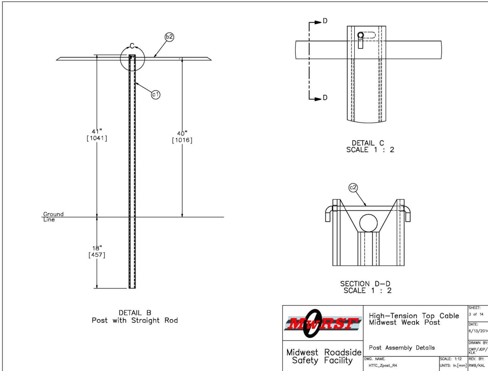
Figure 86. Post Assembly Details, Test No. HTTC-2
