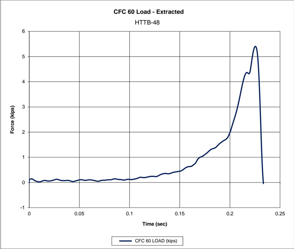
Figure 76. Force vs. Time Data, Test No. HTTB-48
