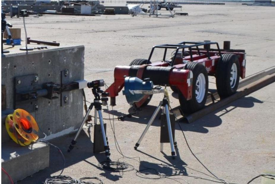
Figure 53. Rigid-Frame Bogie on Guidance Track
