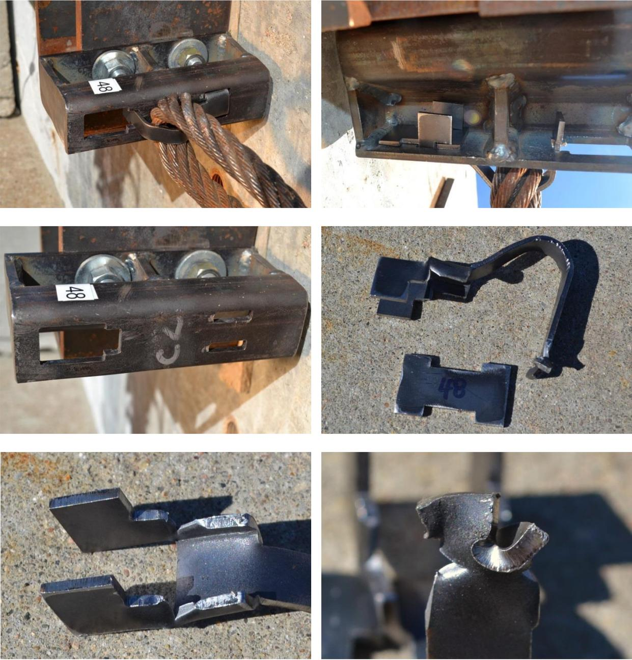
Figure 77. Pre-Test (Top Two) and Post-Test (Bottom Four) Photographs, Test No. HTTP-48
