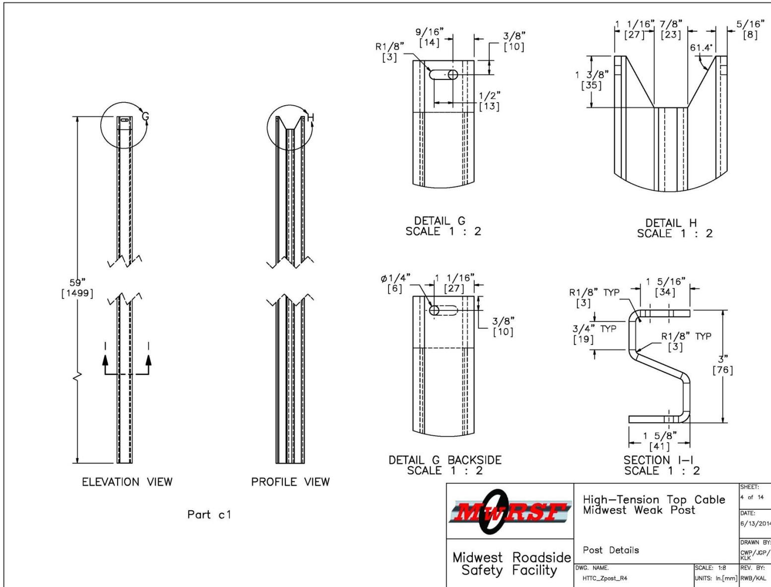
Figure 87. Midwest Weak Post Details, Test No. HTTC-2
