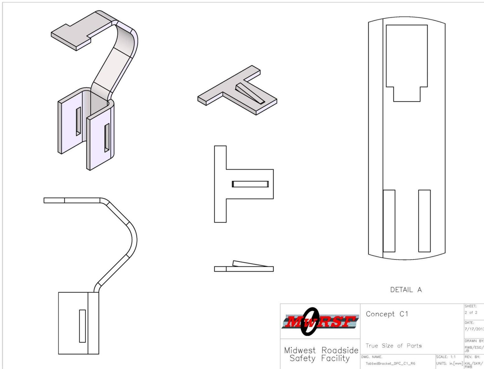
Figure 30. Concept C1, Lateral Shear Plate, Continued
