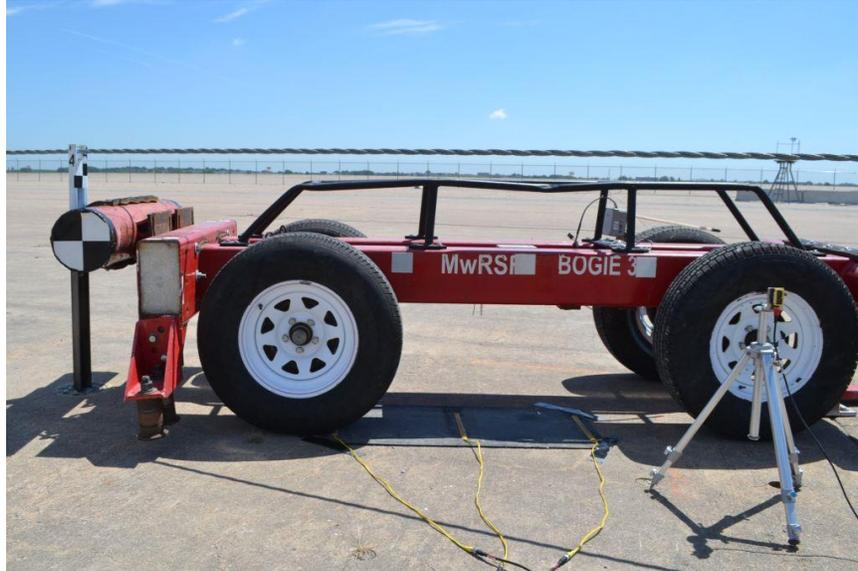
Figure 99. Rigid-Frame Bogie on Guidance Track
