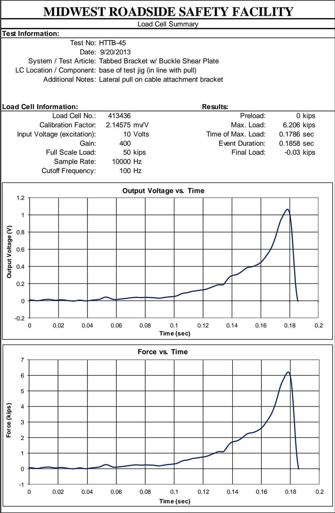
Figure B-5. Load Cell Results, Test No. HTTB-45
