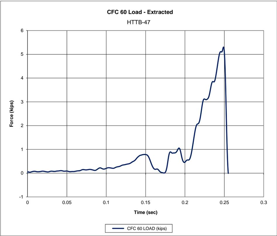
Figure 73. Force vs. Time Data, Test No. HTTPB-47
