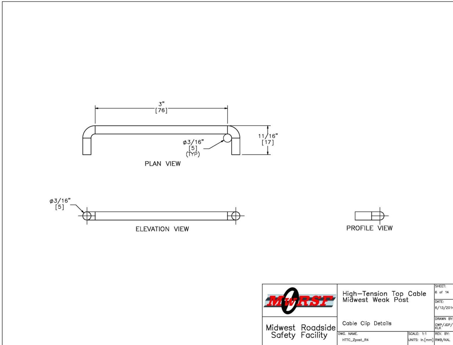
Figure 89. Cable Clip Details, Test No. HTTC-2
