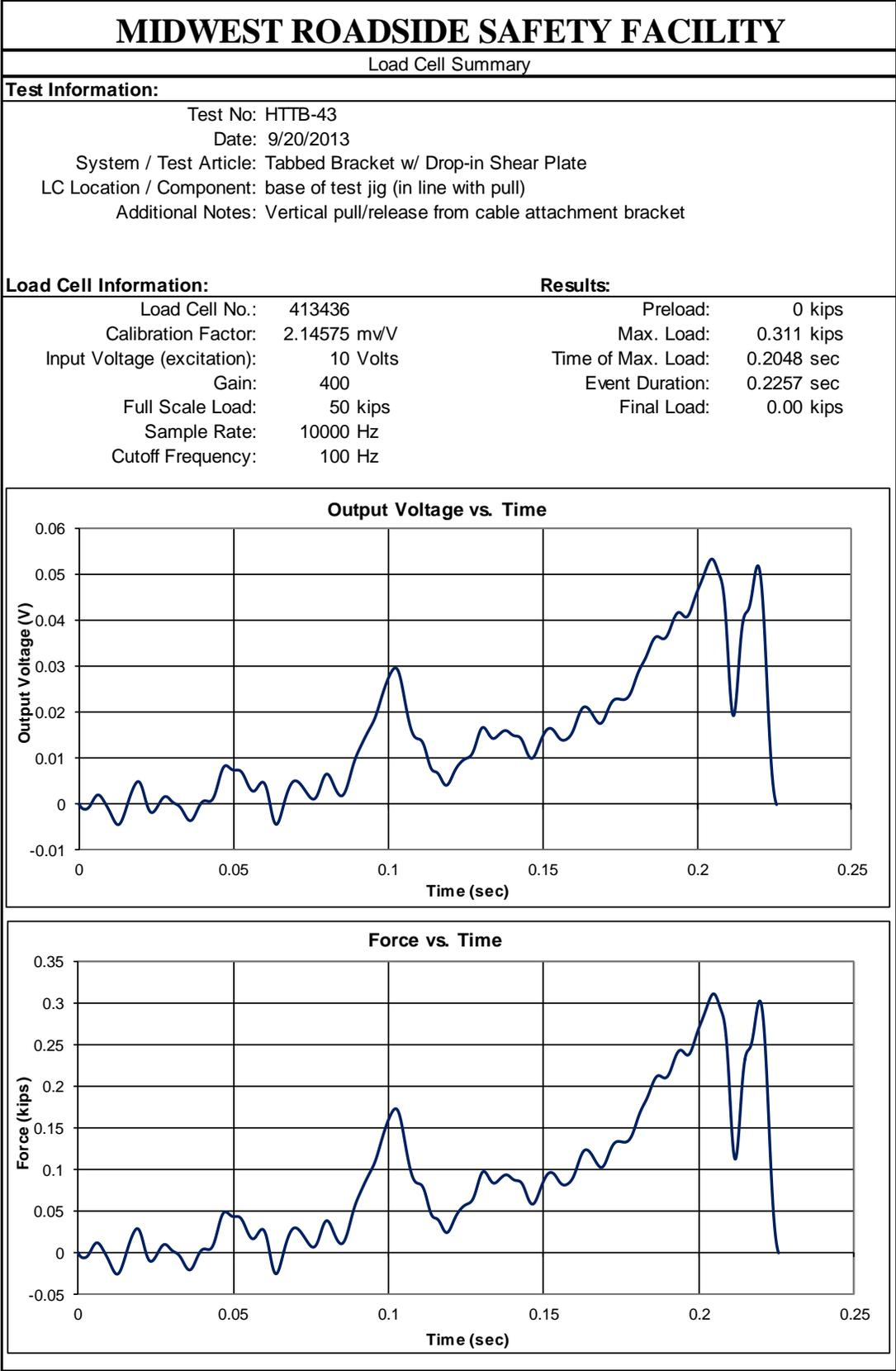
Figure B-3. Load Cell Results, Test No. HTTB-43
