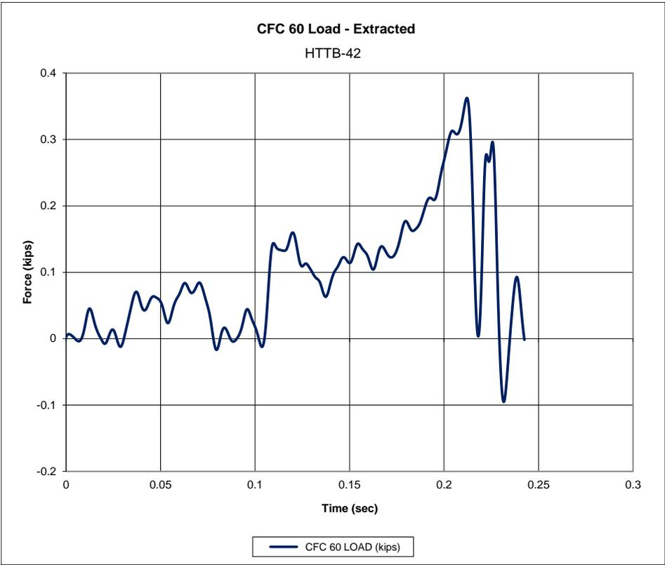
Figure 58. Force vs. Time Data, Test No. HTTPB-42
