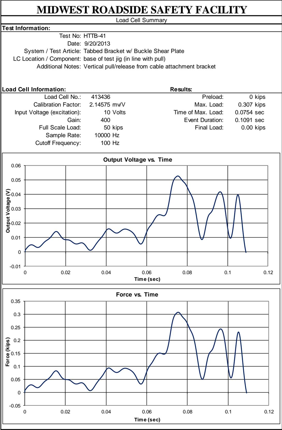
Figure B-1. Load Cell Results, Test No. HTTP-41
