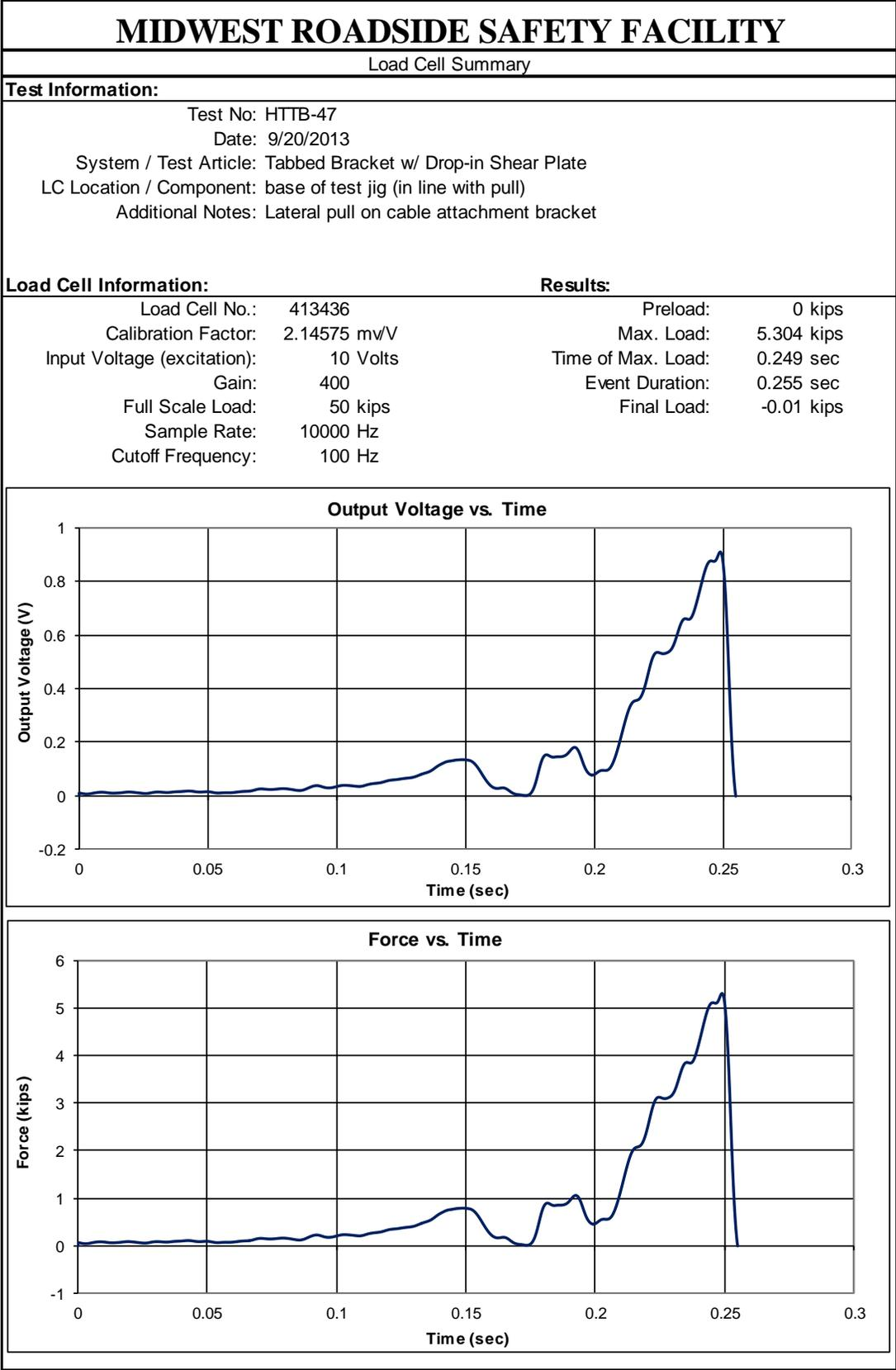
Figure B-7. Load Cell Results, Test No. HTTP-47
