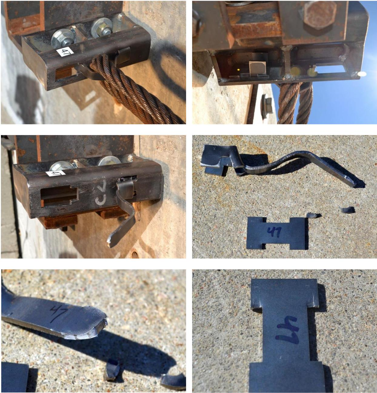
Figure 74. Pre-Test (Upper) and Post-Test (Lower) Photographs, Test No. HTTB-47
