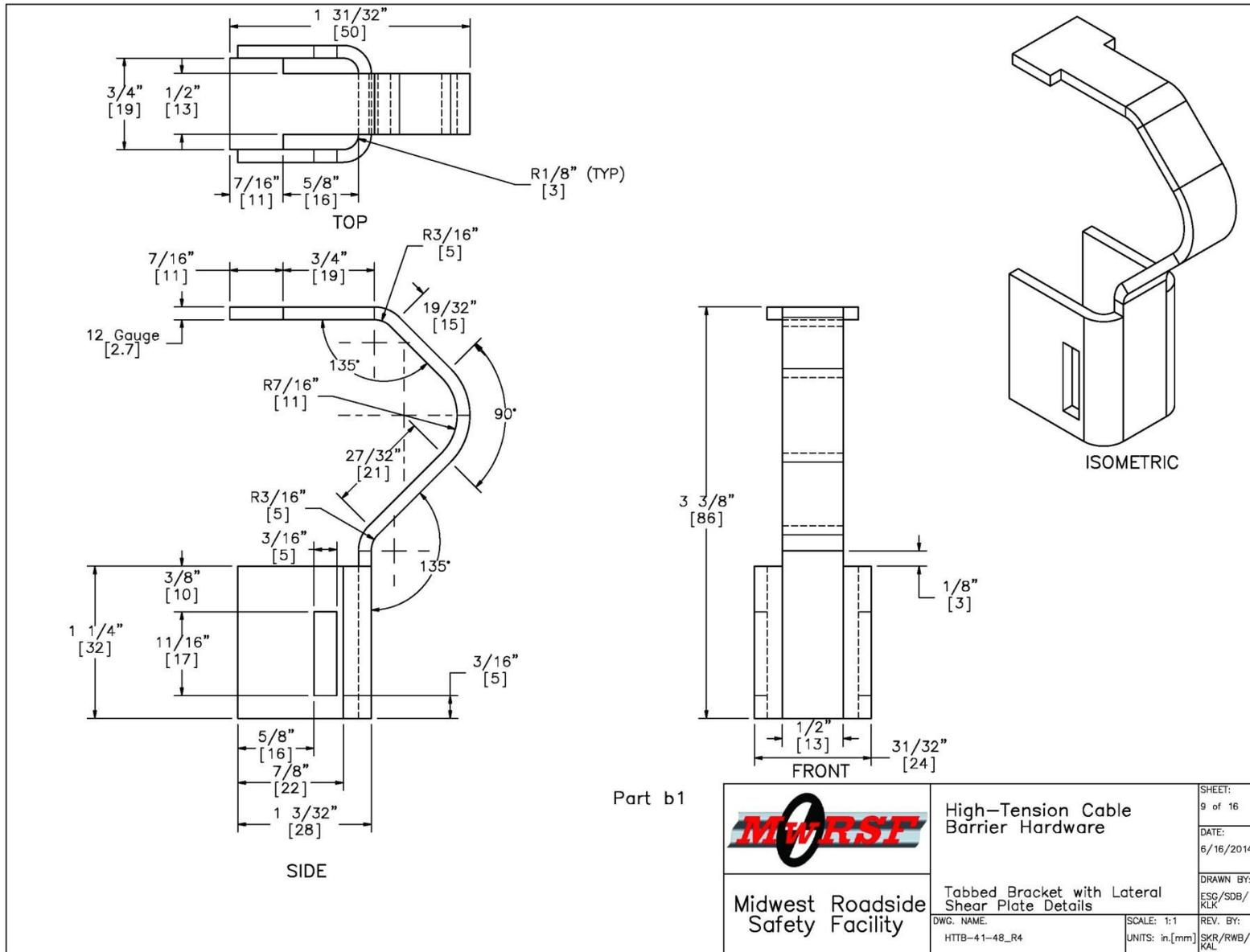
Figure 45. Tabbed Bracket with Lateral Shear Plate Details, Test Nos. HTTP-41, HTTP-42, HTTP-45, and HTTP-46
