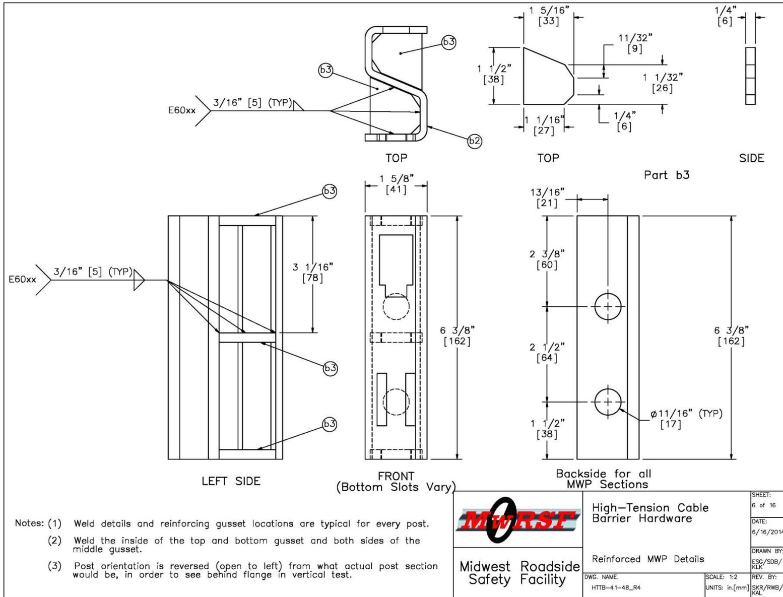
Figure 42. Reinforced MWP Details, Test Nos. HTTB-41 through HTTB-48
