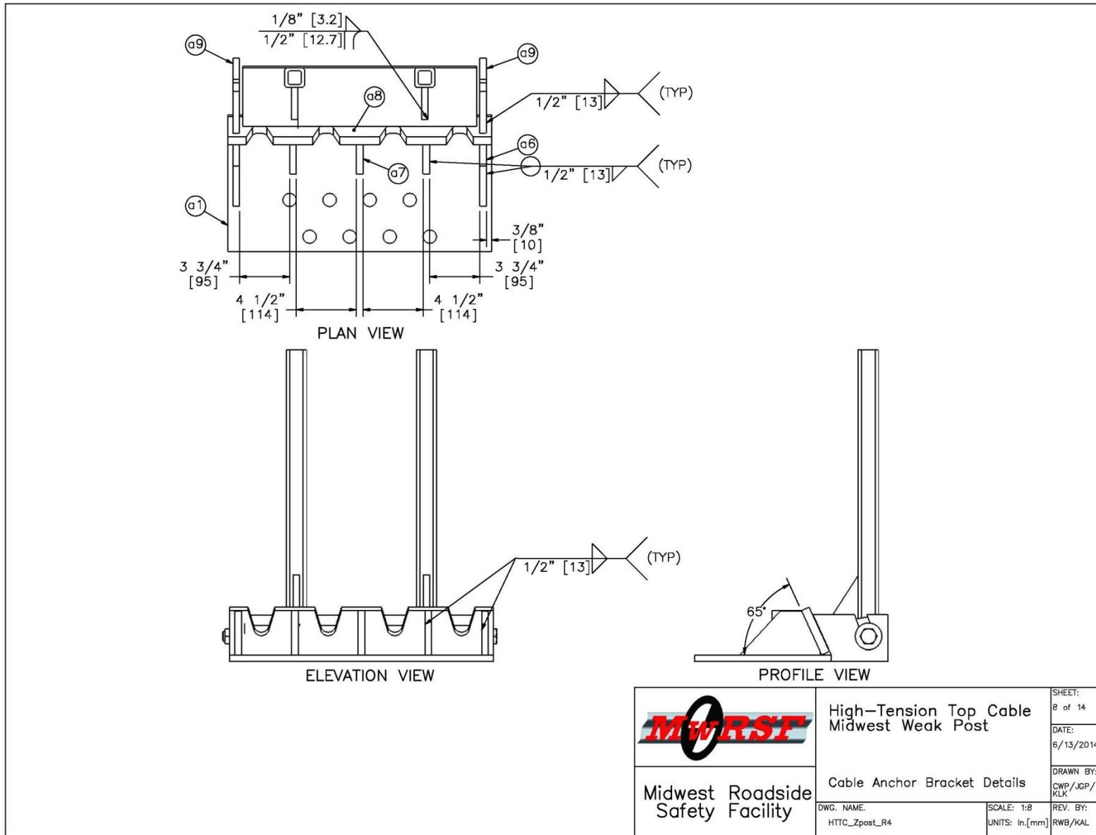
Figure 91. Cable Anchor Bracket Details, Test No. HTTC-2
