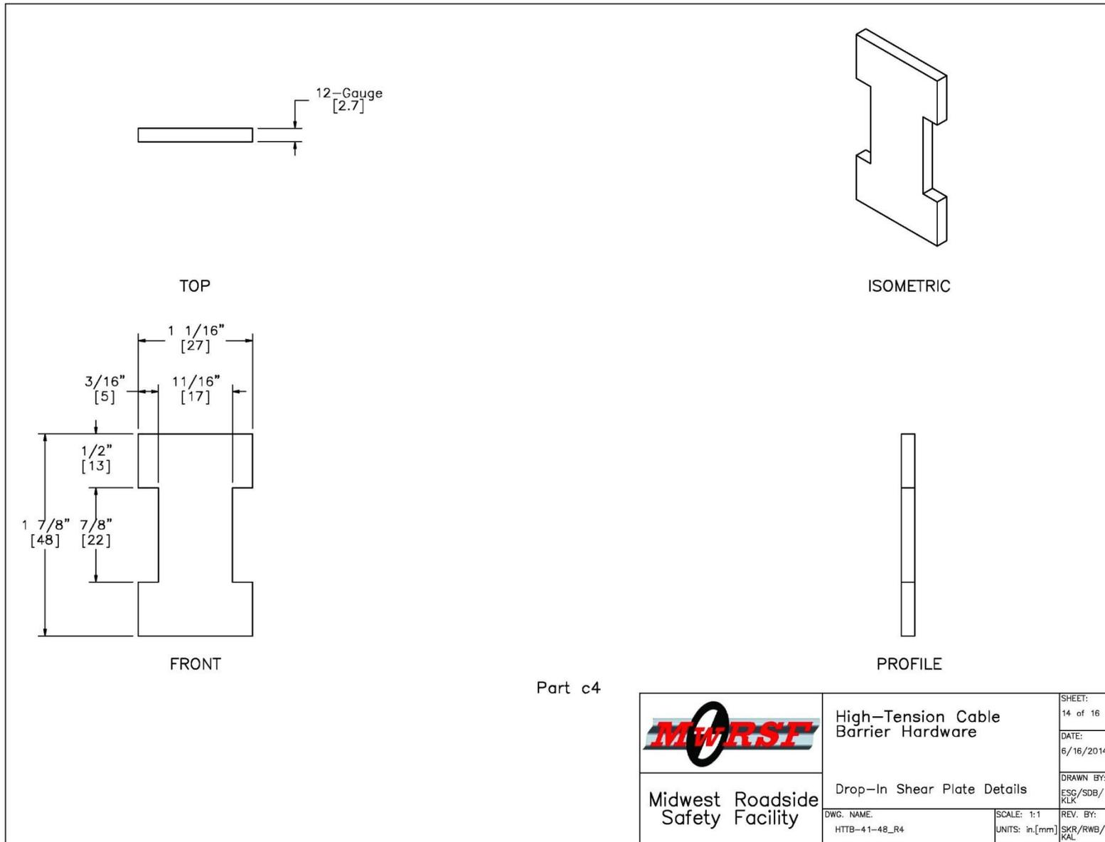
Figure 50. Drop-In Shear Plate Details, Test Nos. HTTB-43, HTTB-44, HTTB-47, and HTTB-48
