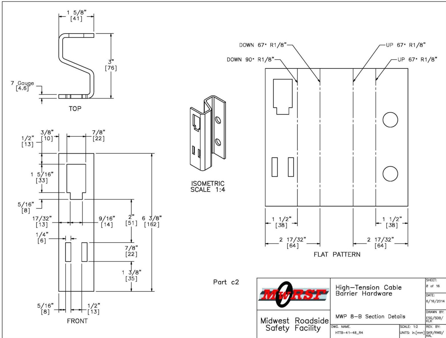
Figure 44. MWP 8-B Section Details, Test Nos. HTTP-43, HTTP-44, HTTP-47, and HTTP-48
