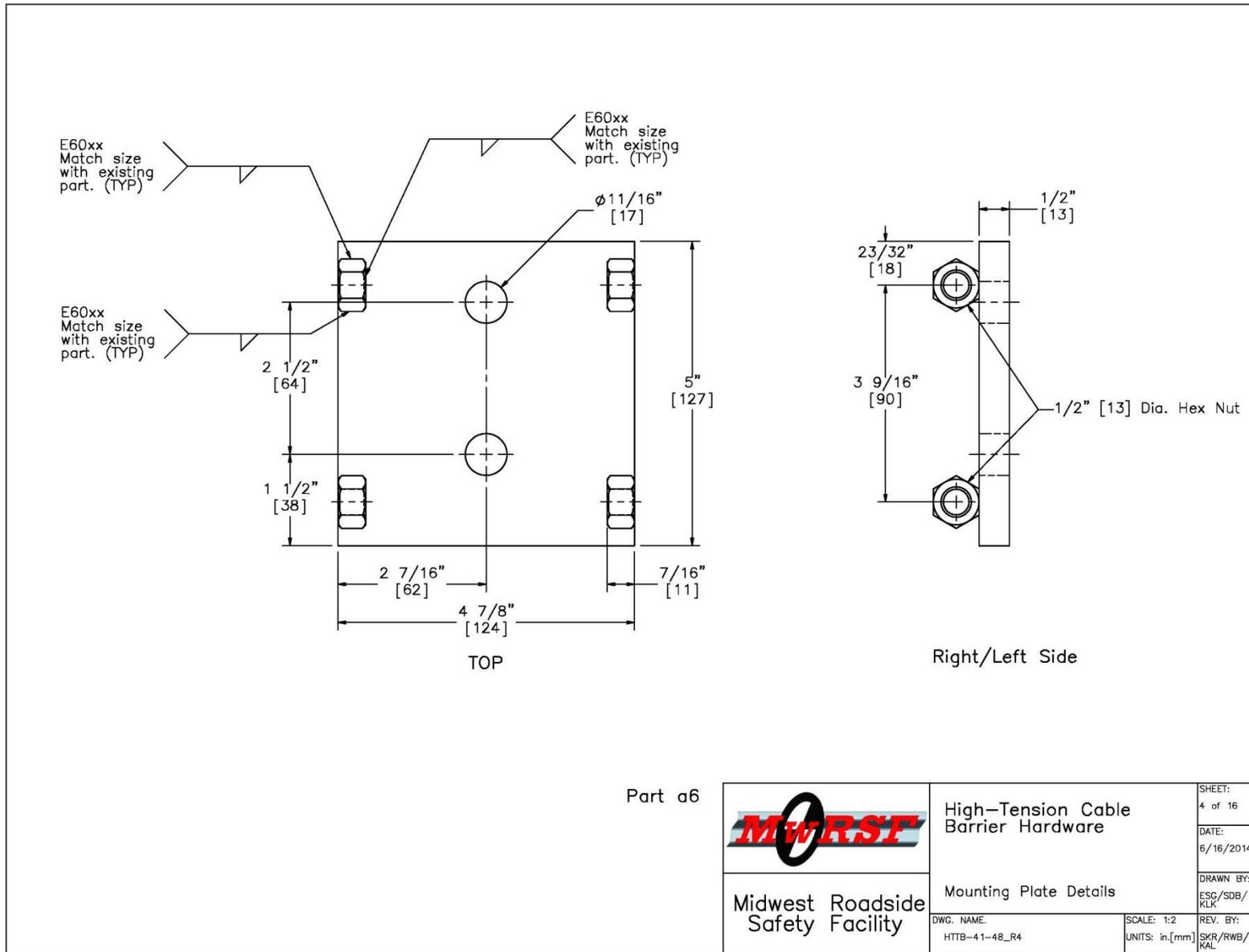
Figure 40. Mounting Plate Details, Test Nos. HTTB-41 through HTTB-48
