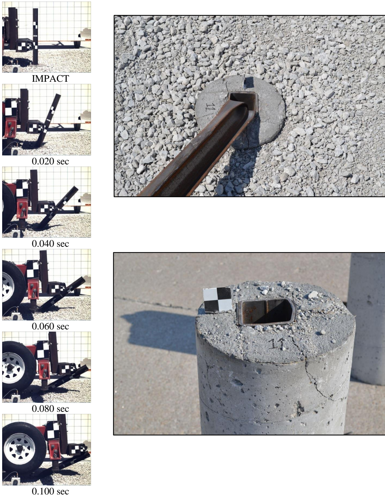
Figure 37. Time-Sequential and Post-Impact Photographs, Test No. HTCB-11
