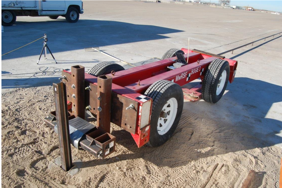
Figure 1. Rigid-Frame Bogie on Guidance Track
