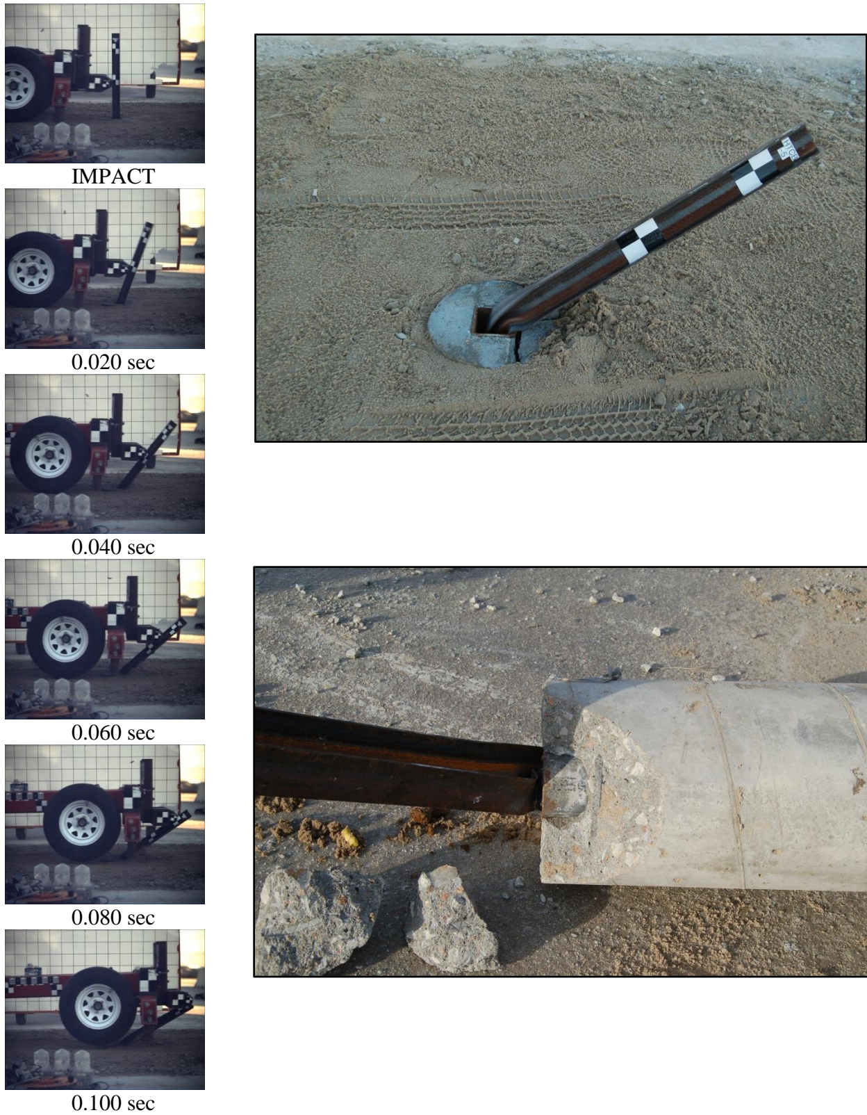
Figure 12. Time-Sequential and Post-Impact Photographs, Test No. HTCB-5
