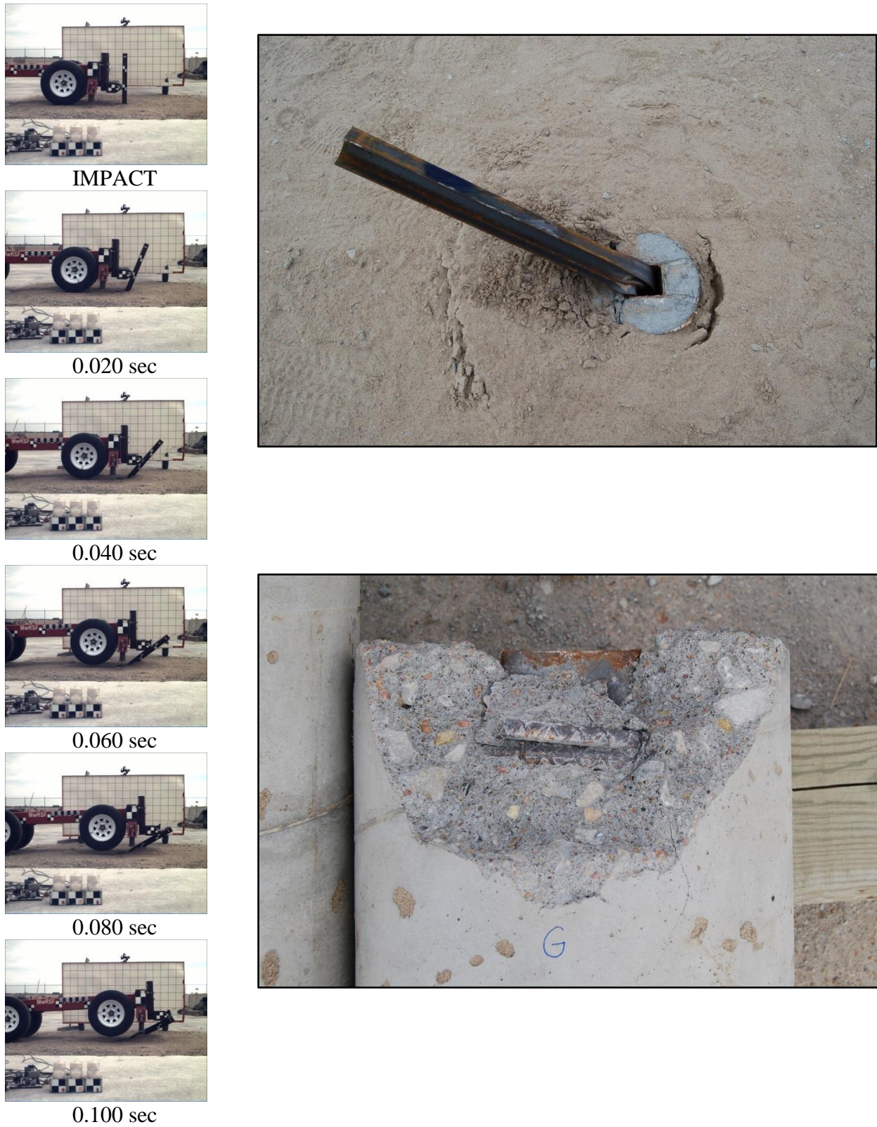
Figure 20. Time-Sequential and Post-Impact Photographs, Test No. HTCB-9
