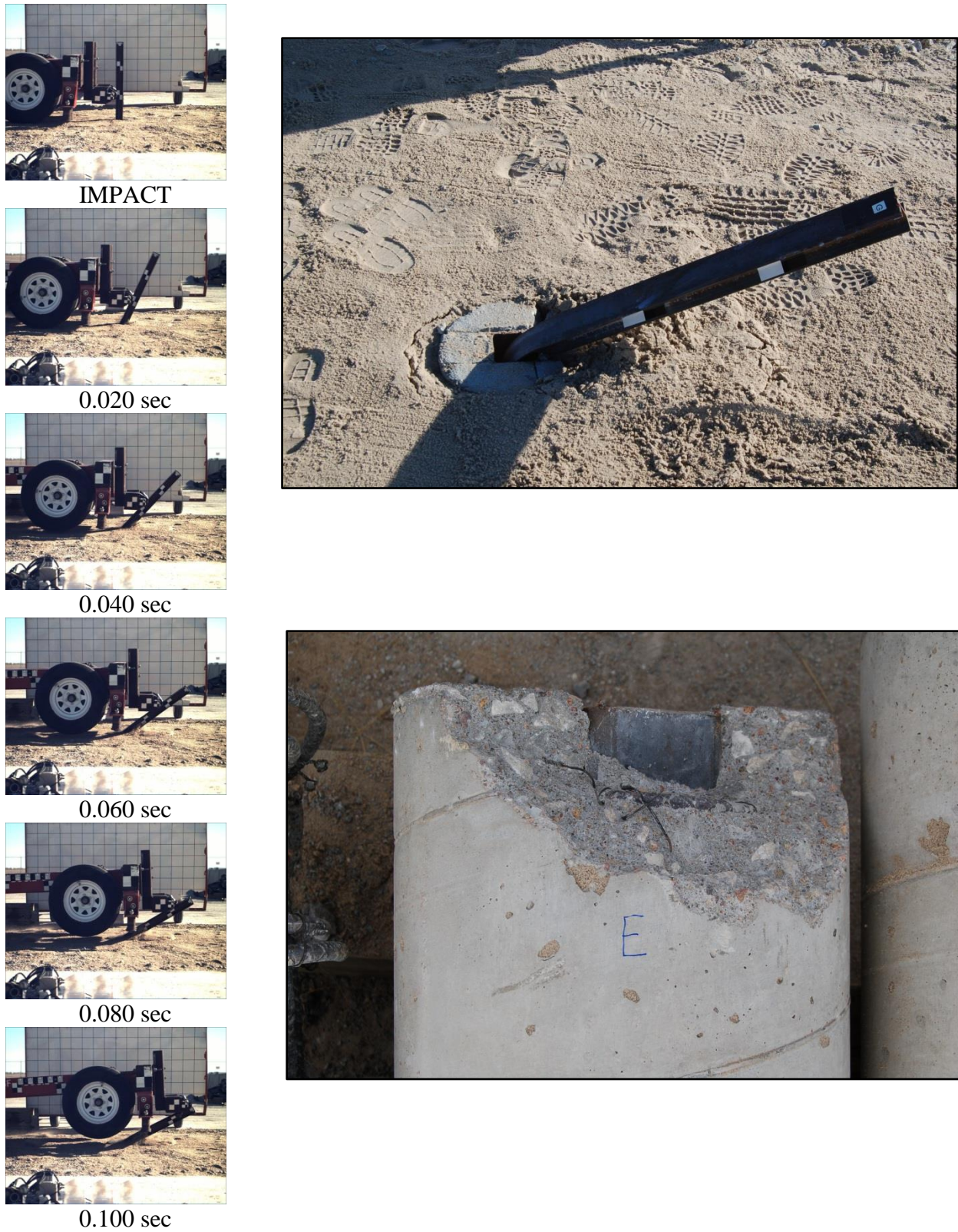
Figure 16. Time-Sequential and Post-Impact Photographs, Test No. HTCB-7
