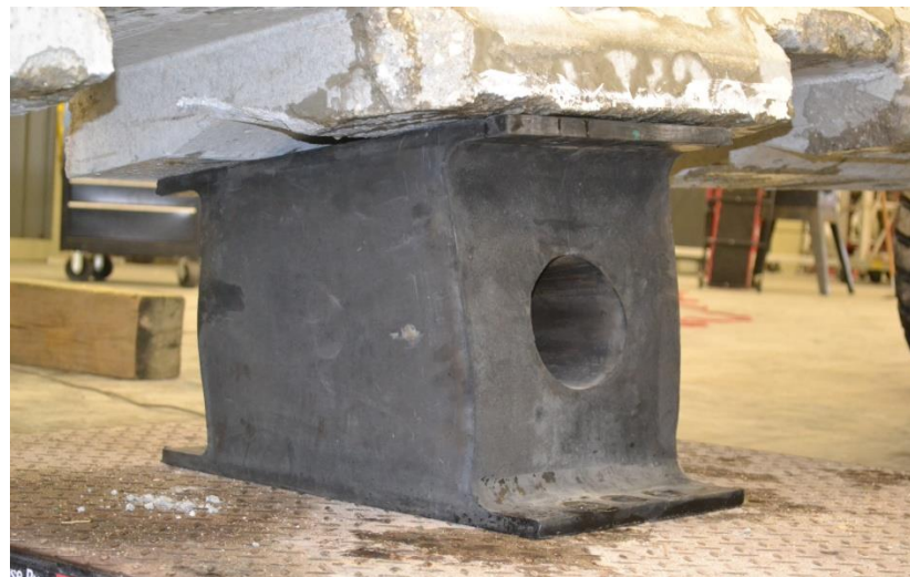
Figure 92. Example of System Instabilities, Test Nos. SFHS-1 through SFHS-3
