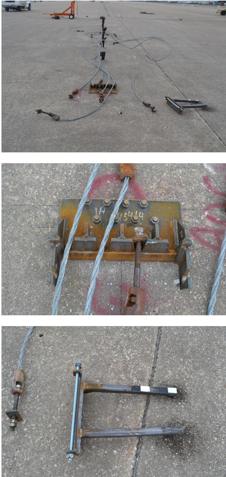
Figure 30. System Damage – Downstream Cable Anchor Bracket, Test No. HTCT-2
