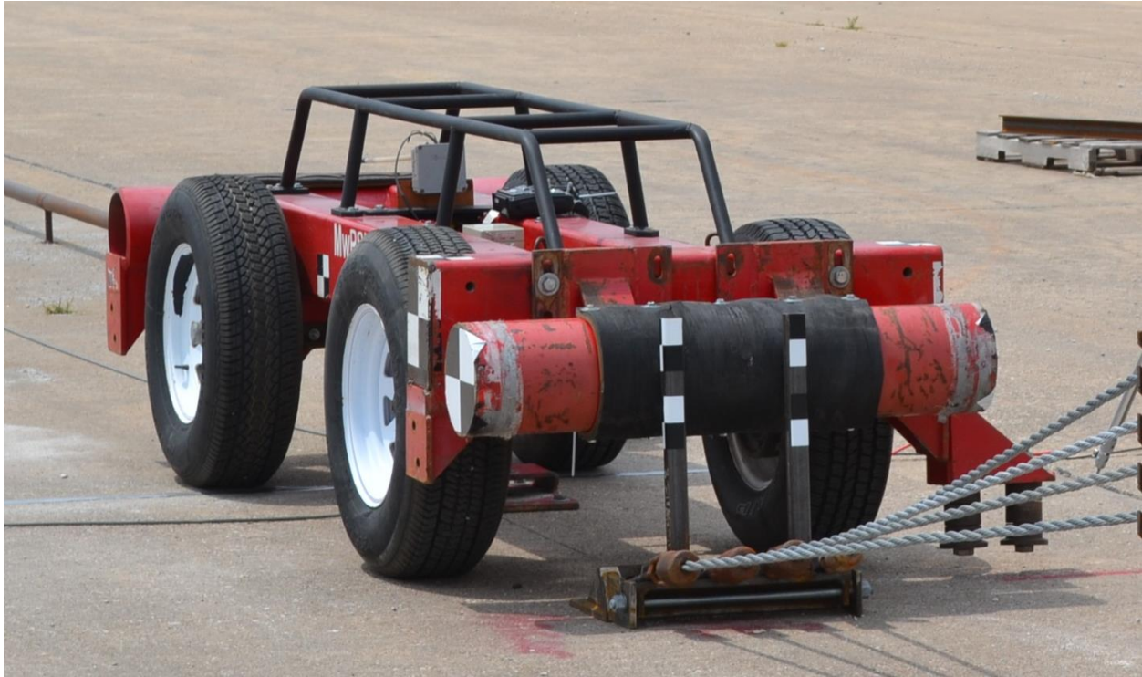
Figure 21. Rigid Frame Bogie on Guidance Track
