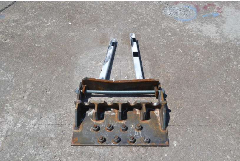
Figure 38. System Damage – Overall and Upstream Cable Anchor Bracket, Test No. HTCT-3
