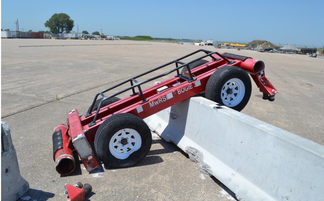
Figure 40. Bogie Damage, Test No. HTCT-3
