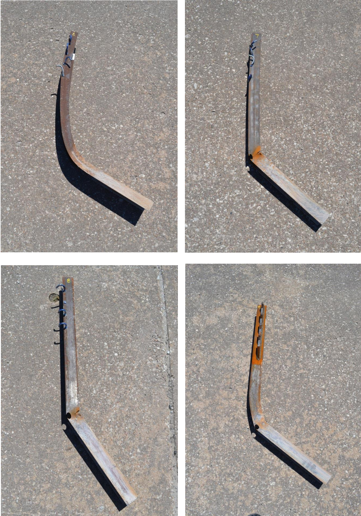
Figure 29. System Damage – Post nos. 6 through 9, Test No. HTCT-2
