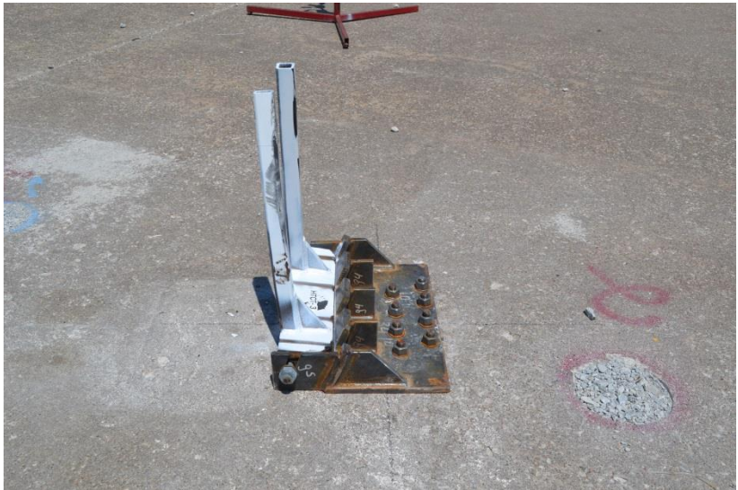
Figure 38. System Damage – Overall and Upstream Cable Anchor Bracket, Test No. HTCT-3
