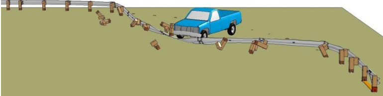
Impact at Post No. 9
