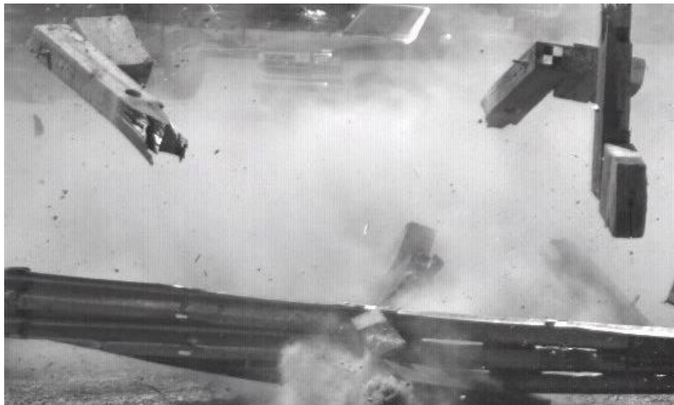
Figure 45. Fractured CRT Posts without Bolt Damage [14]
