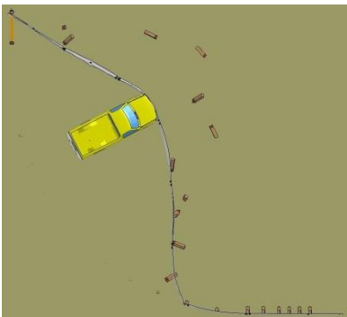
Figure 118. Images of Impacts with 31-in. (787-mm) Tall, 48-ft (15-m) Radius Systems at 50 mph (80 km/h)
