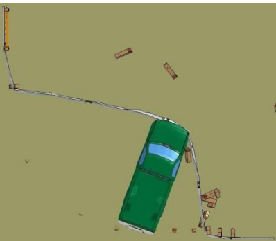
Figure 106. Images of Impacts with 31-in. (787-mm) Tall, 24-ft (7.3-m) Radius Systems at 45 mph (72 km/h)
