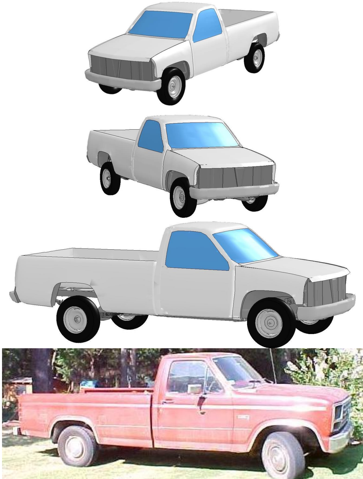
Figure 75. Ballasted 2500 Model and Example 1984 Ford Pickup Similar to Test Vehicle [32]
