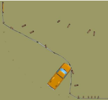
Figure 116. Images of Impacts with 31-in. (787-mm) Tall, 48-ft (15-m) Radius Systems at 45 mph (72 km/h)
