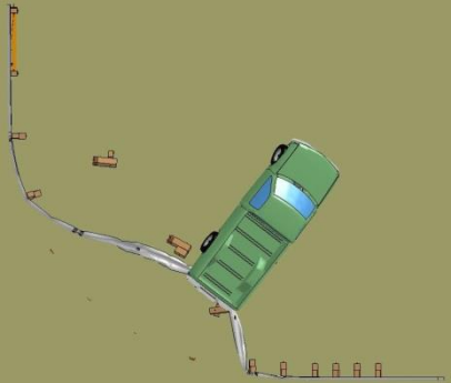
Figure 103. Images of Impacts with 27-in. (686-mm) Tall, 24-ft (7.3-m) Radius Systems with Blockouts Attached to Radius Posts
