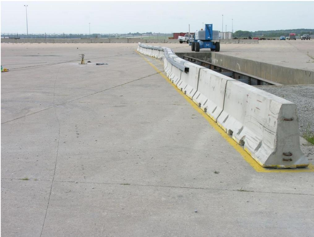
Figure 146. Vehicle Final Position and Trajectory Marks, Test No. RDTCB-2
