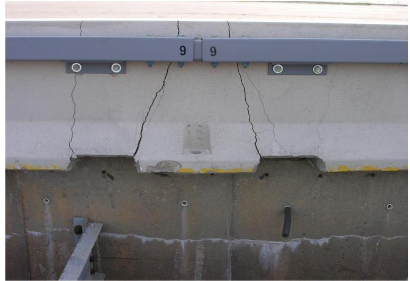
Figure 148. System Damage at Barrier Nos. 8 and 9, Test No. RDTCB-2
