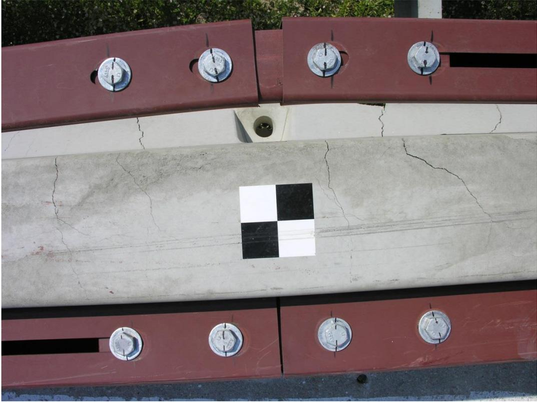
Figure 104. Steel Tube Deformation and Deflection, Test No. RDTCB-1
