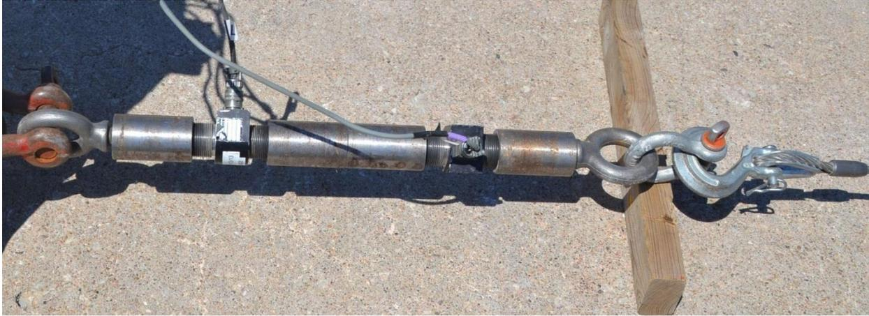
Figure 36. Load Cell Arrangement, Test Nos. TCBF-1 through TCBF-6
