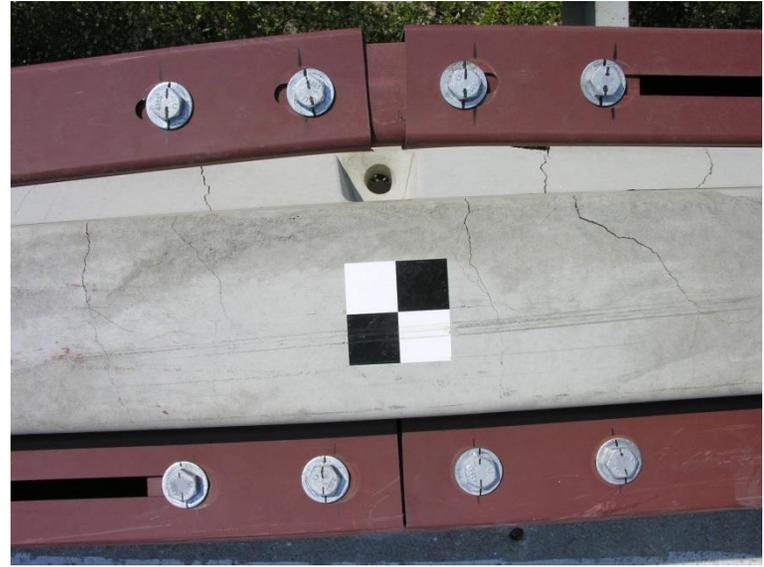
Figure 100. Rail Splice at Barrier Nos. 8 and 9, Test No. RDTCB-1
