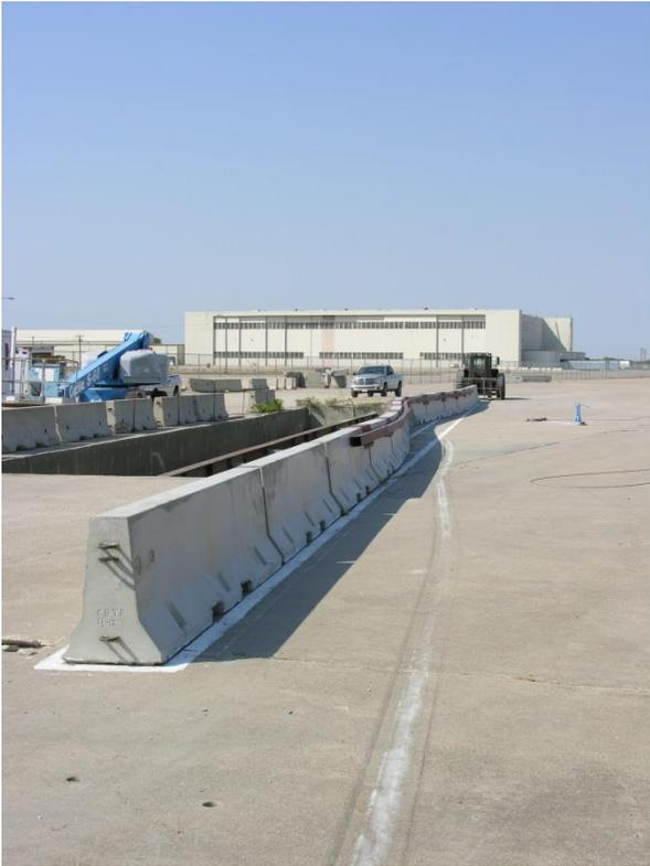
Figure 98. Overall System Damage, Test No. RDTCB-1
