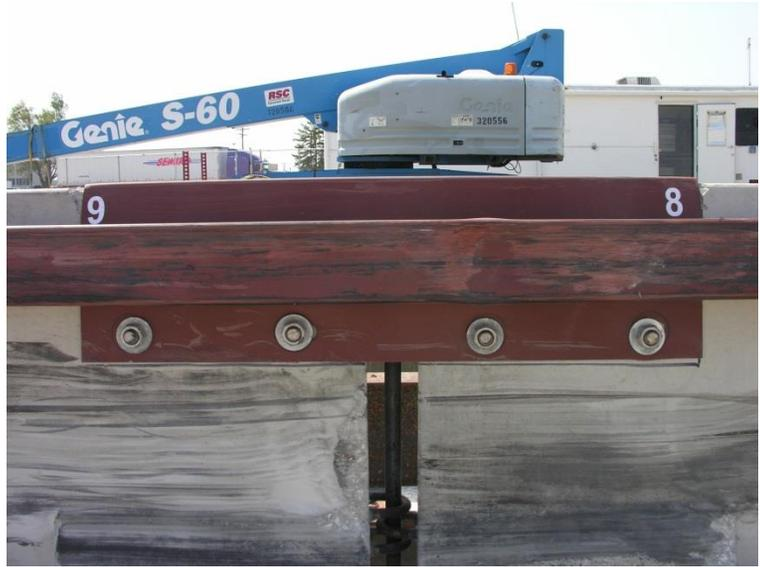
Figure 99. System Damage at Barrier Nos. 8 and 9, Test No. RDTCB-1
