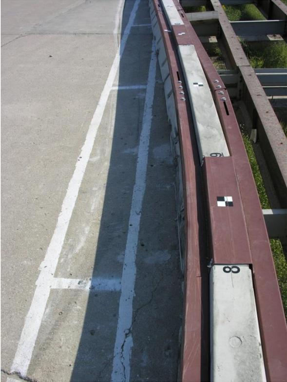
Figure 101. Permanent Barrier Deflection, Test No. RDTCB-1
