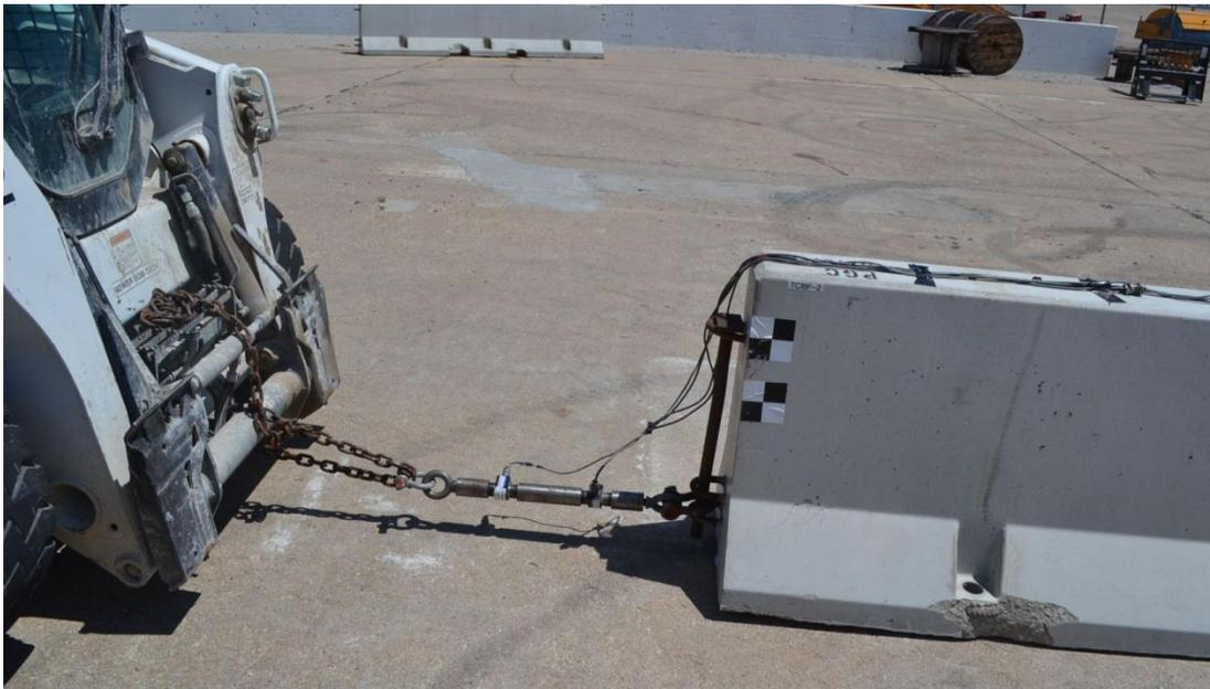
Figure 39. Pull Test Setup, Test No. TCBF-2
