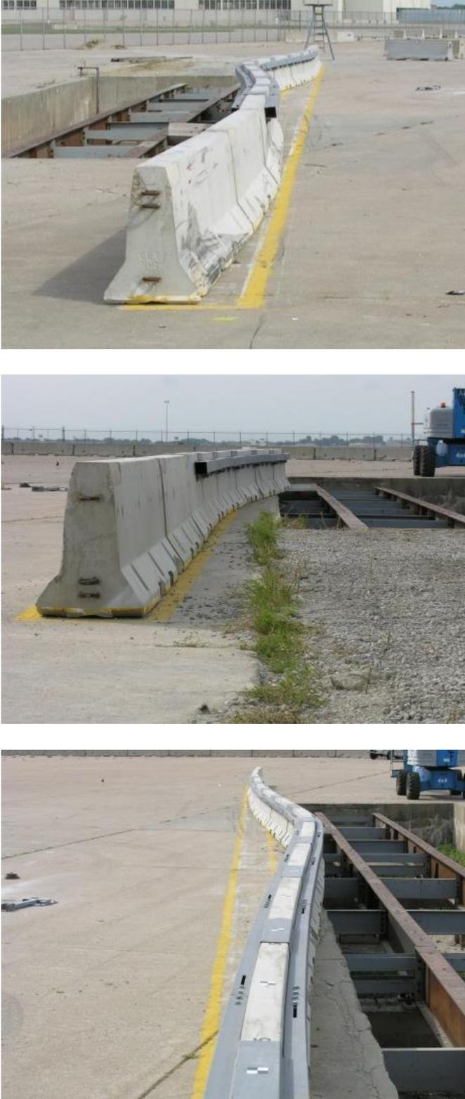
Figure 151. Permanent System Deflection, Test No. RDTCB-2
