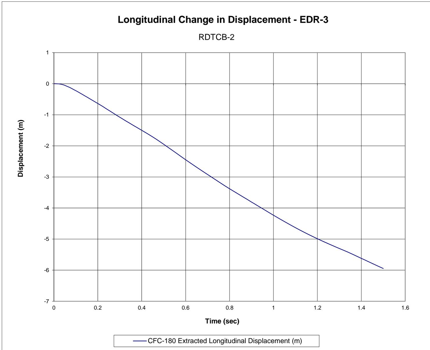
Figure G-19. Longitudinal Change in Displacement (EDR-3), Test No. RDTCB-2
