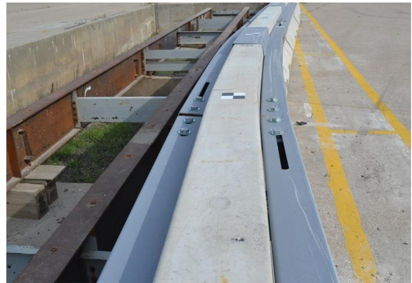
Figure 149. Rail Splices at Barrier Nos. 8 and 9, Test No. RDTCB-2
