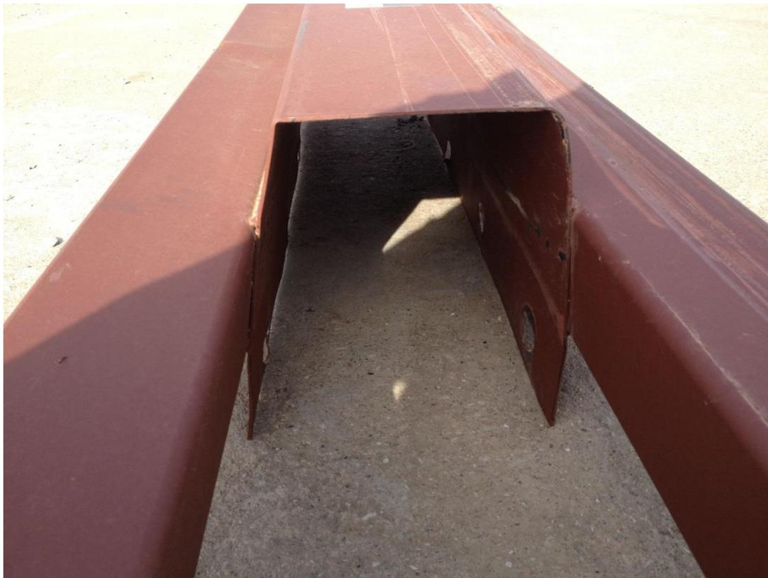
Figure 105. Steel Cap Deformation, Test No. RDTCB-1
