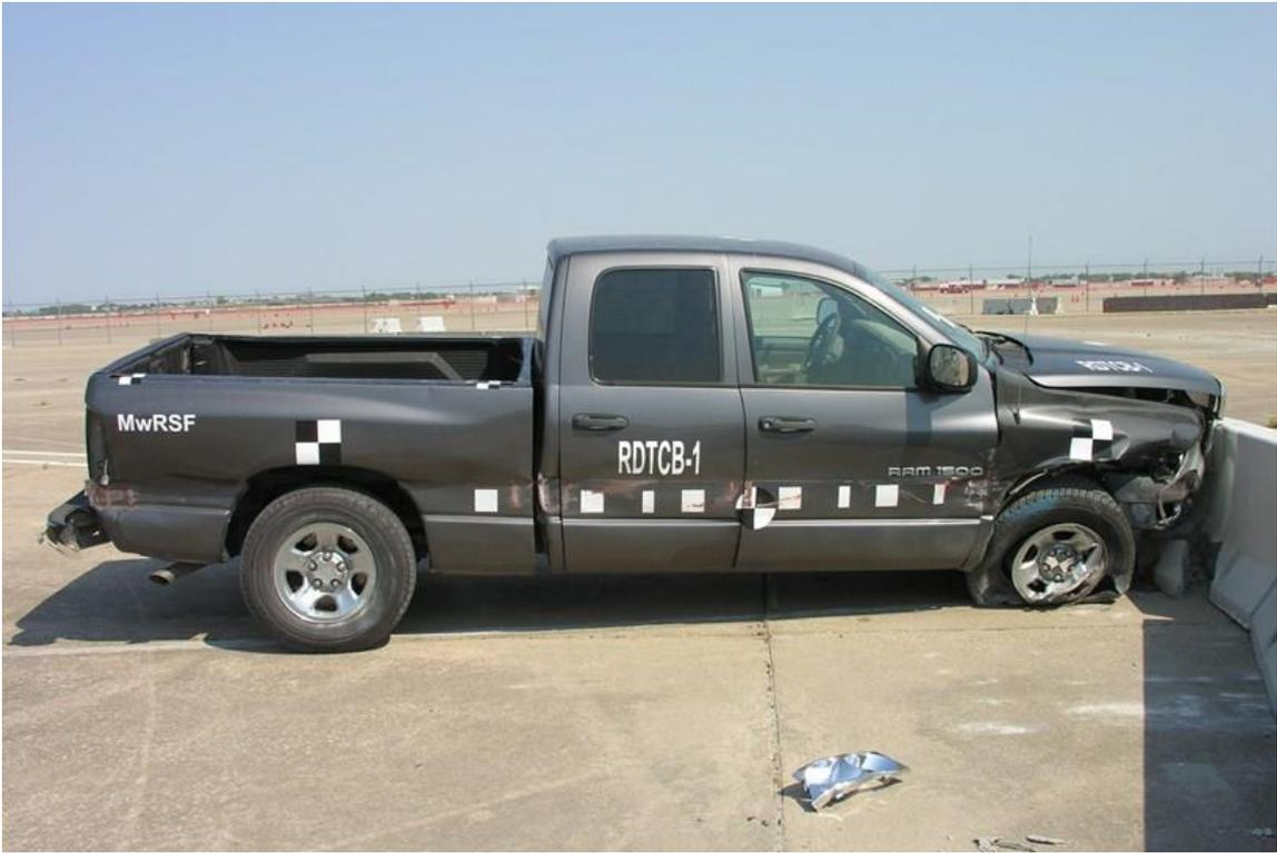
Figure 97. Vehicle Final Position and Trajectory Marks, Test No. RDTCB-1
