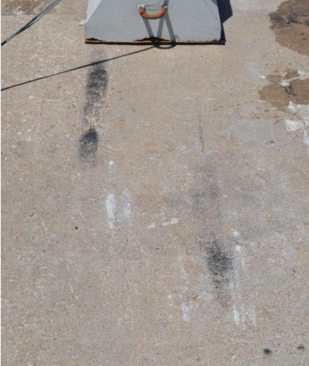
Figure 43. Rubber Wear Marks, Test No. TCBF-4
