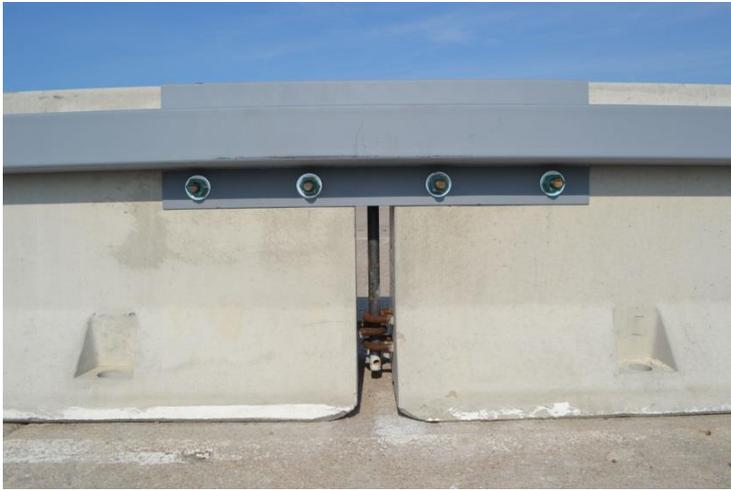
Figure 140. Barrier Segment Connection Designs, Test No. RDTCB-2
