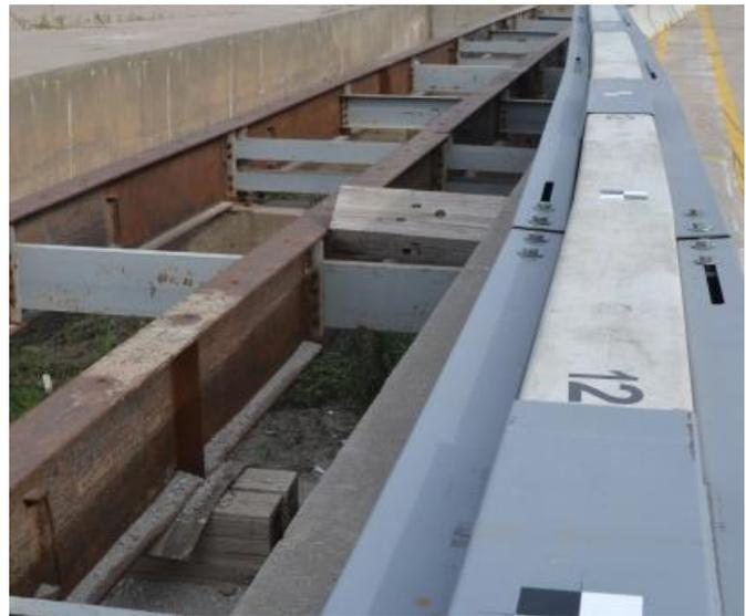
Figure 150. Barrier Segment Damage Due to Reverse Bending, Test No. RDTCB-2
