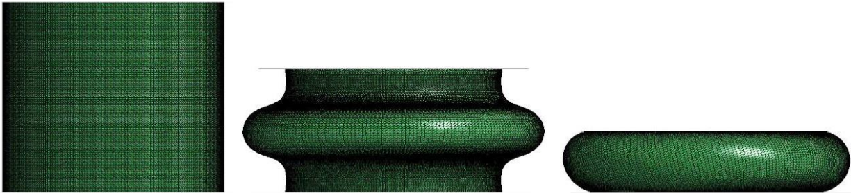
Figure 96. Blatz-Ko Cylinder Deformation, Test No. EPDM-3 Simulation
