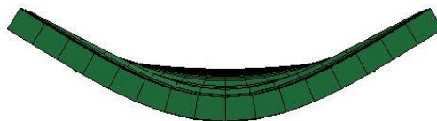
Figure 71. Type 4 and 5 Hourglass Control Solid Element Deformation, End View
