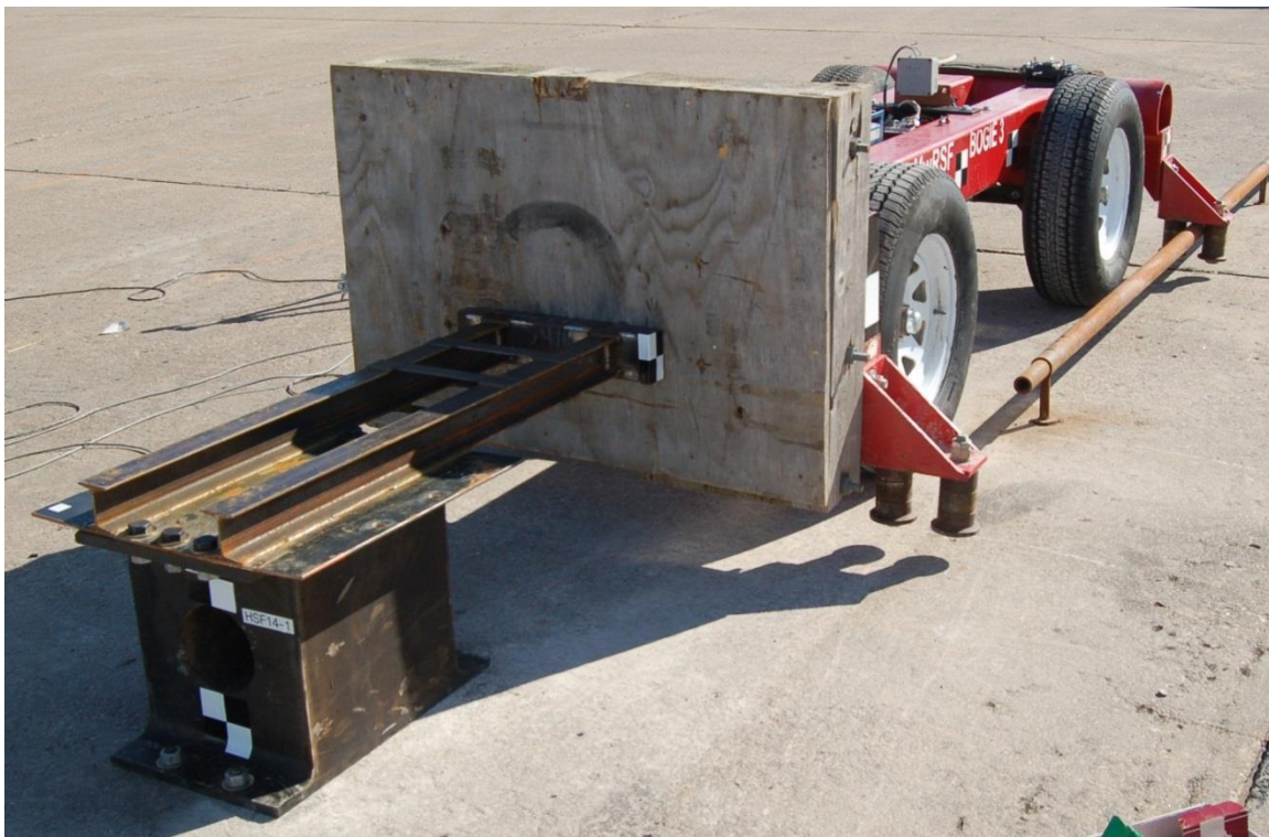
Figure 99. Shear Fender Bogie Test Setup
