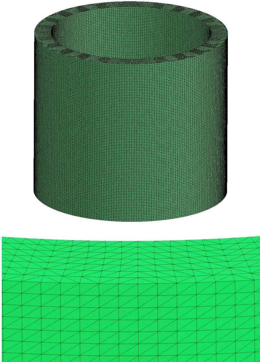
Figure 95. Tetrahedral Mesh, Test No. EPDM-3 Simulation
