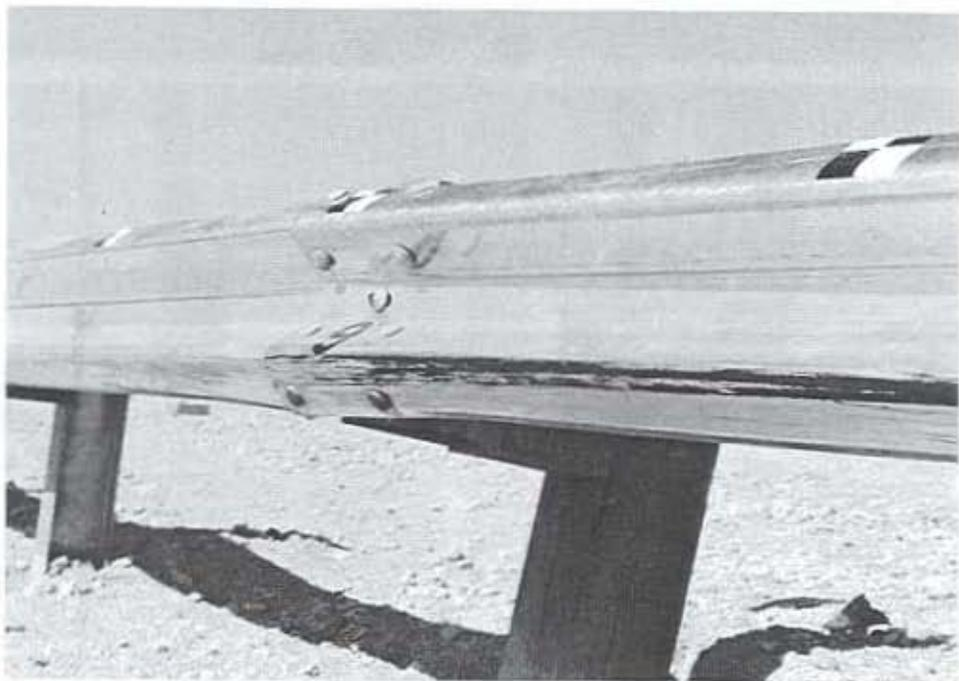
Figure 15. Long-Span Guardrail System Rail Damage, Test OLS-3 (Design No. 3)
