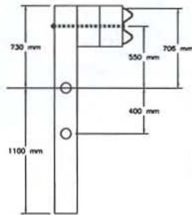
CRT wood posts, 1830 long w/ two 150x200x360 wood blockouts
