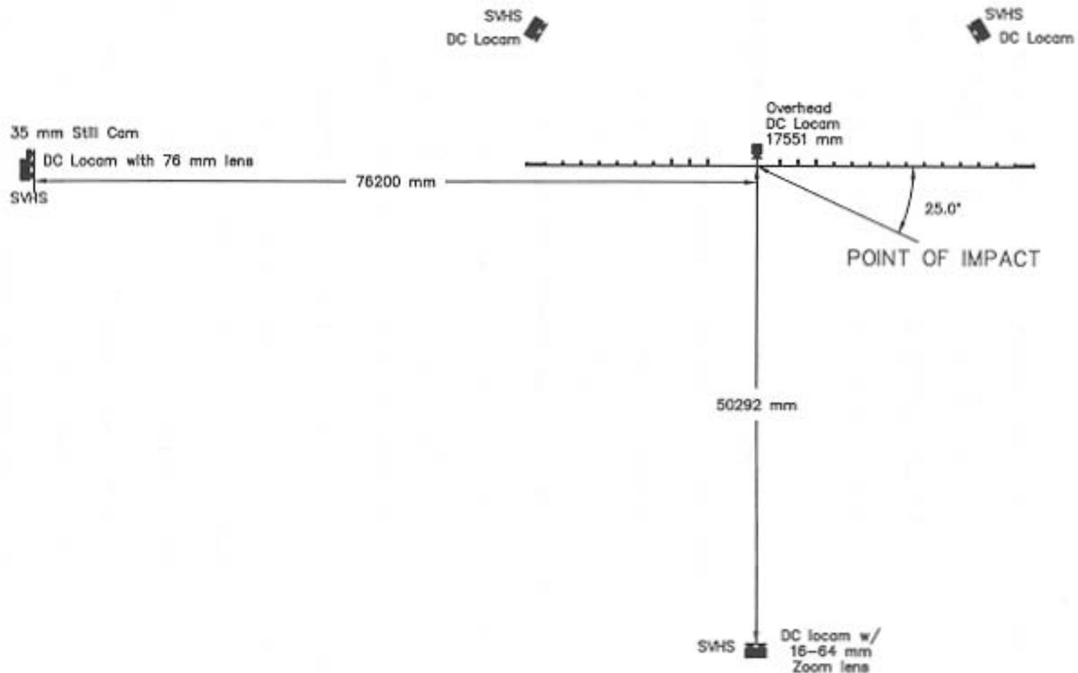
Figure 7. Location of High-Speed Cameras, Test OLS-3
