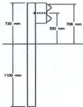
W152x13.4 steel posts, 1830 long w/ 150x200x360 routed wood blockouts
