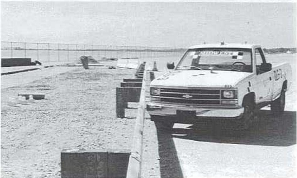
Figure 13. Impact Location, Test OLS-3 (Design No. 3)
