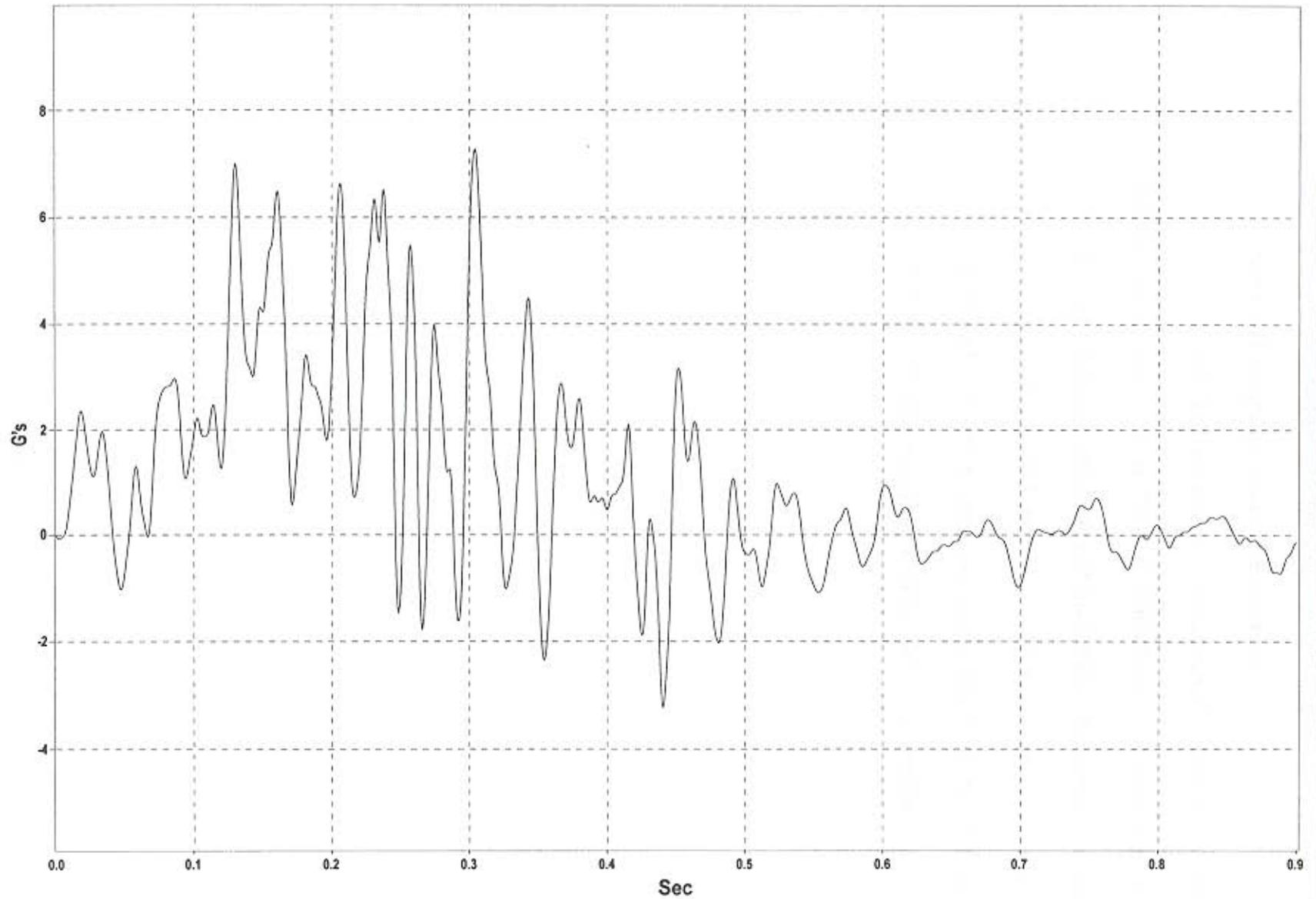
Figure A-1. Graph of Longitudinal Deceleration, Test OLS-3
